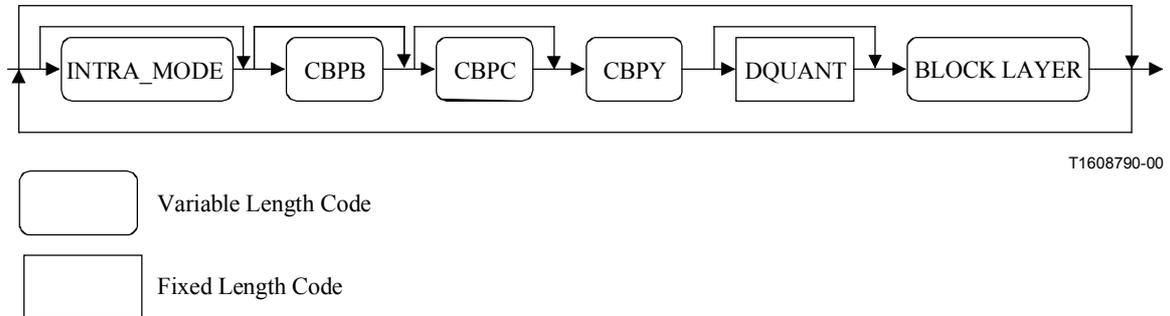
**Figure V.3/H.263 – Coefficient Data syntax**
