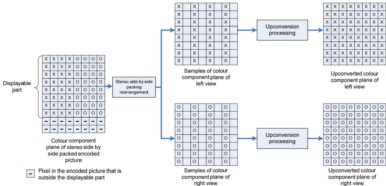
**Figure L.1 – Rearrangement and hypothetical upconversion of "stereo side by side" arrangement views to convert to the full resolution of the displayable part of the encoded picture**
