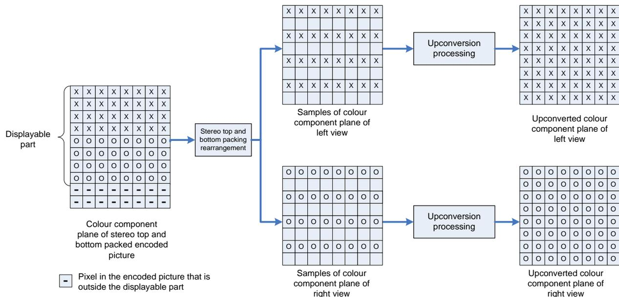
**Figure L.2 – Rearrangement and hypothetical upconversion of "stereo top and bottom" arrangement views to convert to the full resolution of the displayable part of the encoded picture**
