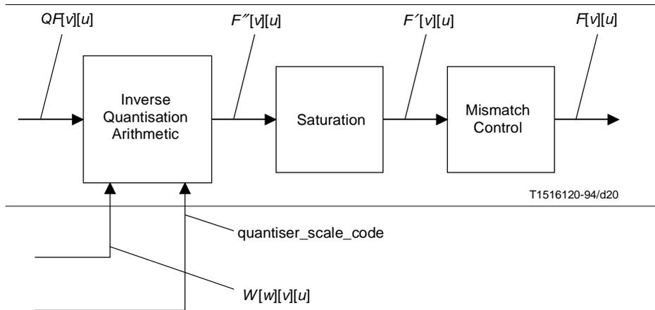
Figure 7-4 – Inverse quantisation process
