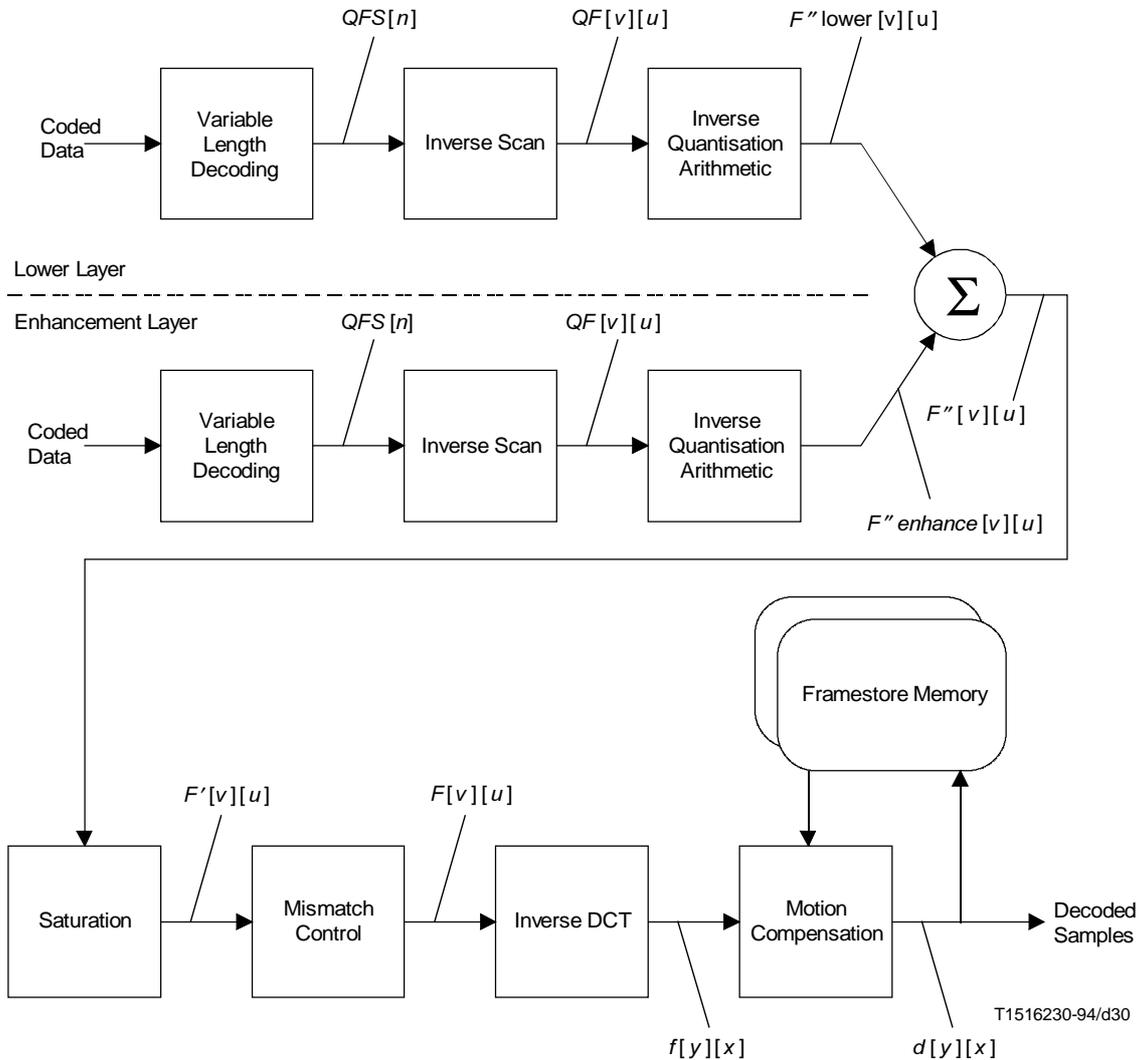
Figure 7-15 – Illustration of decoding process for SNR scalability
