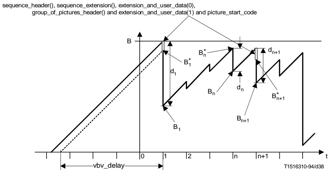
**Figure C.1 – VBV Buffer Occupancy – Constant bit-rate operation**
