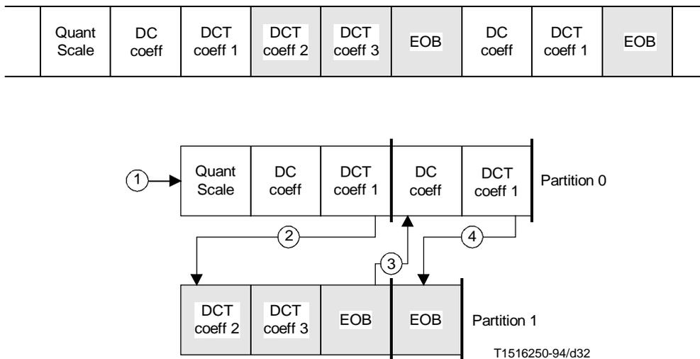
**Figure 7-17 – A segment from a bitstream with two partitions, with *priority\_breakpoint* set to 64 (one (run, level) pair). The two partitions are shown, with arrows indicating how the decoder needs to switch between partitions**
