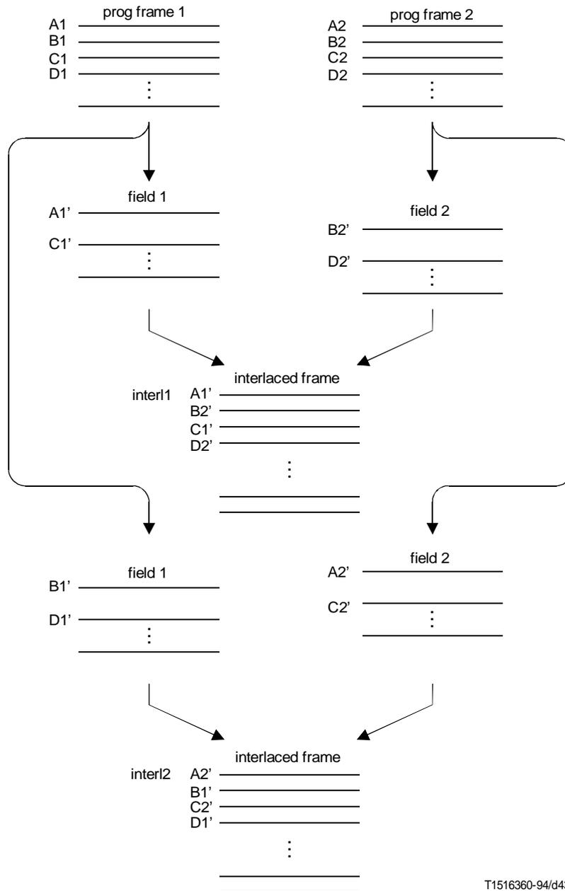
Figure D.3 – Progressive to two interlace conversion
