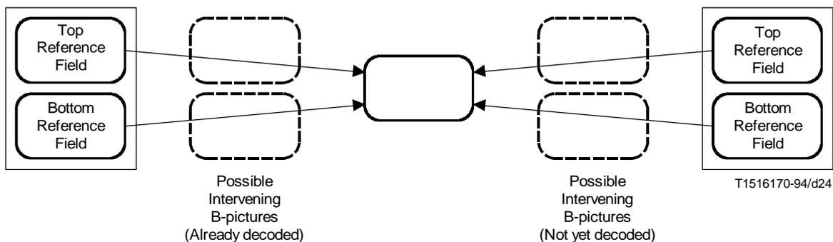
Figure 7-9 – Field-prediction of B-field pictures or B-frame pictures
