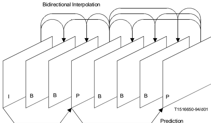
Figure Intro. 1 – Example of temporal picture structure
