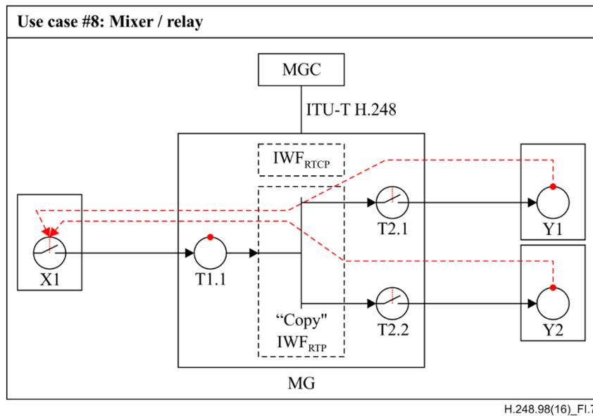
**Figure I.7 – Use-case #8 "Point-to-Dual point copying" (with three RTP participants) and a "P/R-signalling passive MG"**
