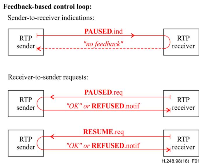
NOTE – The "P/R-signalling" path is highlighted in red.
