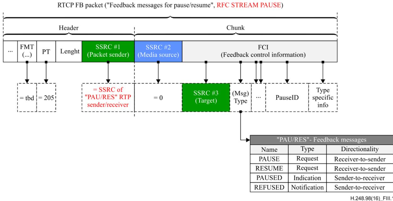
**Figure III.1 – RTCP FB packets for pause/resume-signalling – SSRC related fields**
