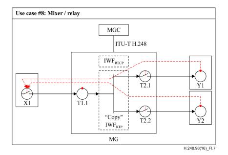
Figure I.7 – Use-case #8 "Point-to-Dual point copying" (with three RTP participants) and a "P/R-signalling passive MG"
