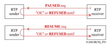
NOTE - The "P/R-signalling" path is highlighted in red.
