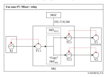
Figure I.6 – Use-case #7 "Point-to-Dual point copying" (with three RTP participants) and a "P/R-signalling active MG"
