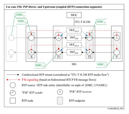
Figure III.2 – Example use case #3b (from Appendix I) – Extended for bidirectional P/R-signalling and indication of SSRCs
