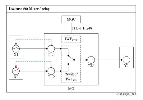
Figure I.5 – Use-case #6 "Dual point-to-Point switching" (with three RTP participants)
