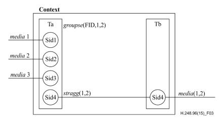
**Figure 3 – Signals on an aggregation stream with FID semantic**
