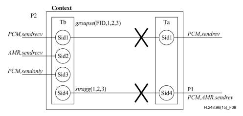
Figure 9 – Example of invalid direct stream and aggregation stream connection between two Terminations
