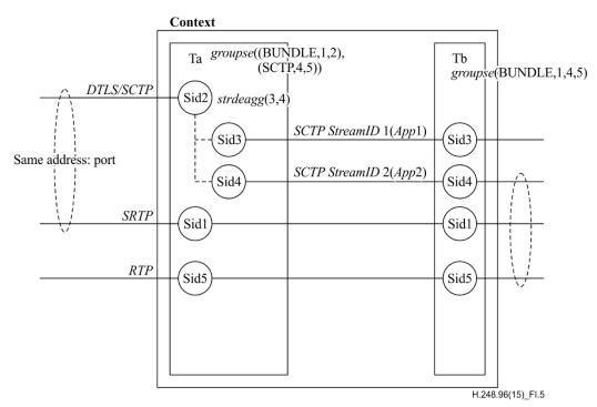
**Figure I.5 – Deaggregation component to subsequent semantic**
