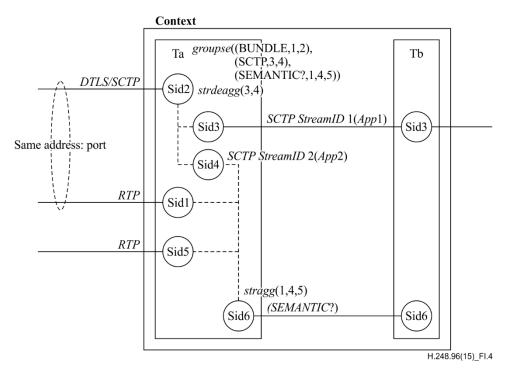
**Figure I.4 – Deaggregation component to aggregation cascade**
