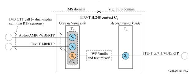
Figure II.2 – Use case #1.1: alternate speech-text telephony in IP-to-IP gateways – Context stream grouping model
