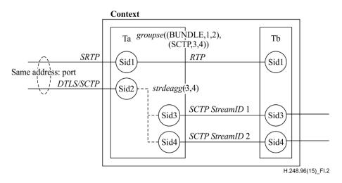
Figure I.2 – Multiple de-multiplexes one deaggregation
