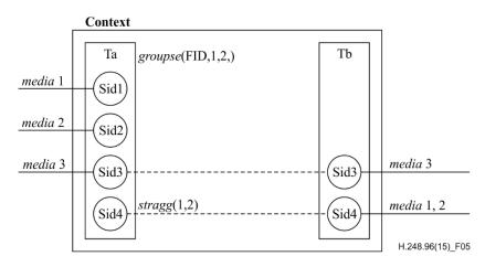
Figure 5 – Events on an aggregation stream with FID semantic
