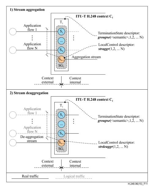
Figure 11 – Half context model – Principle use cases of 1) Stream aggregation and 2) Stream deaggregation
