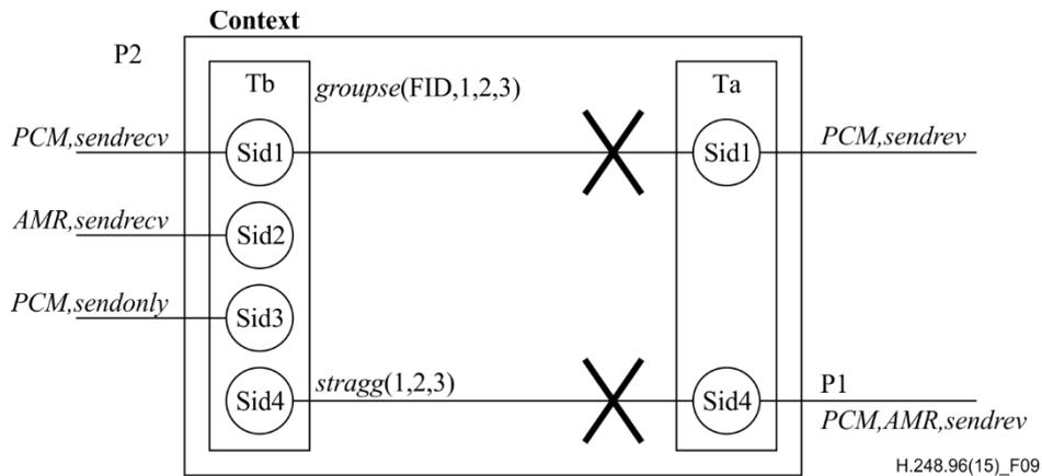
**Figure 9 – Example of invalid direct stream and aggregation stream connection between two Terminations**
