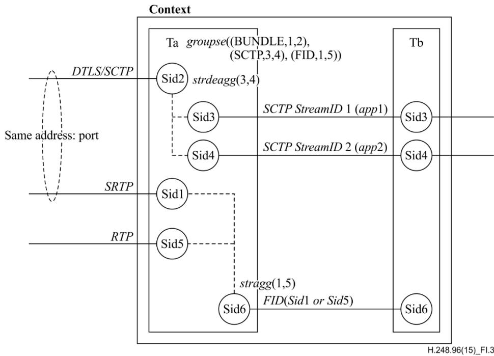
**Figure I.3 – Deaggregation to aggregation no cascade**
