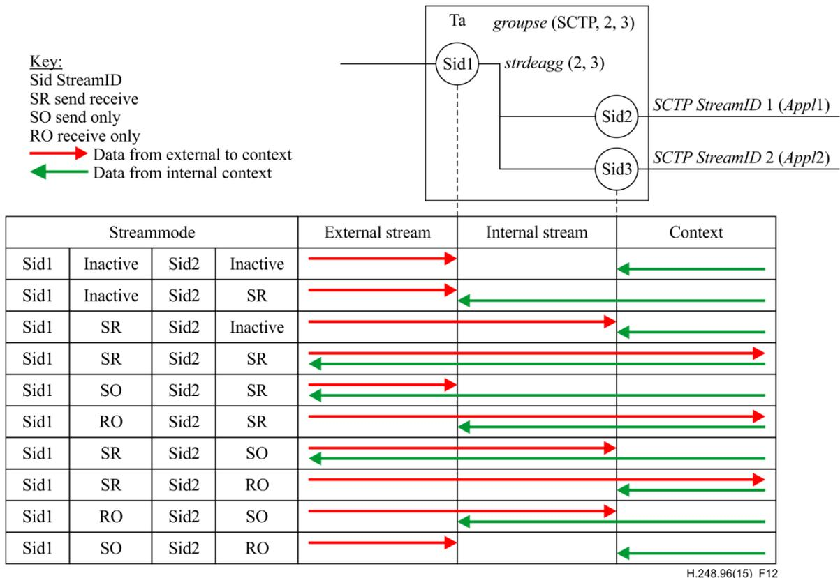
**Figure 12 – Deaggregation stream property interaction: StreamMode**
