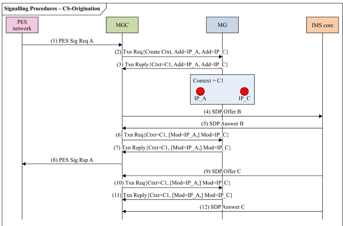
**Figure II.3 – Overall message sequence diagram for a call in PES-to-IMS direction**
