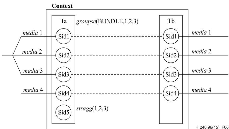
**Figure 6 – Statistics on an aggregation stream with BUNDLE semantic**
