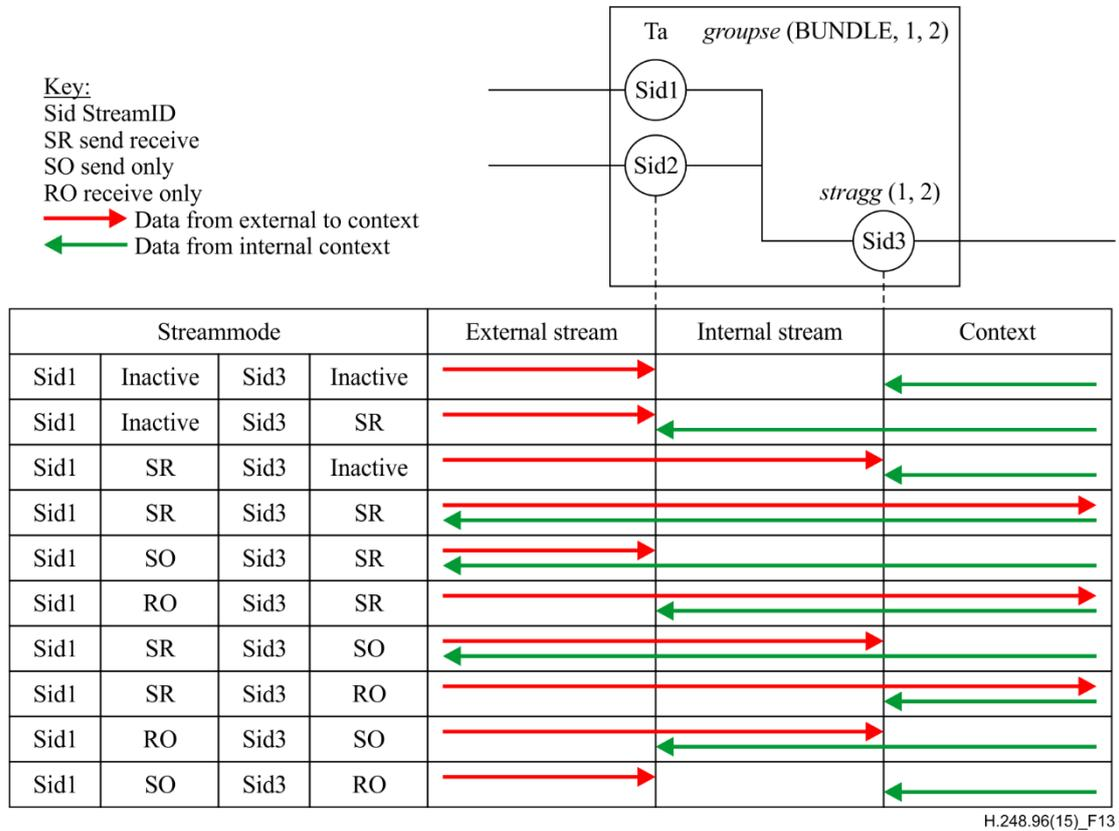
**Figure 13 – Aggregation stream property interaction: StreamMode**
