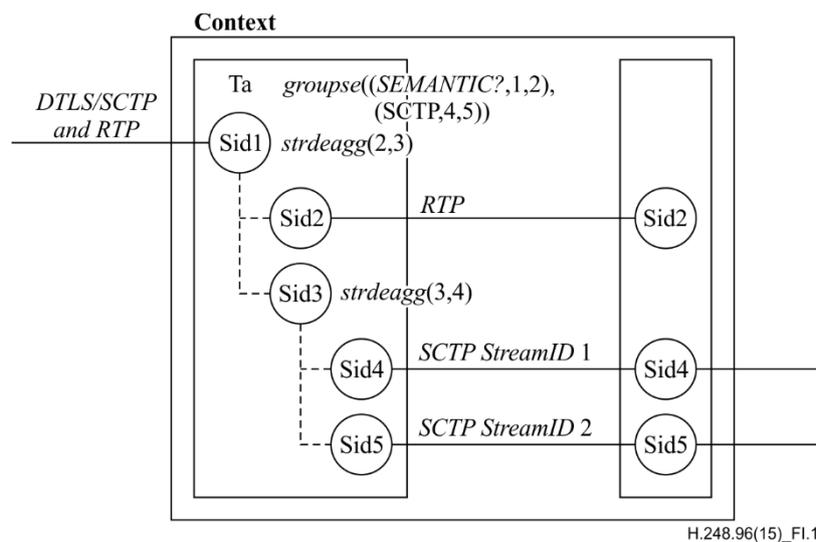
Figure I.1 – Deaggregation component to deaggregation stream cascade
