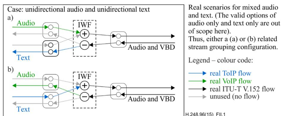
**Figure II.1 – Use case #1.1: alternate speech-text telephony in IP-to-IP gateways – Traffic flow models**
