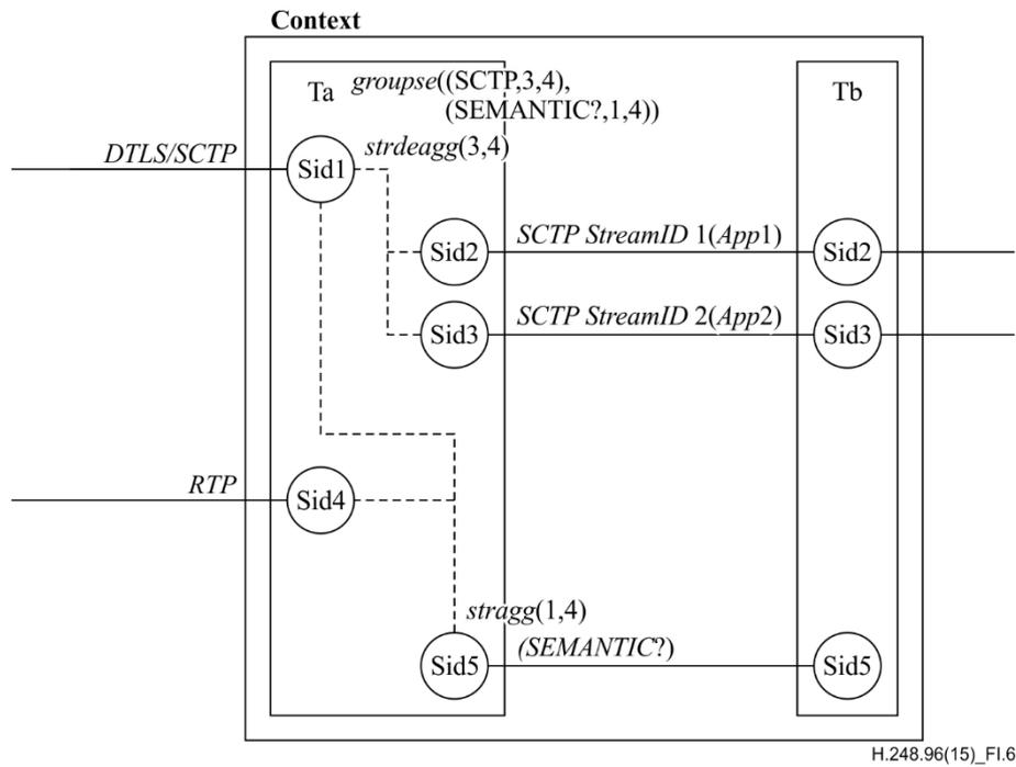
**Figure I.6 – Deaggregation stream to aggregation cascade**
