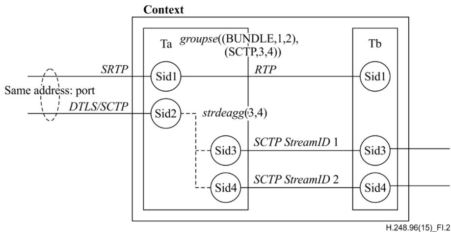
**Figure I.2 – Multiple de-multiplexes one deaggregation**
