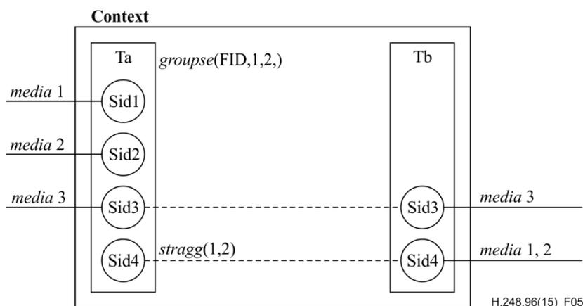
**Figure 5 – Events on an aggregation stream with FID semantic**
