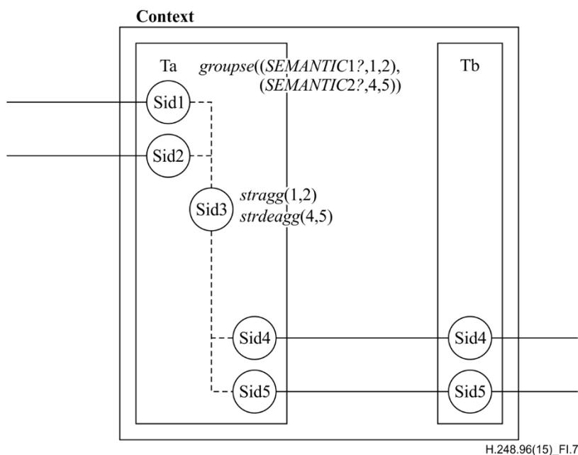
**Figure I.7 – Aggregation to deaggregation cascade**
