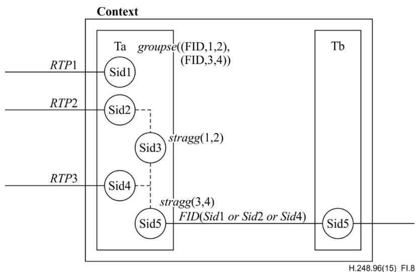
**Figure I.8 – Aggregation stream as aggregation component**
