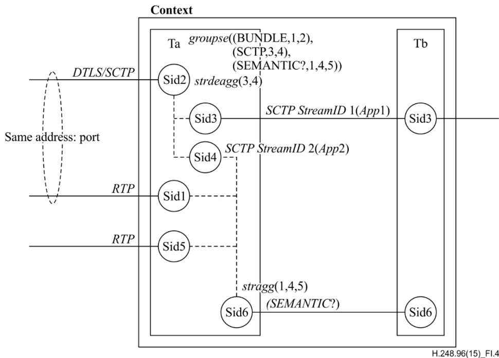
**Figure I.4 – Deaggregation component to aggregation cascade**
