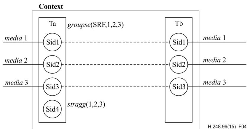
**Figure 4 – Events on an aggregation stream with SRF semantic**
