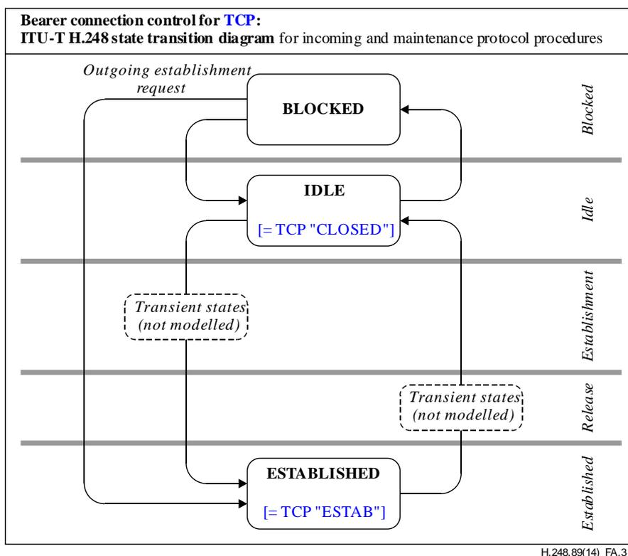
**Figure A.3 – Extended state model for ITU-T H.248-based TCP basic connection control**
