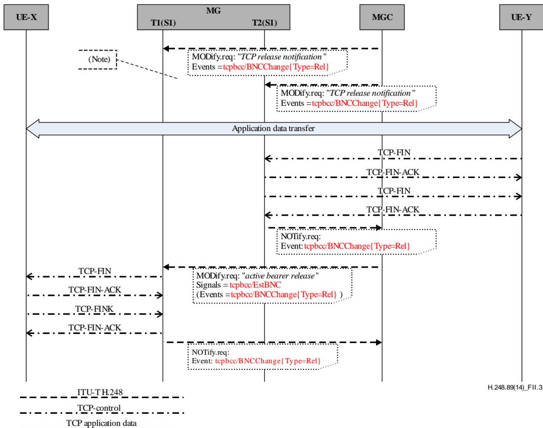
NOTE – MGC does not know whether X or Y initiates a TCP CLOSE procedures. Thus, release notification enabled at both SFPs.
