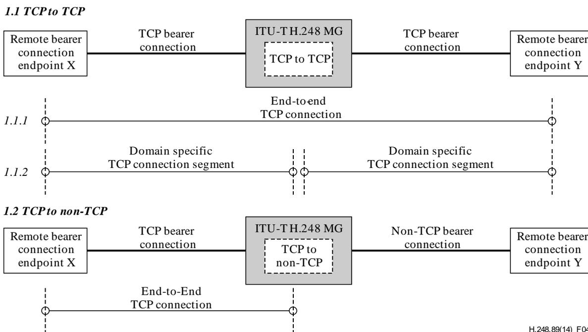
**Figure 4 – Bearer connection network use cases with TCP stream endpoints**
