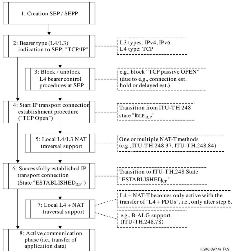
**Figure 9 – Principal ITU-T H.248 control steps for establishing a native TCP bearer**
