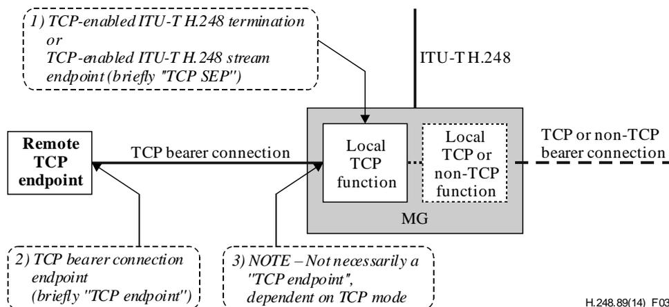
**Figure 3 – Conventions for TCP endpoint types**
