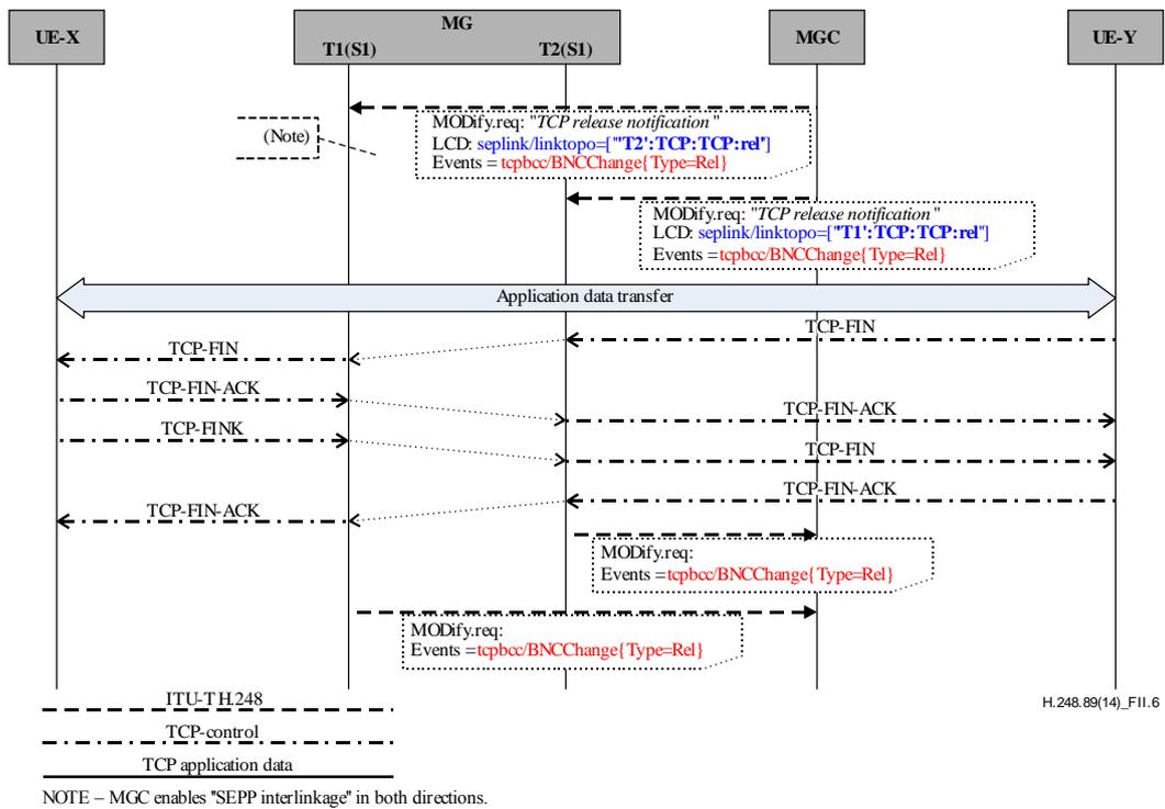
**Figure II.6 – Traffic flow example for an extended TCP bearer connection release**
