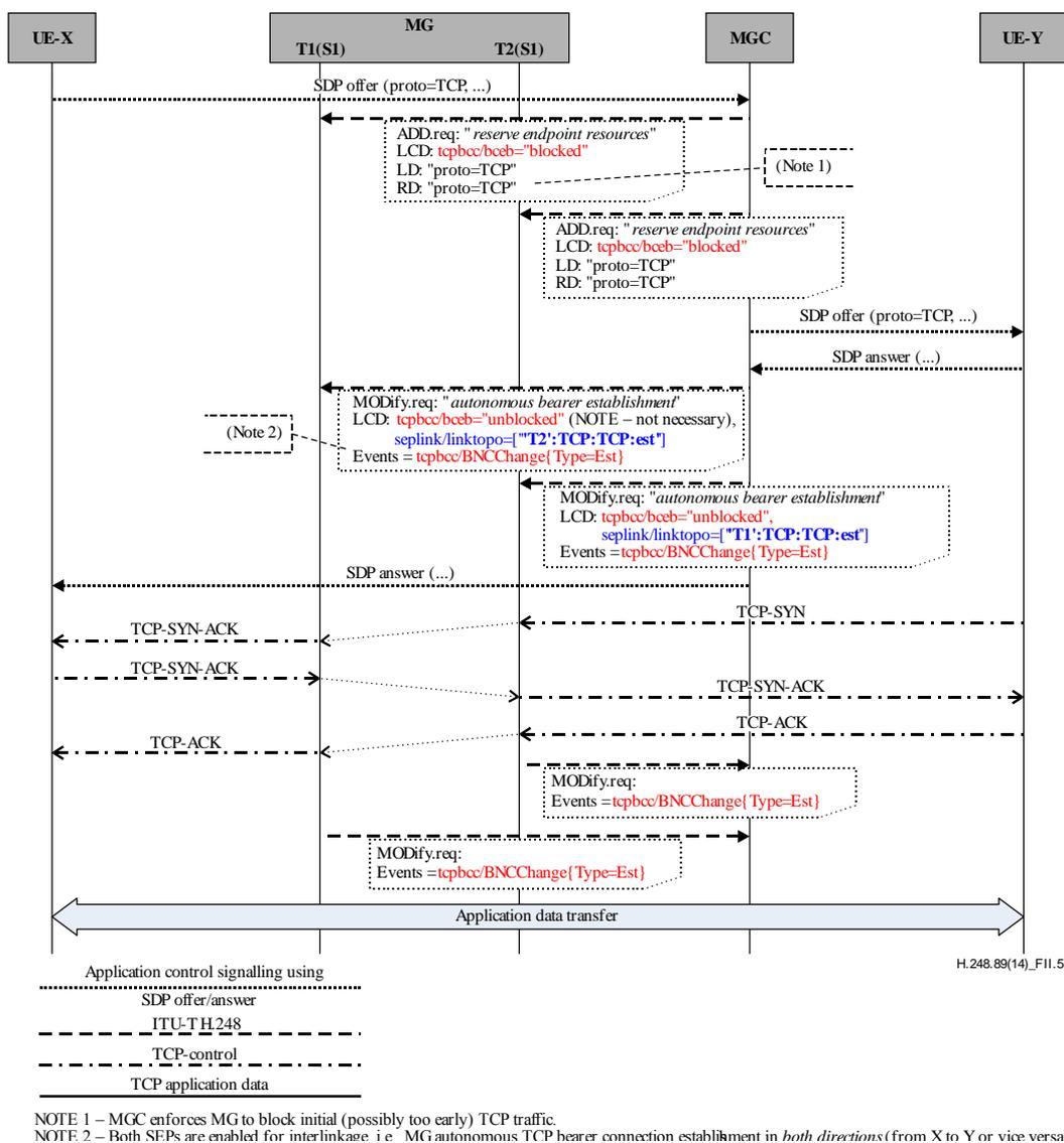
Figure II.5 – Traffic flow example for an extended TCP bearer connection establishment
