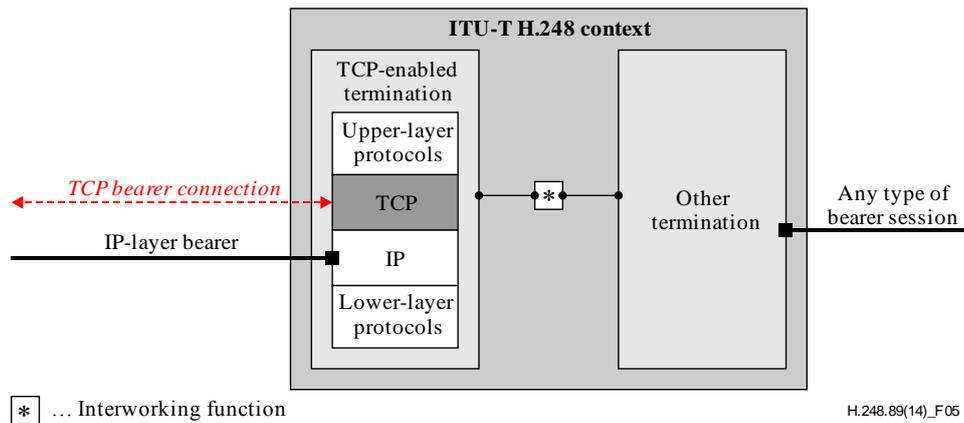
**Figure 5 – Two-termination context with a single TCP termination only**
