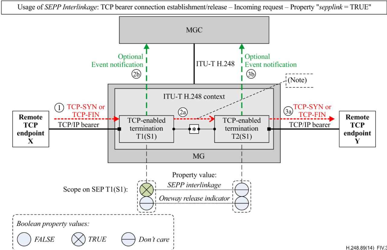
**Figure IV.3 – Property "seplink/linktopo" enabled for establishment and release at SEP T1(S1)**
