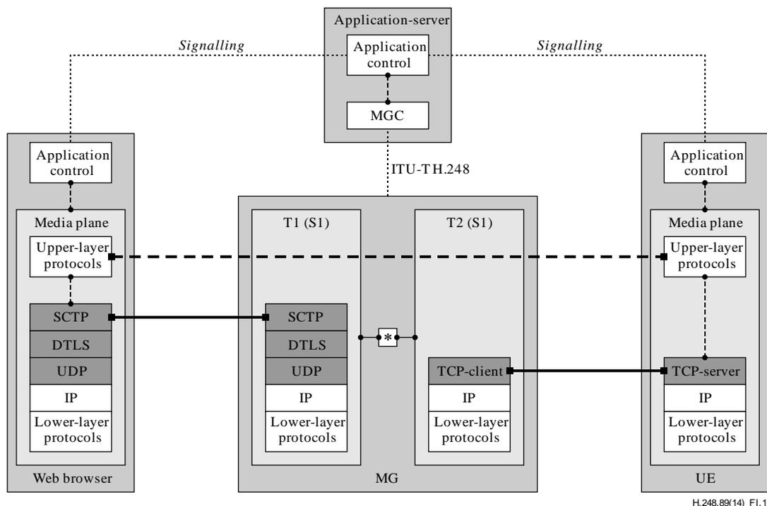
Figure I.1 – Use-case #1: WebRTC to IMS interworking function
