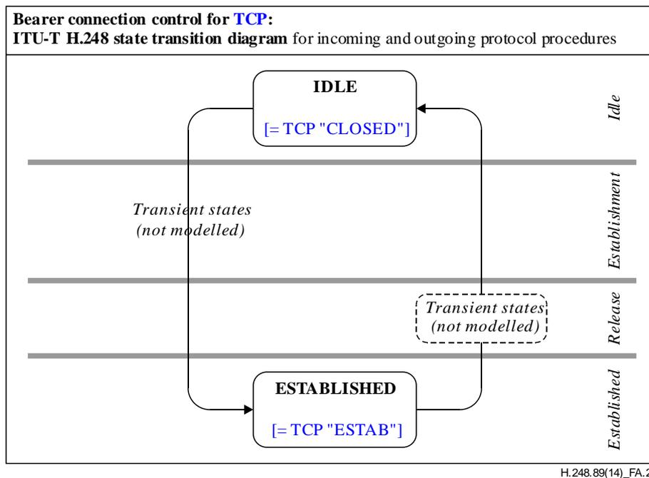
**Figure A.2 – Simplified state model for ITU-T H.248-based TCP basic connection control**
