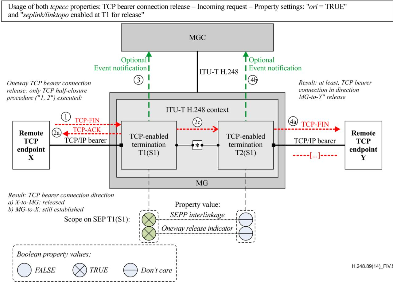
**Figure IV.8 – Property settings: "ori = TRUE" and "seplink/linktopo" enabled for release**
