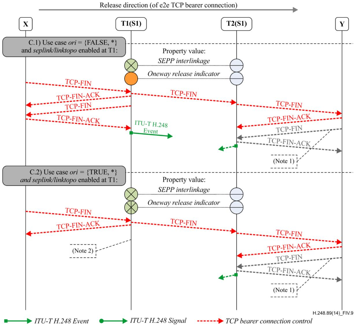
**Figure IV.9 – Signalling example for TCP bearer connection release and example value combinations for both properties**
