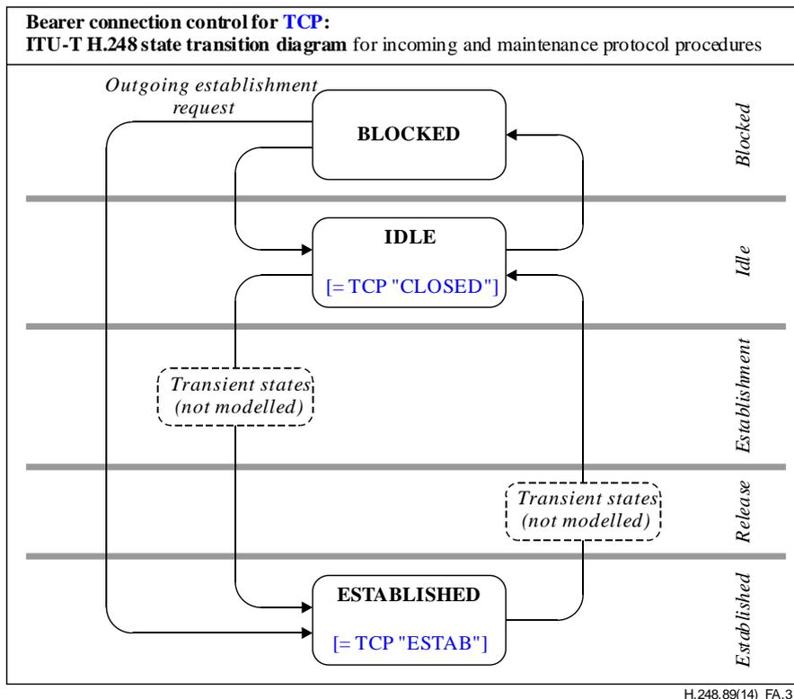
**Figure A.3 – Extended state model for ITU-T H.248-based TCP basic connection control**
