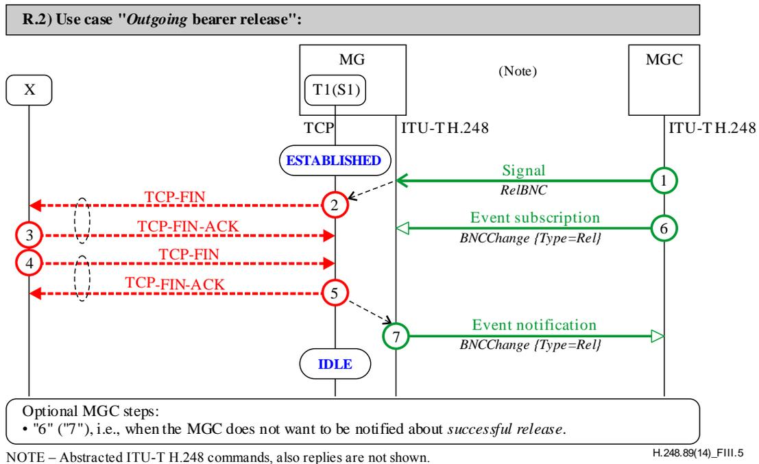
**Figure III.5 – Successful release – Originating side**
