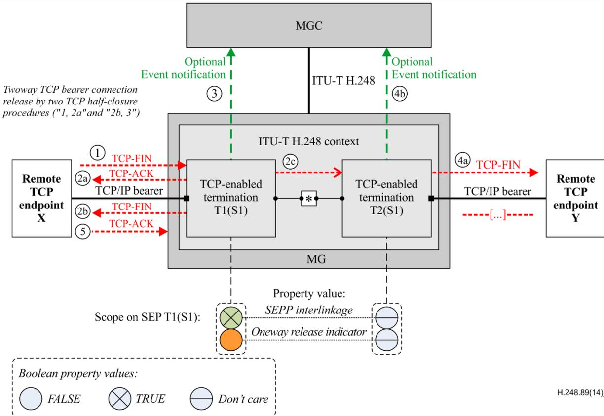
**Figure IV.7 – Property settings: "*ori* = FALSE" and "*seplink/linktopo*" enabled for release**
