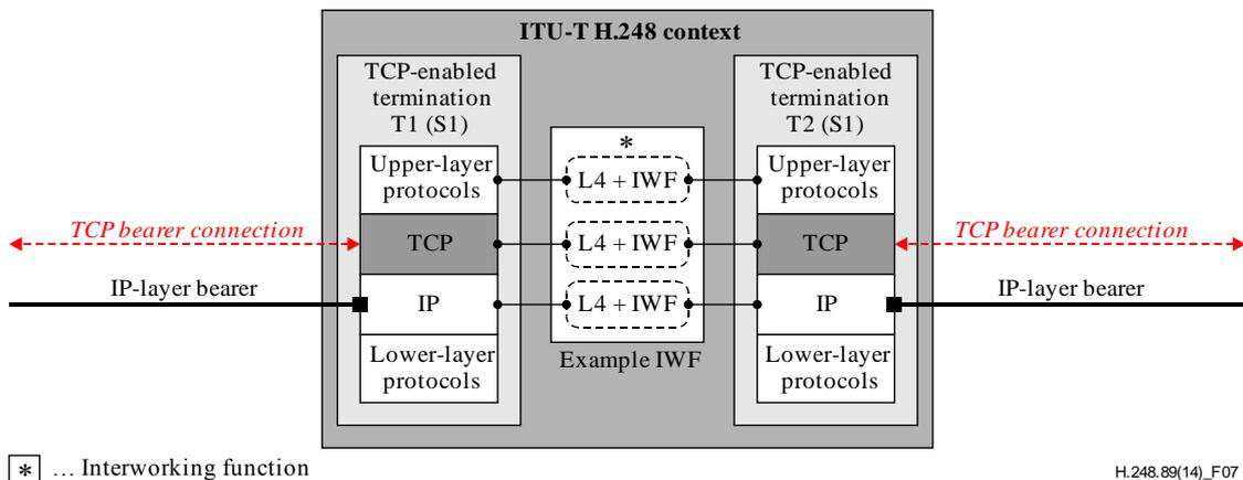
**Figure 7 – Two-termination context with context-internal interworking function**
