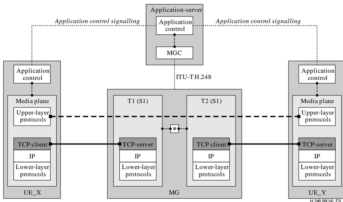
**Figure II.1 – Configuration "application agnostic TCP-proxy"**
