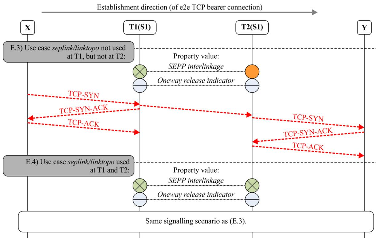
NOTE – It should be noted that the first received TCP-SYN at T1(S1) is not MG-internally forwarded as a "TCP/IP packet", rather an internal, abstracted stimuli is generated which triggers the outgoing TCP-SYN at T2(S1).
