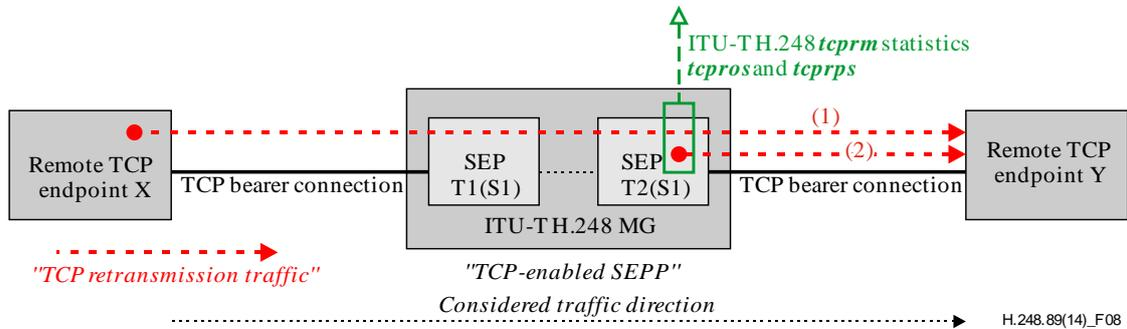
**Figure 8 – "TCP retransmission traffic" in (TCP, TCP) connection models**
