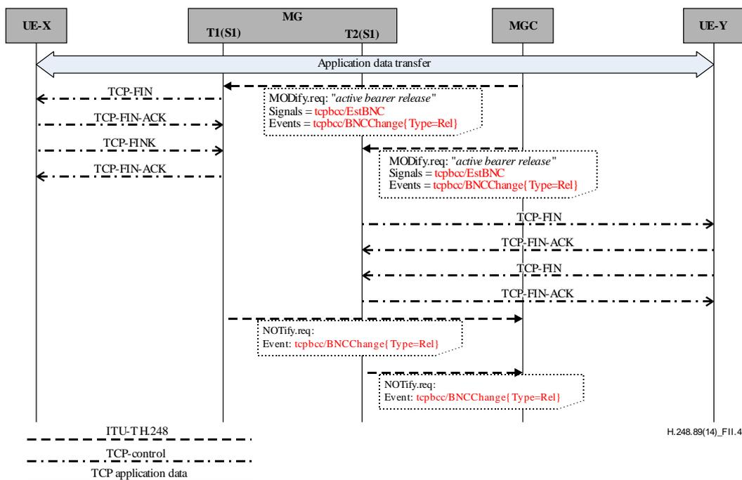
**Figure II.4 – Traffic flow example for outgoing TCP bearer connection release procedures towards both remote TCP endpoints X and Y**
