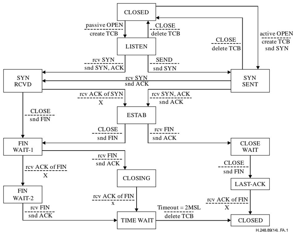
Figure A.1 – TCP connection state diagram [IETF RFC 793]
