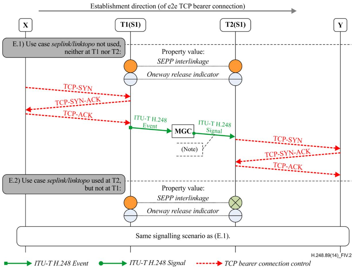
NOTE – The Signal for SEP<sub>T2(S1)</sub> may be independent of Event from SEP<sub>T1(S1)</sub>
