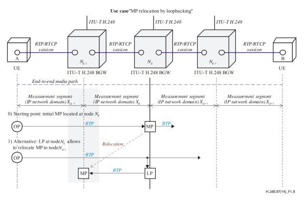
Figure I.8 – Use case 8: MP relocation by loopbacking
