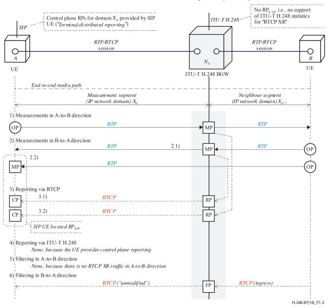
Use case"IP-IP ITU-T H.248 MG and remote SIP UE - Single control plane RP, by UE"
