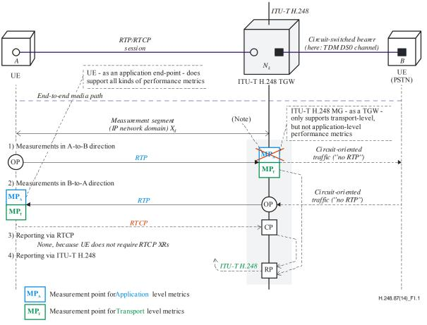
Use case "ITU-T H.248 MG with connection model (RTP, non-RTP), e.g., trunking gateway"
