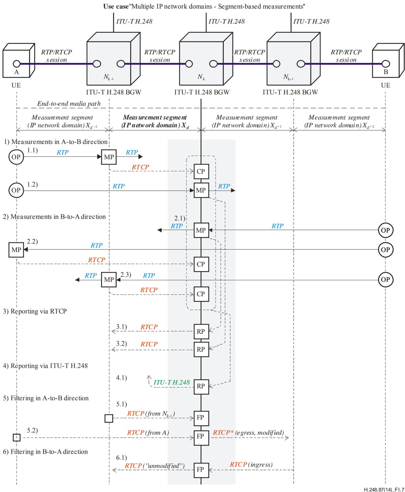
**Figure I.7 – Use case 7: Multiple IP network domains – Segment-based measurements**
