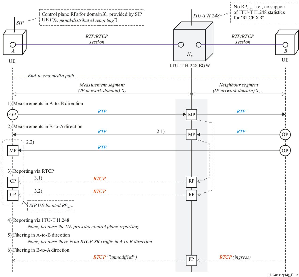
Figure I.3 – Use case 3: IP-IP ITU-H.248 MG and remote SIP UE – Single control plane RP by UE
