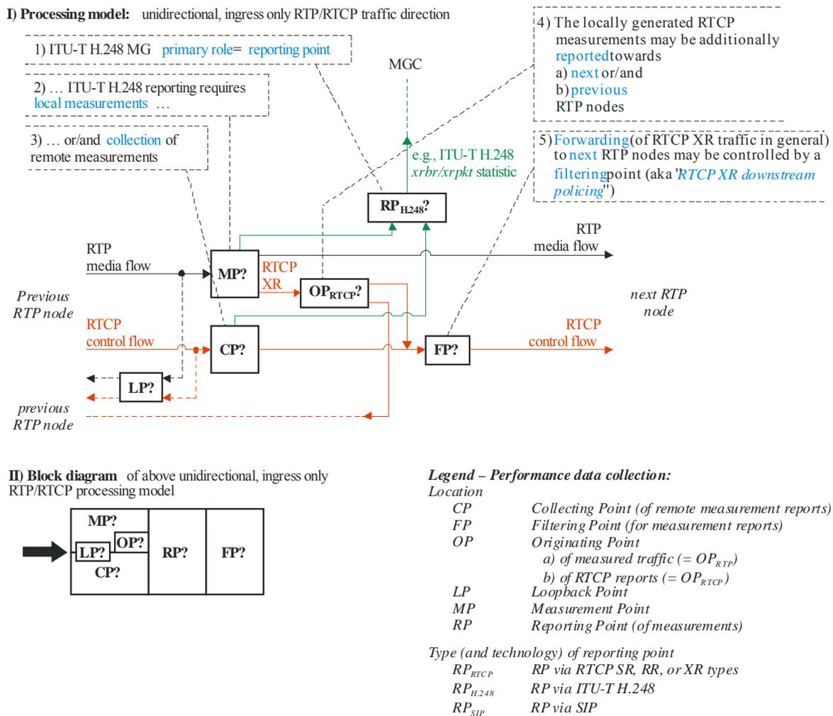
**Figure 3 – RTCP-based performance measurements – ITU-T H.248 IP-to-IP border gateway/router – Unidirectional, ingress only RTP/RTCP processing model**
