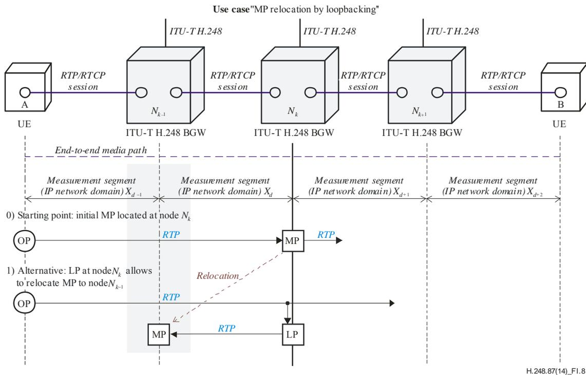
**Figure I.8 – Use case 8: MP relocation by loopbacking**
