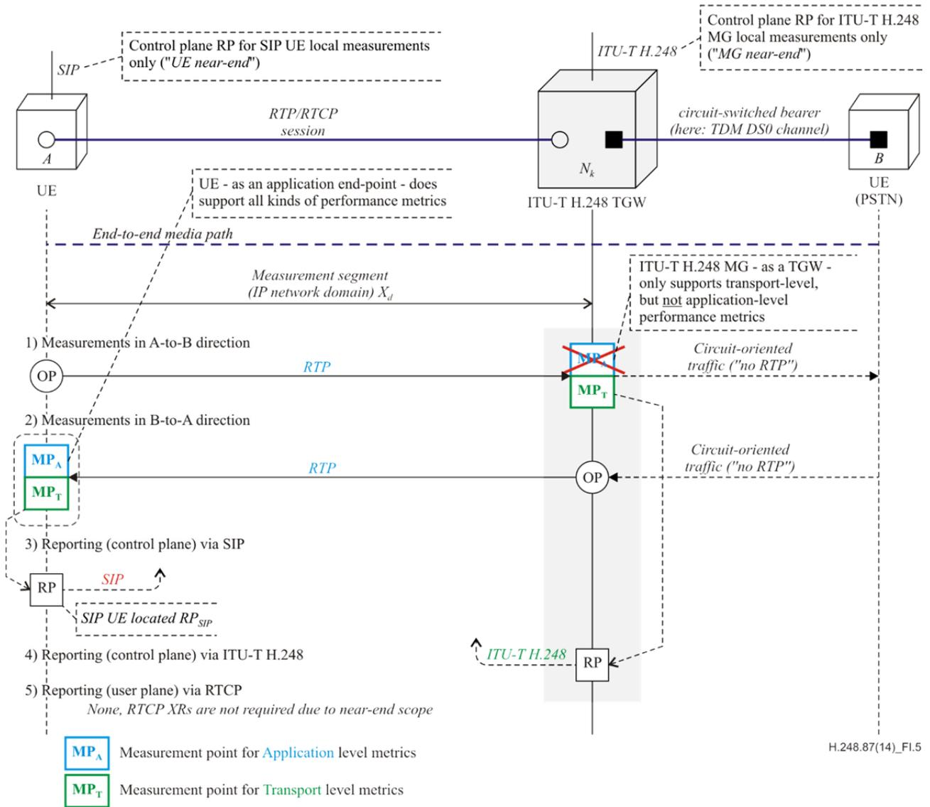
**Figure I.5 – Use case 5: Distributed control plane reporting covering near-end measurements only (at the example of a trunking gateway)**
