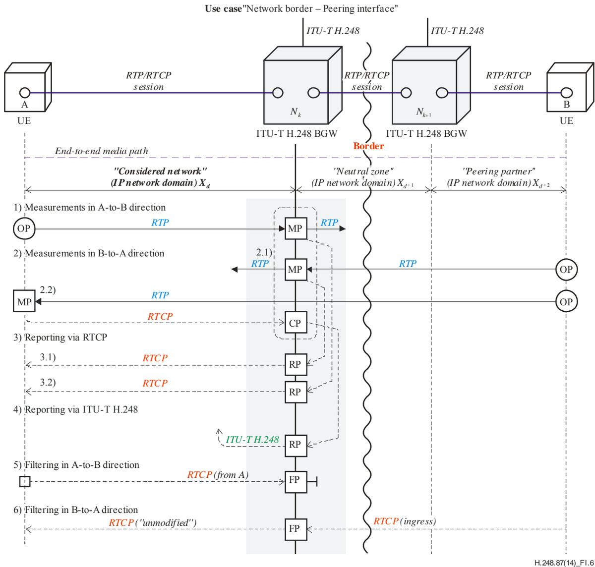
**Figure I.6 – Use case 6: IP-IP ITU-T H.248 MG as peering node**
