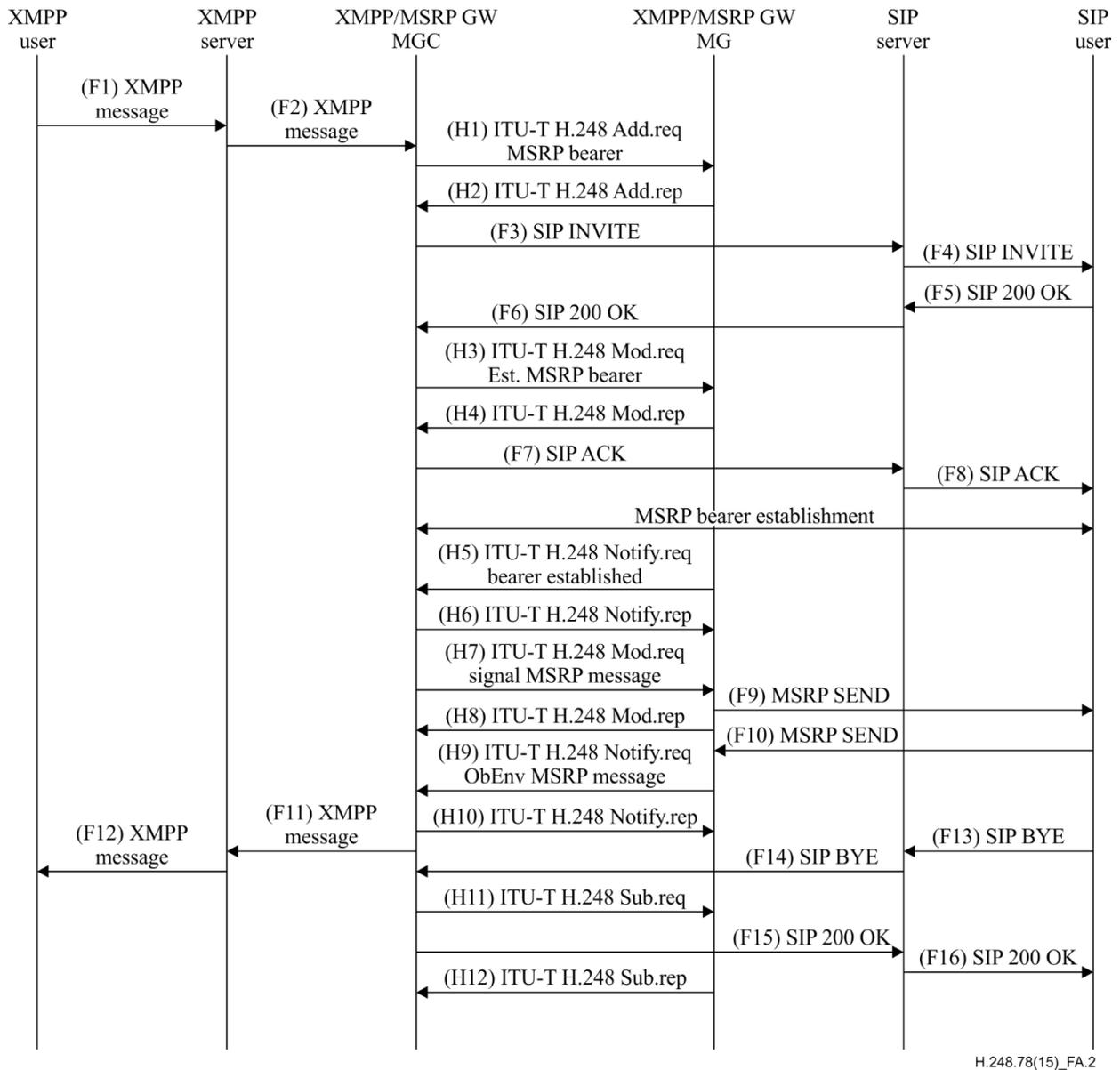
Figure A.2 – XMPP to MSRP order of events in an ITU-T H.248 controlled gateway
