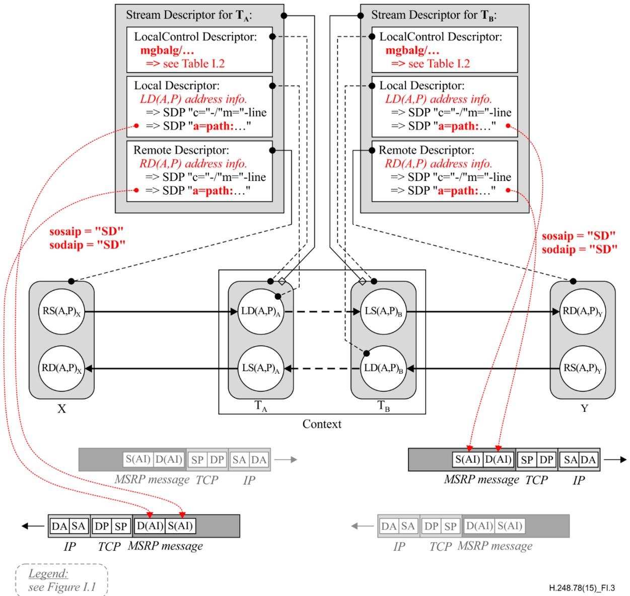
**Figure I.3 – Use case "Bidirectional B-ALG with source and destination address information translation" – MSRP bearer traffic**
