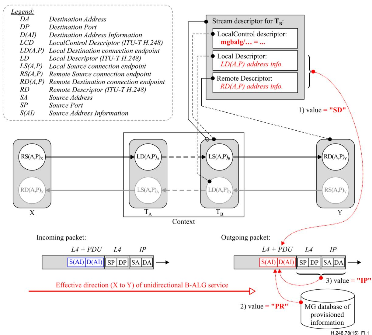
**Figure I.1 – Concept of MG located bearer level ALG service**
