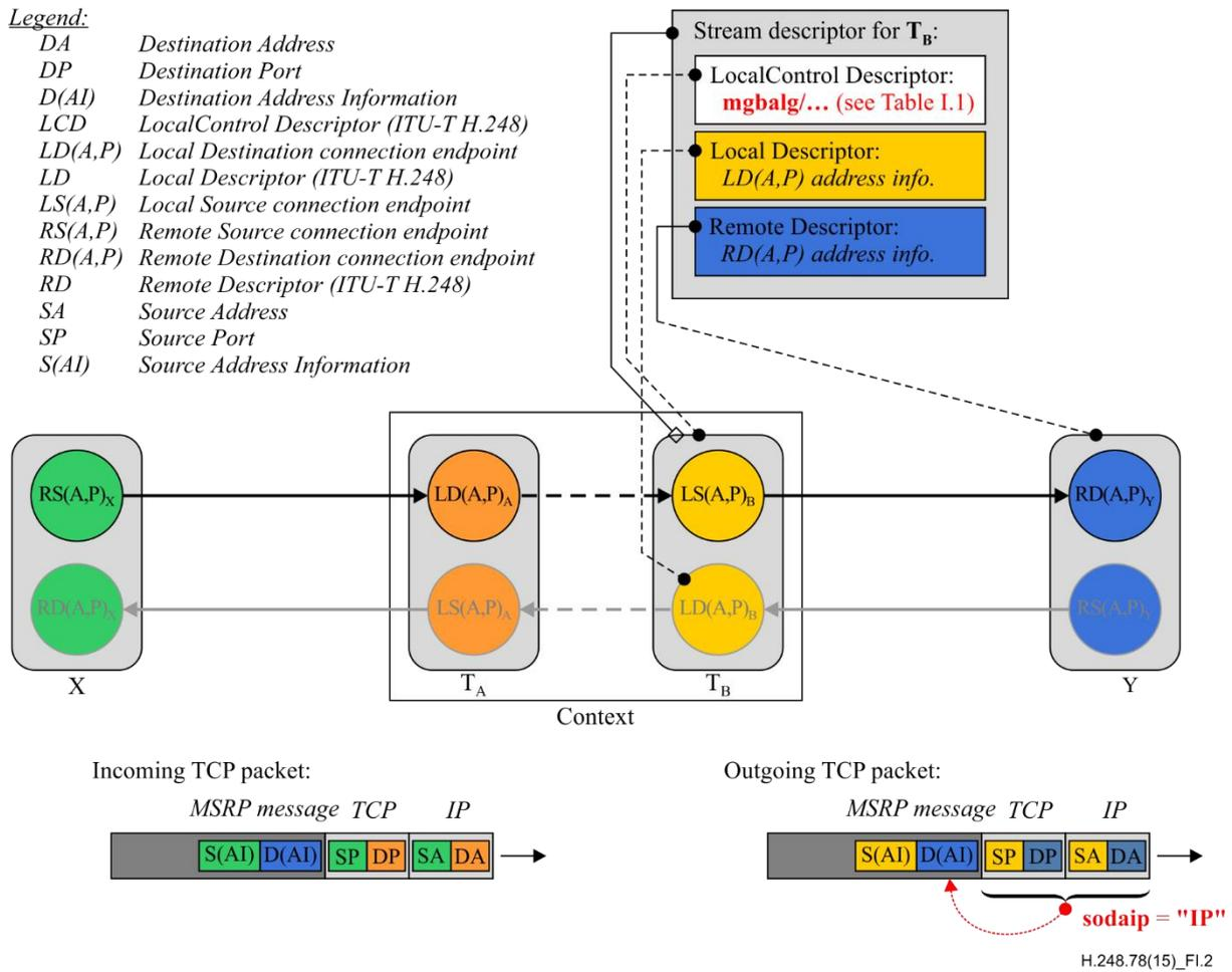
**Figure I.2 – Use case "Unidirectional B-ALG with destination address information translation" – MSRP bearer traffic**
