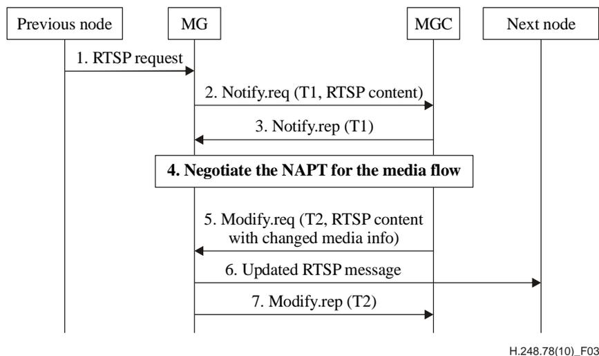
**Figure 3 – RTSP and media traversal signalling flow**
