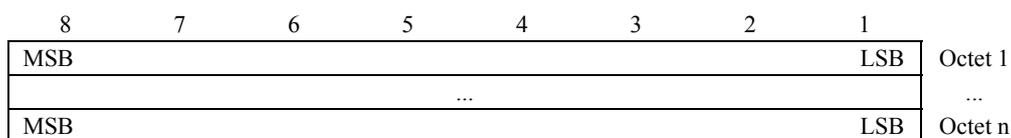
NOTE – Octet 1 contains the most significant octet of data.
