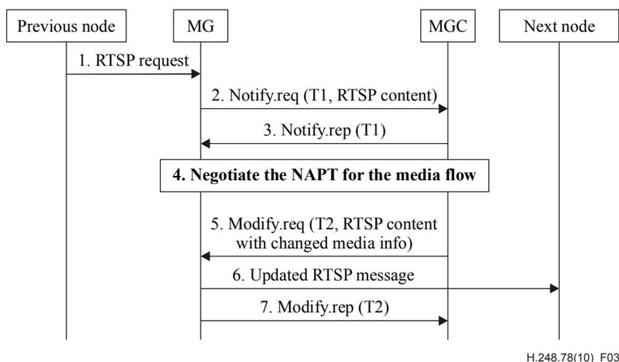
**Figure 3 – RTSP and media traversal signalling flow**
