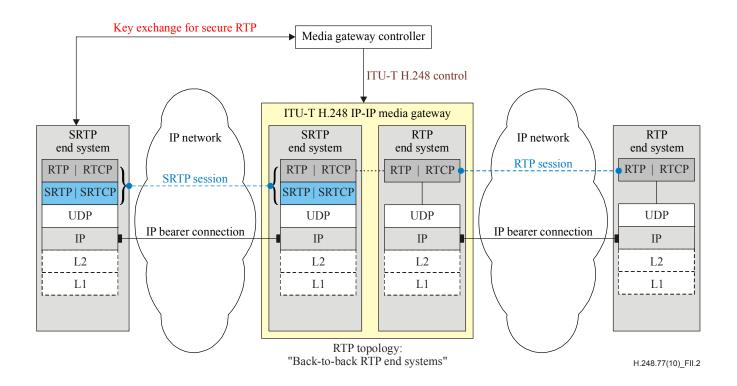
Figure II.2 – Use case #2: SRTP to RTP ITU-T H.248 MG
