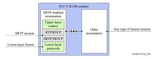
Figure 1 – Two-termination context with a SRTP termination
