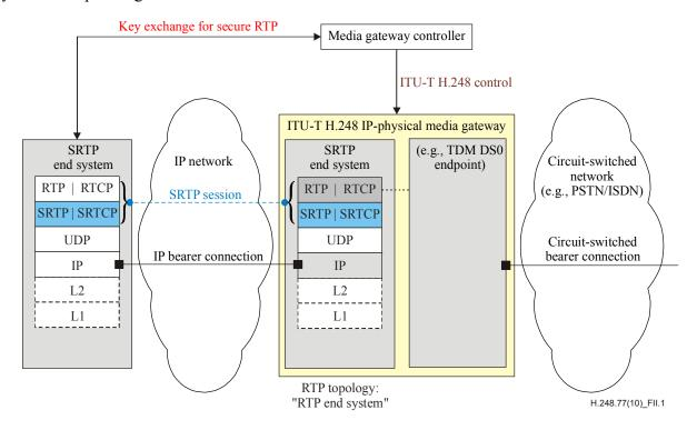
Figure II.1 – Use case #1: SRTP to circuit-switched ITU-T H.248 MG
