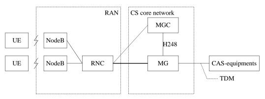
NOTE – Left side of MG: radio access network of the 3GPP defined 3G PLMN: Right side: legacy PSTN with a CAS-based NNI; Middle: 3GPP R3+ CS CN domain with Mc reference point between MSC server (MGC role) and CS-MGW.
