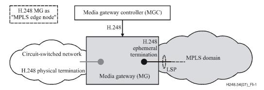
Figure I.1 - H.248 MG as MPLS edge node
