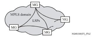
NOTE 1 – One example could be the interconnection of MGs by an MPLS infrastructure in NGN PSTN emulation subsystems (PES) core networks. [ITU-T Y.2261] depicts two PES scenarios based on (a) TMGs only and (b) TMGs and AMGs.
