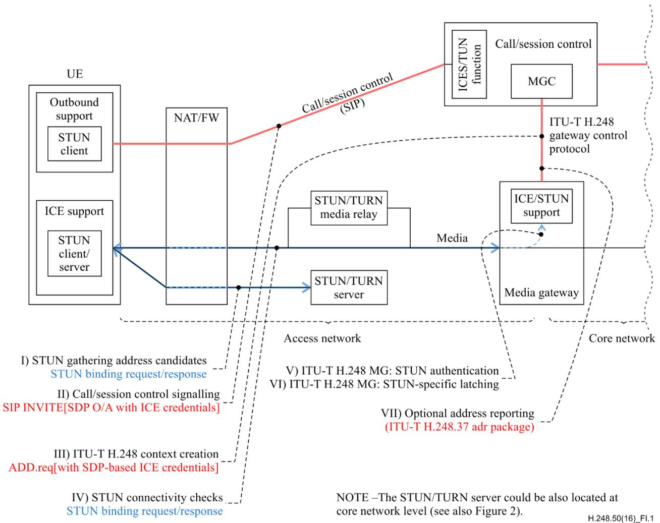
**Figure I.1 – Network model for ITU-T H.248 IP access gateways (derived from Figure 2 with scope on half call only)**
