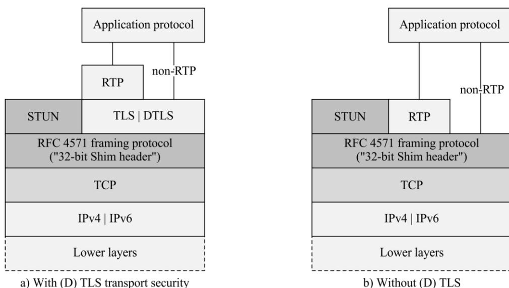
**Figure II.1 – ICE for TCP – protocol stack (MG bearer interface)**
