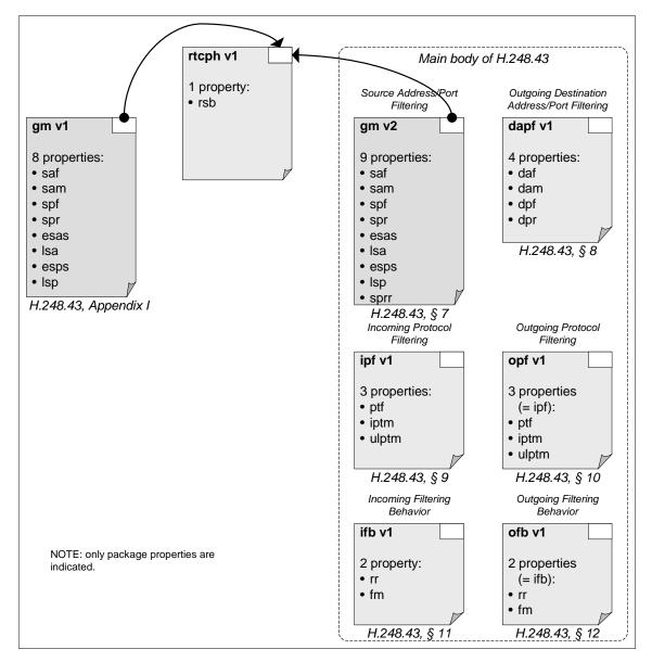
Figure II.1 – Overview of packages for gate management and gate control
