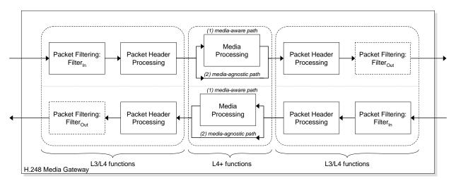
Figure 1 – General model for IP-to-IP interworking
