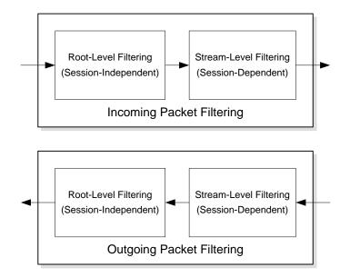
**Figure 3 – Interaction of root and stream level filtering**
