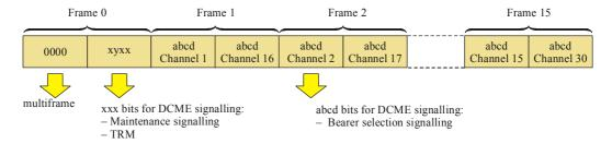
NOTE 1- Channel numbers refer to telephone channel numbers. 64 kbit/s channel time slots 1 to 15 and 17 to 31 are assigned to telephony channels numbered from 1 to 30.
