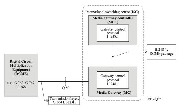
Figure 1/H.248.42 – Scope of the DCME Package
