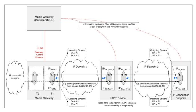
NOTE – The single H.248 stream at Termination T1 relates to the two IP flows of the bidirectional IP connection.
