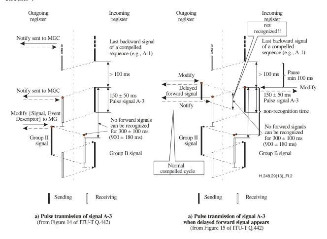
Figure I.2 – Time sequence of a pulsed transmission signal based on [ITU-T Q-Sup.7]
