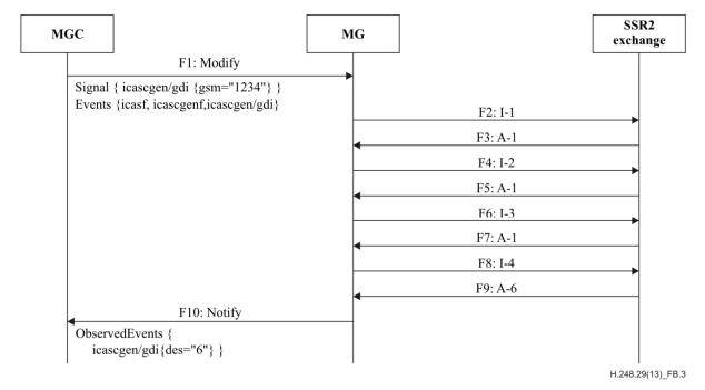
NOTE – SSR2 interregister signalling codepoints shown are Group I Forward Signals defined in Table 6 of [ITU-T Q.441], and Group A Backward Signals defined in Table 8 of [ITU-T Q.441].
