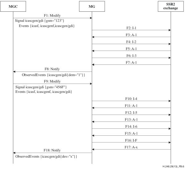
NOTE – SSR2 interregister signalling codepoints shown are Group I Forward Signals defined in Table 6 of [ITU-T Q.441], and Group A Backward Signals defined in Table 8 of [ITU-T Q.441].
