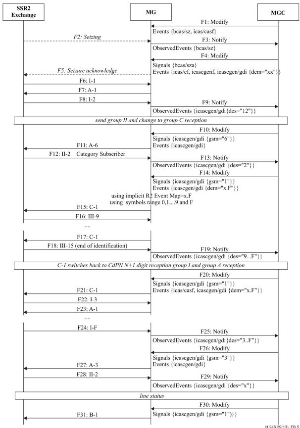
NOTE – SSR2 interregister signalling codepoints used here are Group II Forward Signals defined in Table 7 of [ITU-T Q.441], Group III Forward Signals and Group C Backward Signals to show an example of national extensions. The exact definitions of these codepoints are not relevant here.
