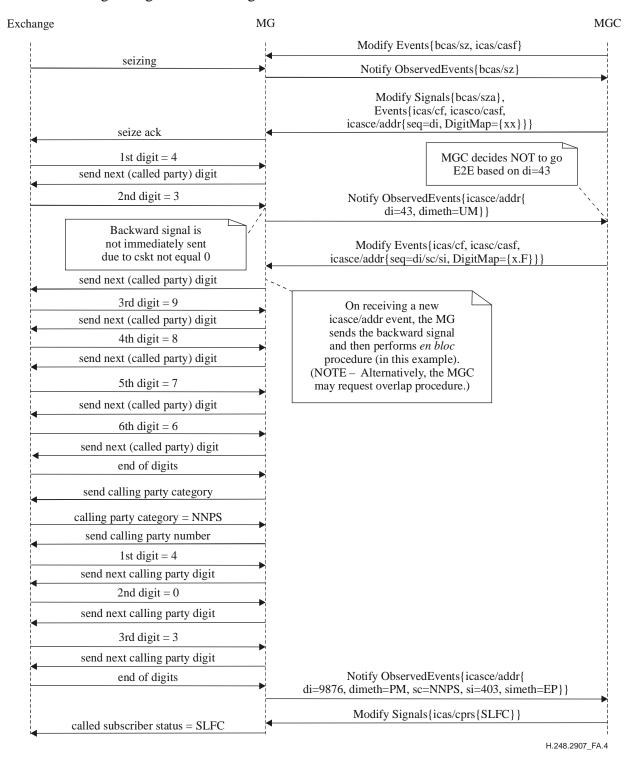
Figure A.4 – Example where MGC decides NOT to use end-to-end signalling
