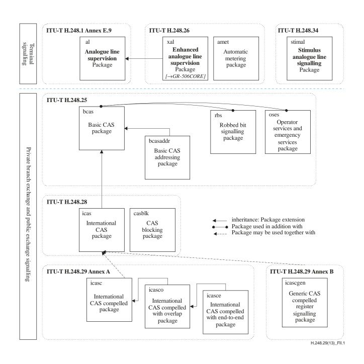
Figure II.1 – Survey of ITU-T H.248 packages for CAS (incl. ALS) interfaces
