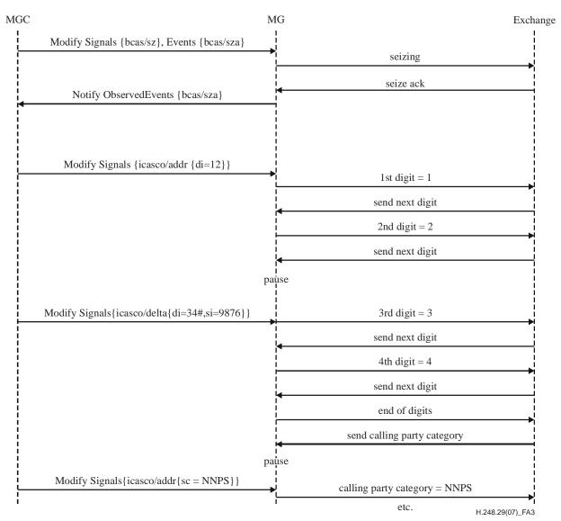
Figure A.3 – Outgoing overlap compelled register signalling example
