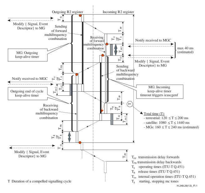
Figure I.1 – Time sequence of a complete compelled signalling cycle (based on [ITU-T Q.457])
