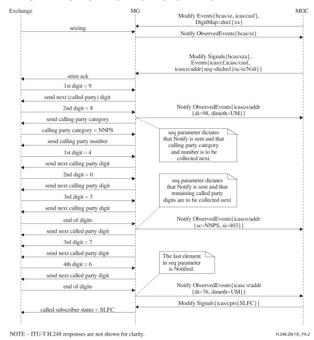
Figure A.2 – Incoming overlap compelled register signalling example
