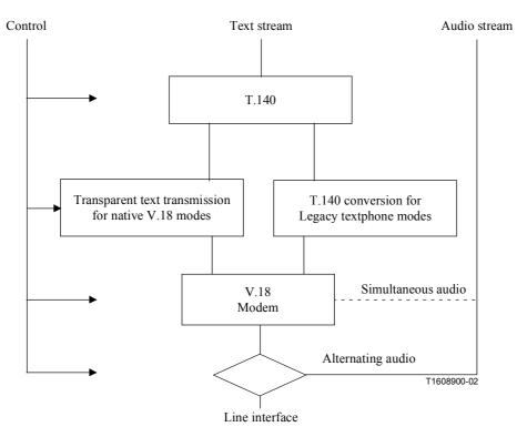
Figure 2/H.248.2 – Text telephone package functional view
