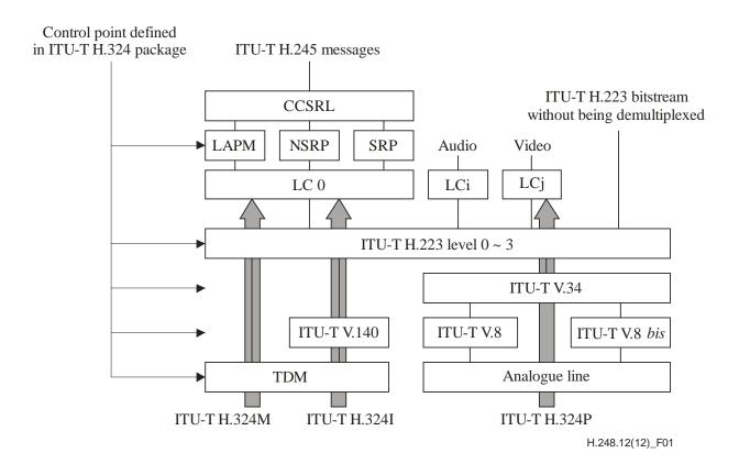
Figure 1 – Control point defined in ITU-T H.324 package
