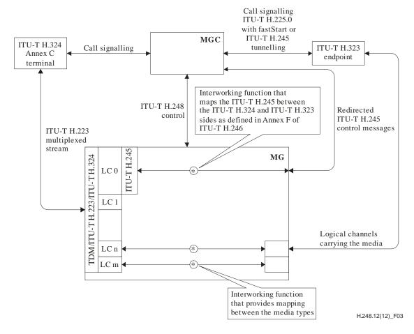
Figure 3 – Resource control at the MG (with fastStart/ITU-T H.245 tunnelling)
