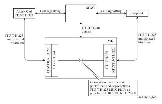
Figure 5 – Configuration for IP tunnelling of Annex C of ITU-T H.324 bitstream
