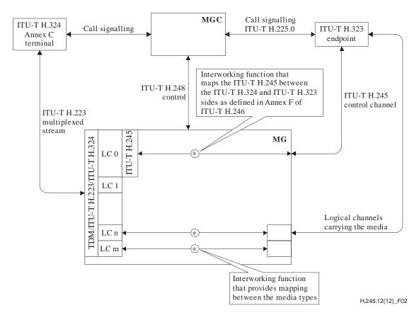
Figure 2 – Resource control at the MG (without fastStart/H.245 tunnelling)
