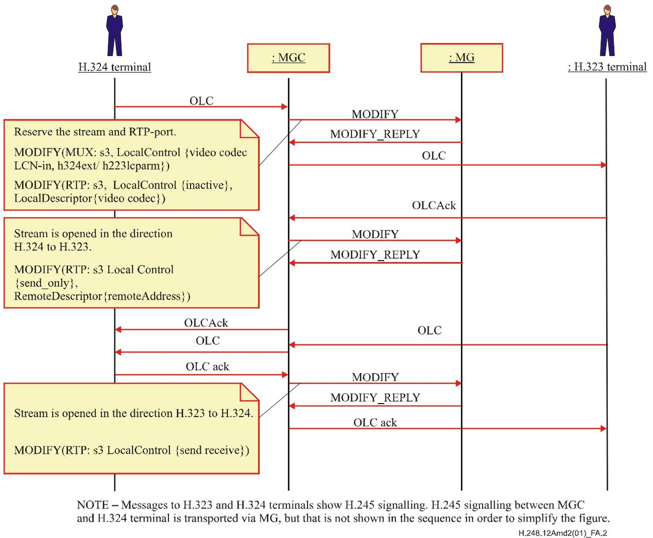
**Figure A.2/H.248.12 – Sequence diagram for opening the logical channel**
