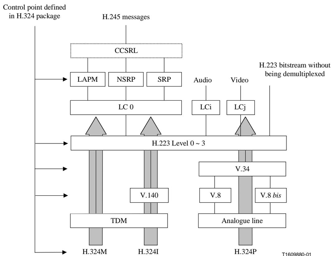
Figure 1/H.248.12 – Control point defined in H.324 package
