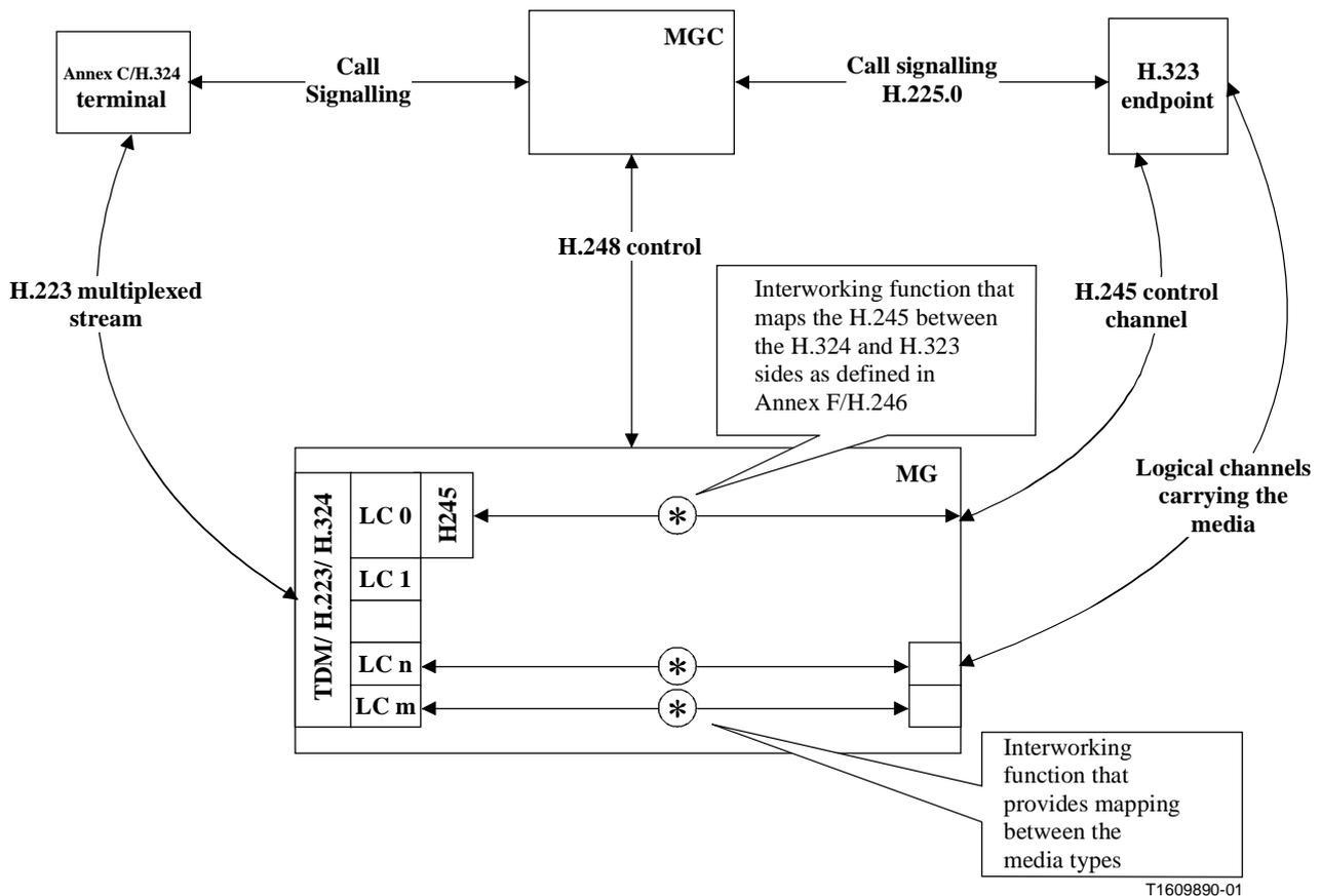
**Figure 2/H.248.12 – Resource control at the MG (without fastStart/H.245 tunnelling)**
