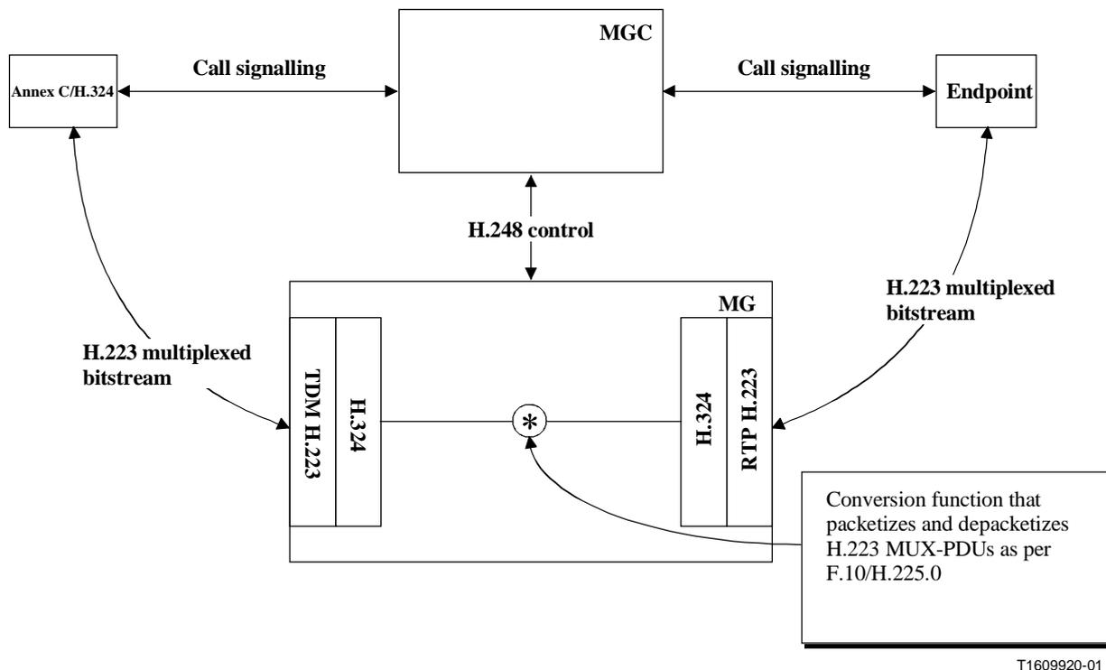
Figure 5/H.248.12 – Configuration for IP tunnelling of Annex C/H.324 bitstream
