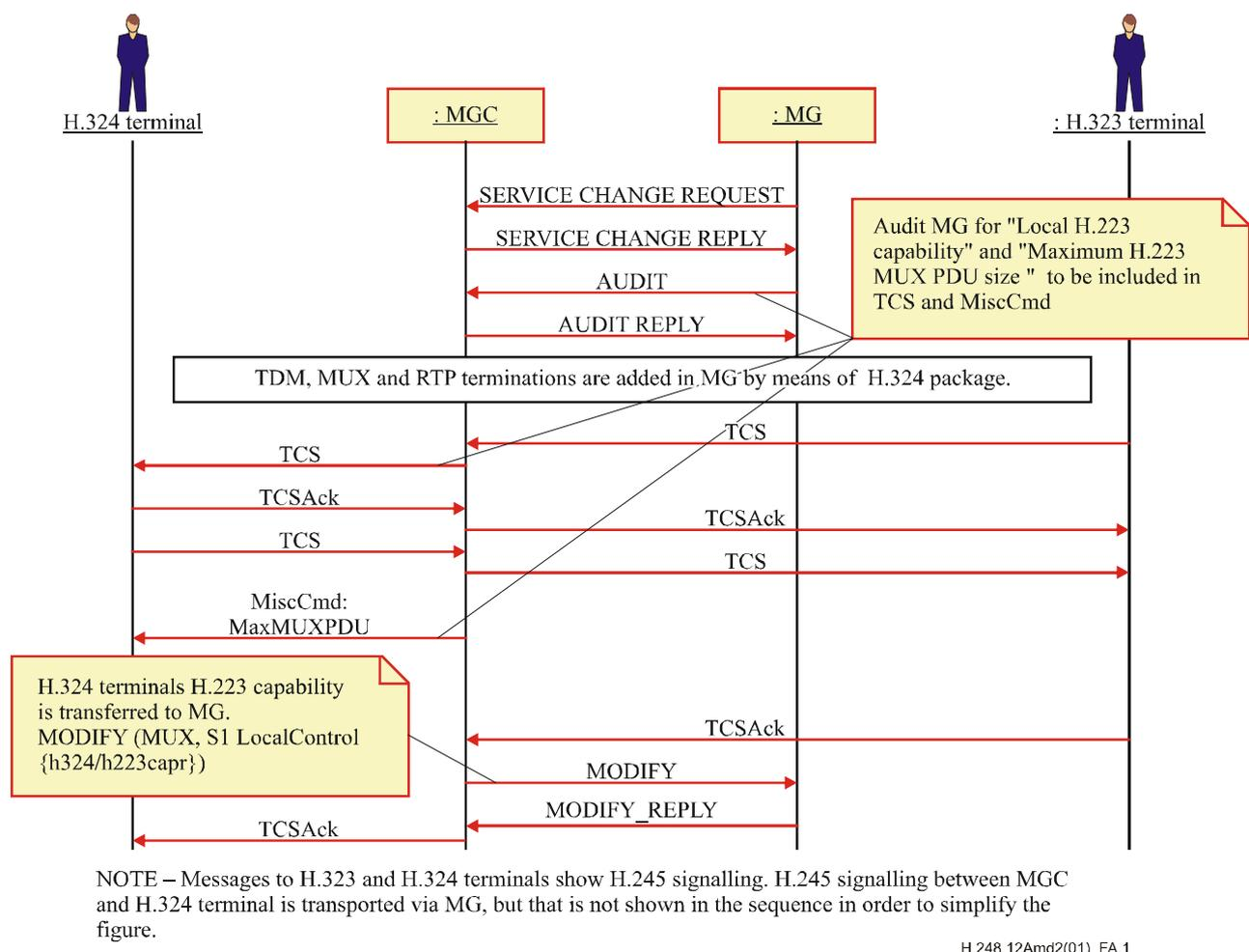
**Figure A.1/H.248.12 – Sequence diagram terminal capability exchange at H.324 and H.323 interworking**
