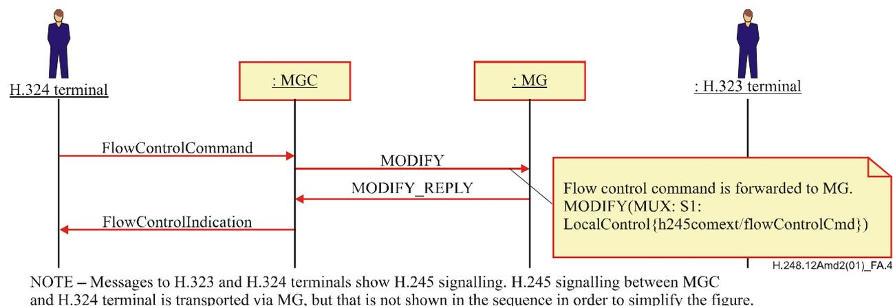
**Figure A.4/H.248.12 – Sequence diagram for flow control modification**
