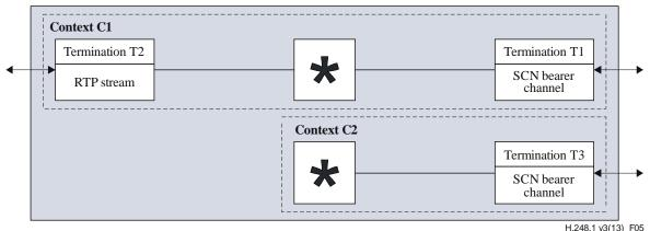
Figure 5 – Example call waiting scenario/alerting applied to T1
