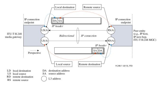
Figure 3 – Connection endpoint naming conventions – IP connection
