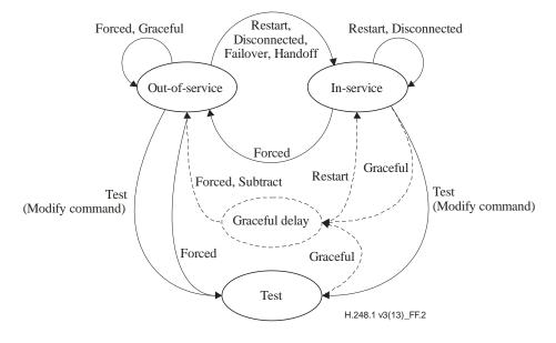
Figure F.2 – Simple ServiceChange state model
