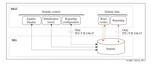
Figure IV.1 – Categories of MGC operations on statistics ('Reporting' requires support of [b-ITU-T H.248.47])
