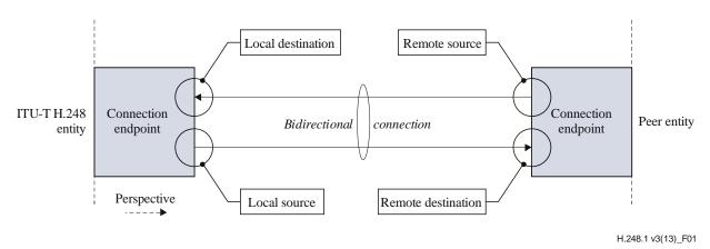
Figure 1 – Connection endpoint naming conventions – Generic concept
