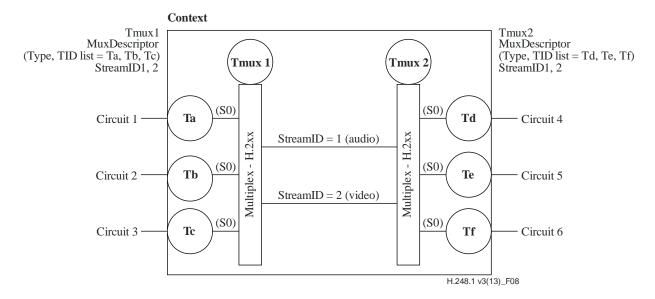
Figure 8 – Multiplexed termination scenario – Circuit-to-circuit
