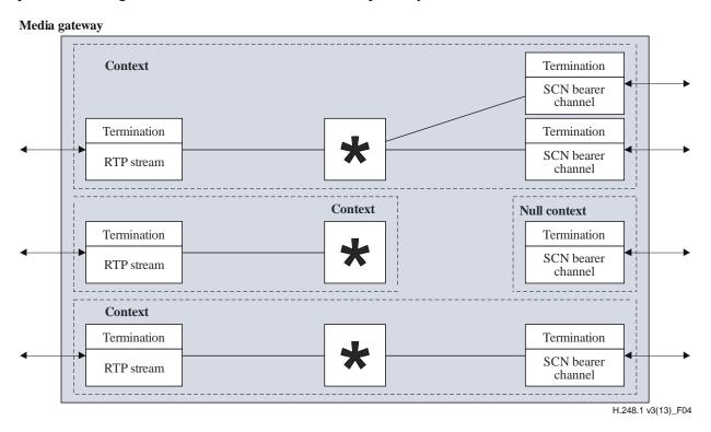
Figure 4 – Example of ITU-T H.248.1 connection model
