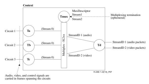
Figure 7 – Multiplexed termination scenario – Circuit-to-packet
