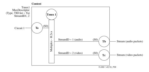
Figure 9 – Multiplexed termination scenario – Single-to-multiple terminations
