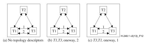
Figure 12 – Example topology at stream level
