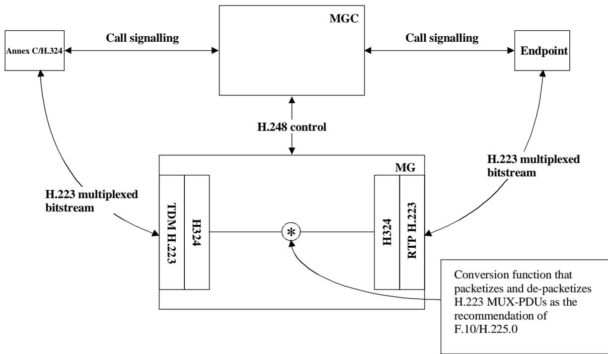
Figure M4-5/H.248 – Configuration for IP tunnelling of Annex C/H.324 bitstream
