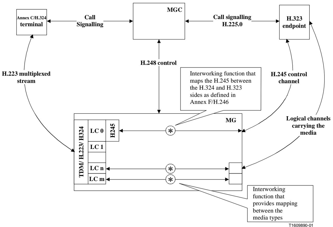
**Figure M4-2/H.248 – Resource control at the MG (without fastStart/H.245 tunnelling)**
