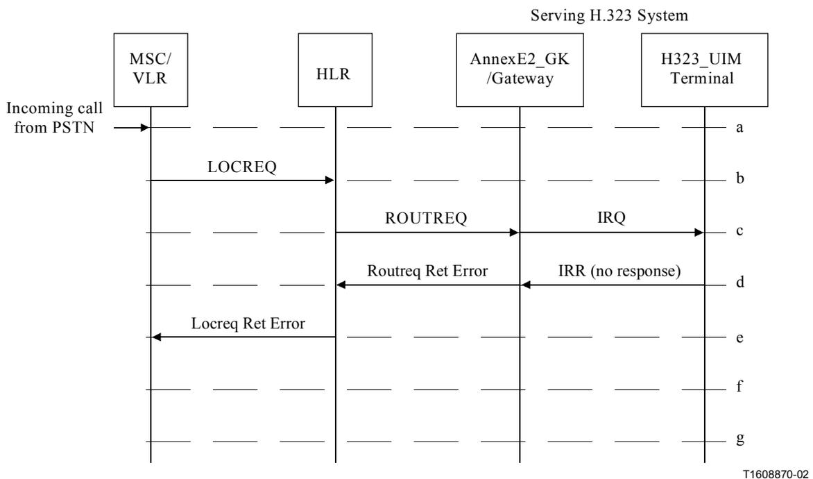
**Figure E2.7/H.246 – Unsuccessful call delivery to an ANSI-41 subscriber roaming in an H.323 network**
