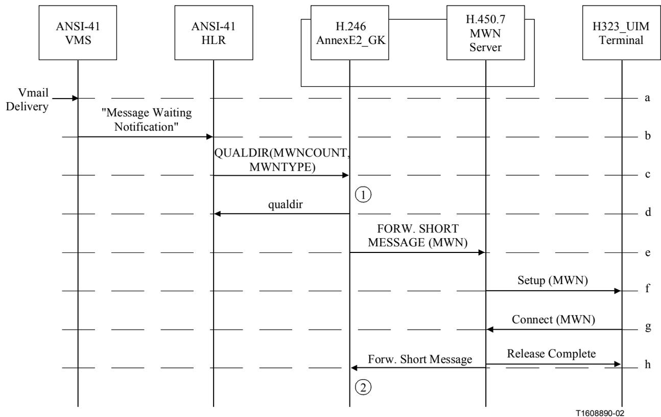
**Figure E2.9/H.246 – Message Wait Notification for the ANSI-41 Subscriber roaming in H.323 Networks messages flow**
