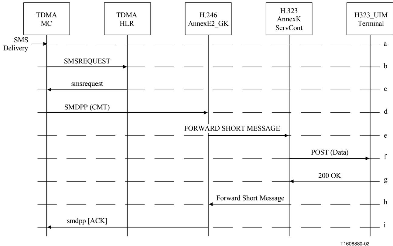
**Figure E2.8/H.246 – Short Message Delivery to Subscriber's H323\_UIM Terminal while roaming in H.323 network**
