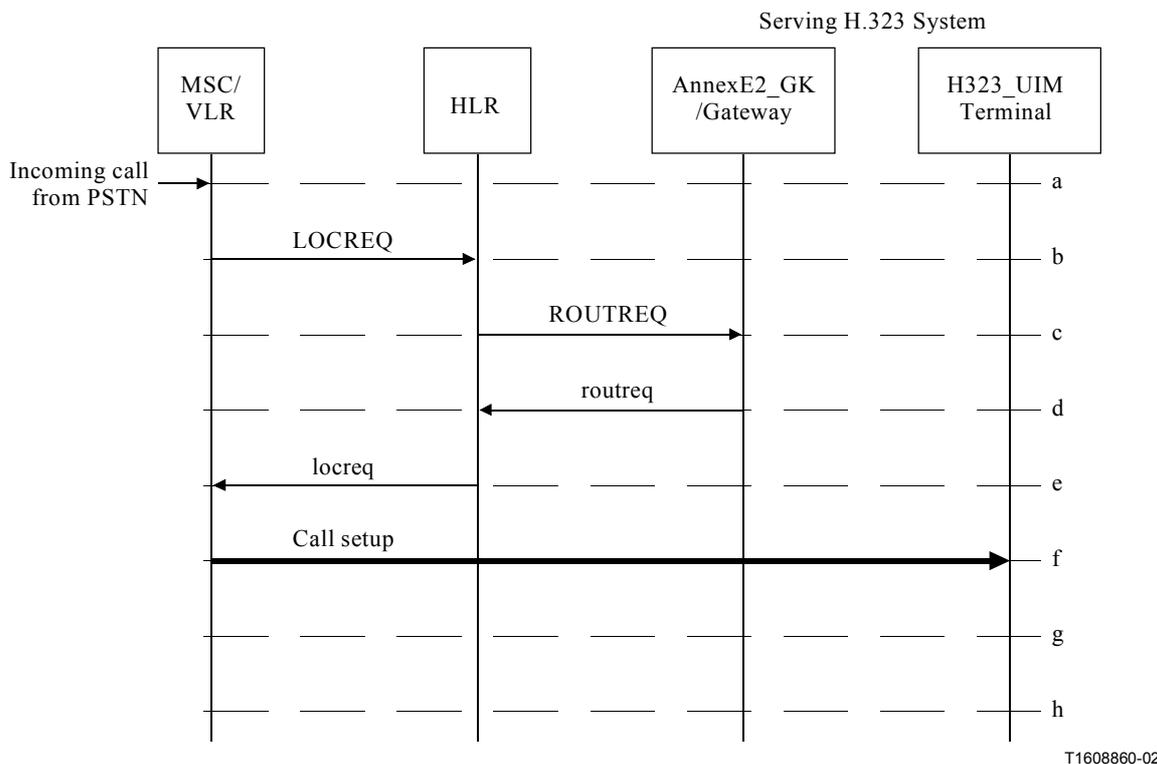
**Figure E2.6/H.246 – Call delivery to ANSI-41 subscriber roaming in an H.323 network**
