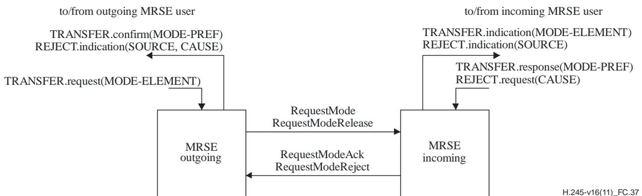
**Figure C.37 – Primitives and messages in the Mode Request Signalling Entity**
