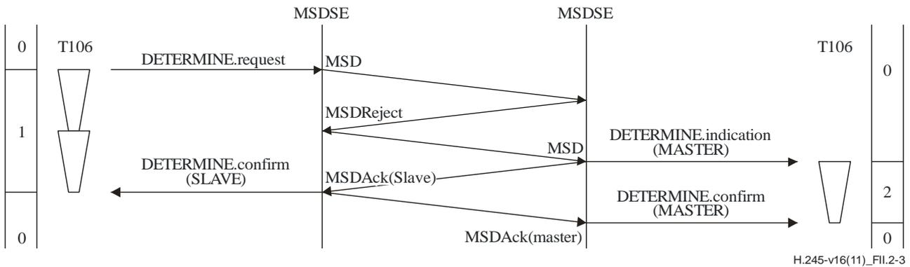
**Figure II.2-3 – Master-slave determination – First attempt produced an indeterminate result. The second attempt was successful**
