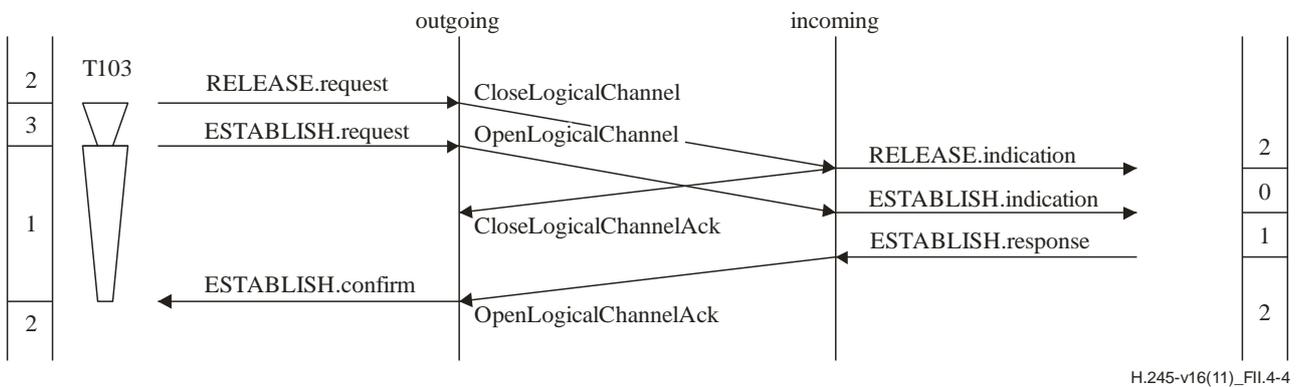
**Figure II.4-4 – Logical channel release followed by immediate re-establishment**
