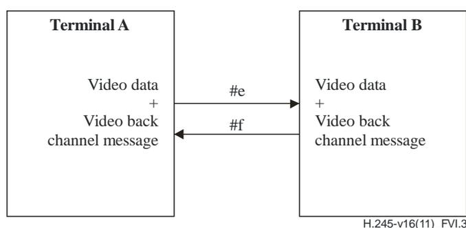
**Figure VI.3 – Logical channels for VideoMux mode**
