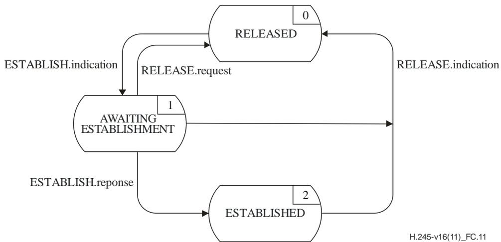
**Figure C.11 – State transition diagram for sequence of primitives at incoming LCSE**
