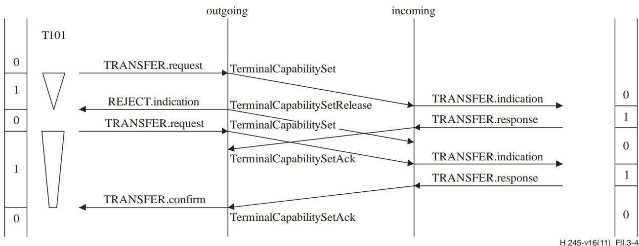
NOTE – The TerminalCapabilitySetRelease message arrives at the incoming CESE after response from the incoming CESE user. At the outgoing CESE the TerminalCapabilitySetAck message in response to the first TerminalCapabilitySet message is ignored. Only the second capability exchange is successful.
