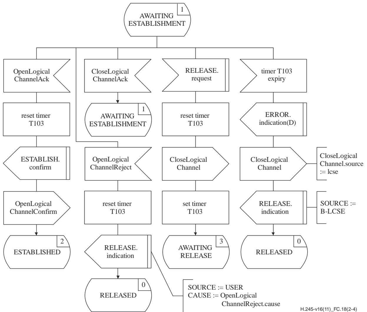
**Figure C.18 – Outgoing B-LCSE SDL (sheet 2 of 4)**
