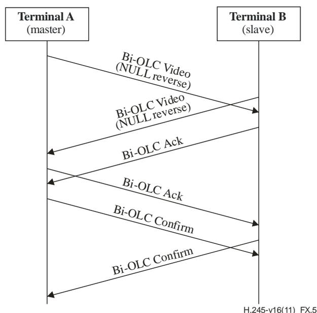
Figure X.5 – Both terminals propose bidirectional OLC with nullData
