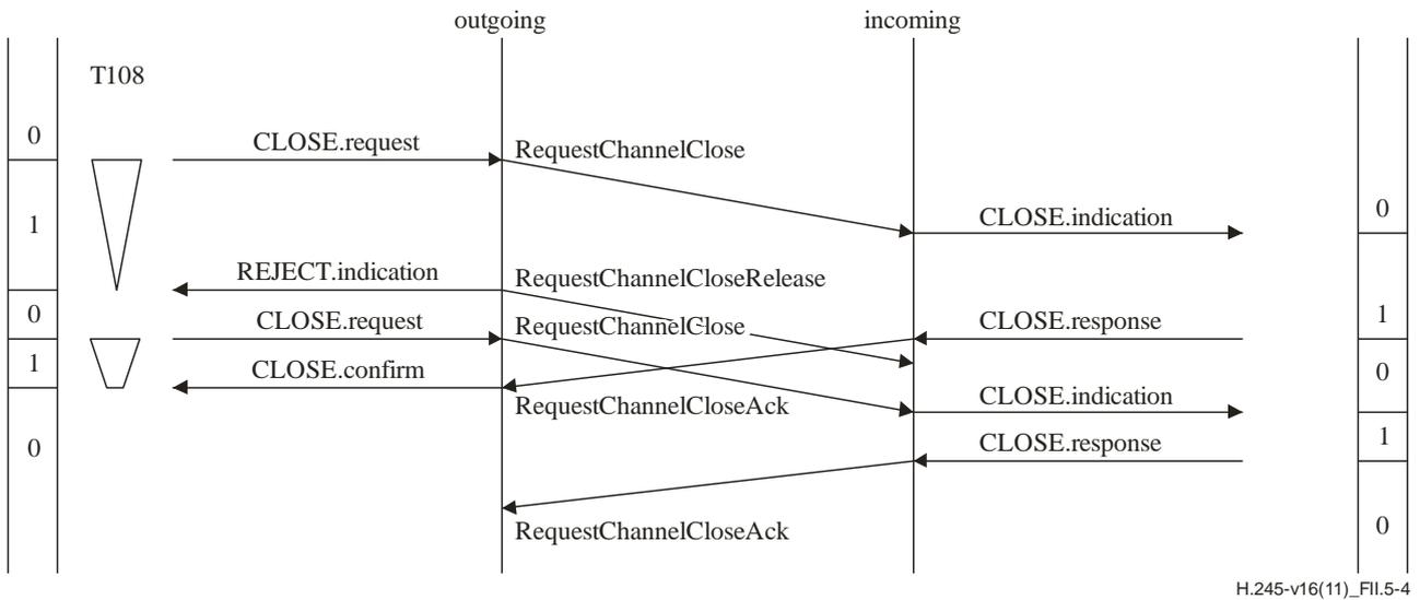
NOTE – The Close channel request is confirmed on reception of the first RequestChannelClose message.
