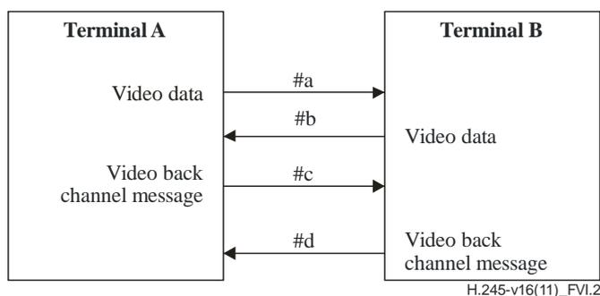
**Figure VI.2 – Logical channels for Separate Logical Channel mode**
