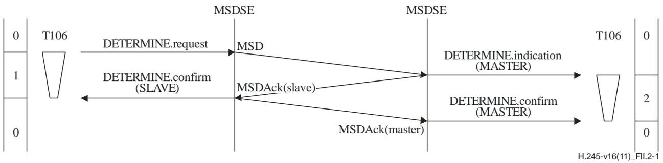
**Figure II.2-1 – Master-slave determination – Master at remote MSDSE**
