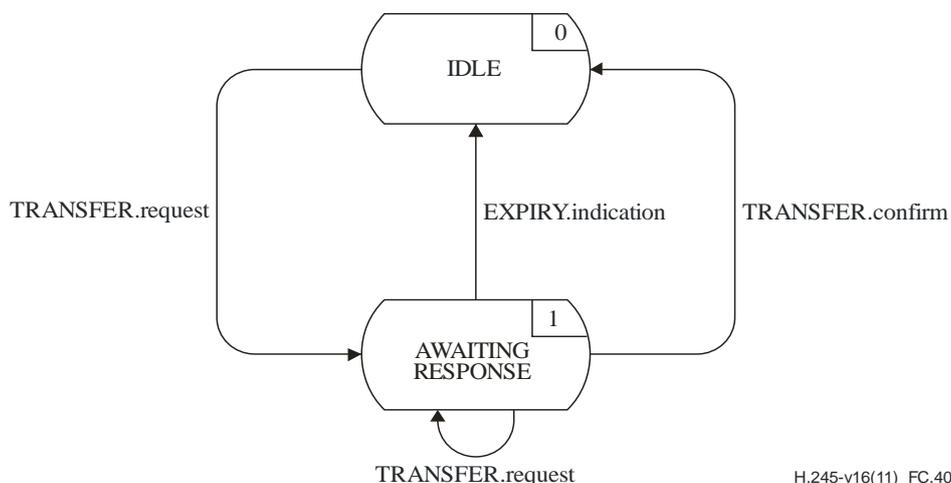
Figure C.40 – State transition diagram for sequence of primitives at RTDSE
