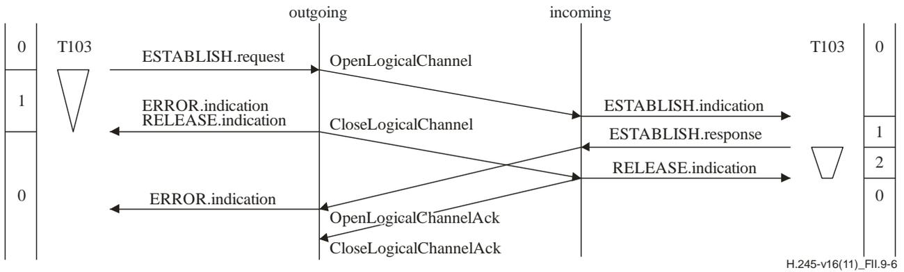
NOTE – Timer T103 at the outgoing side has expired after transmission of the OpenLogicalChannelAck message at the incoming B-LCSE, but before reception of the OpenLogicalChannelAck message at the outgoing B-LCSE.
