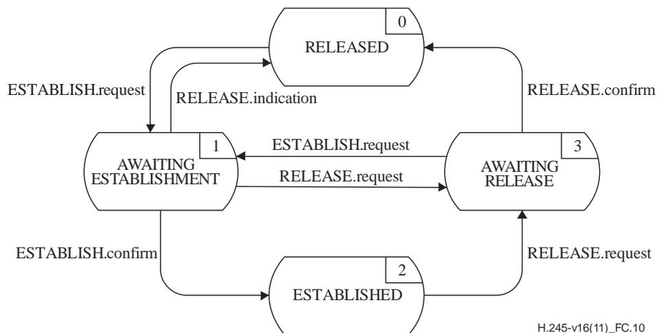
**Figure C.10 – State transition diagram for sequence of primitives at outgoing LCSE**
