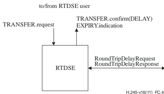
**Figure C.41 – Primitives and messages in the RTDSE**
