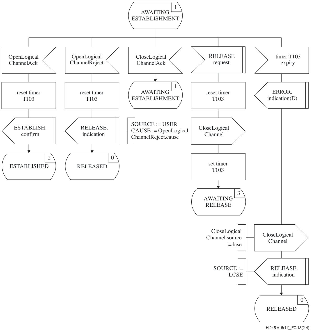
**Figure C.13 – Outgoing LCSE SDL (sheet 2 of 4)**
