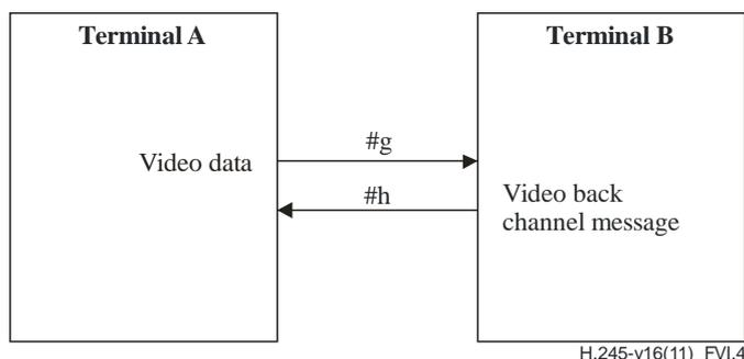
**Figure VI.4 – Separate Logical Channel mode in unidirectional video communication**
