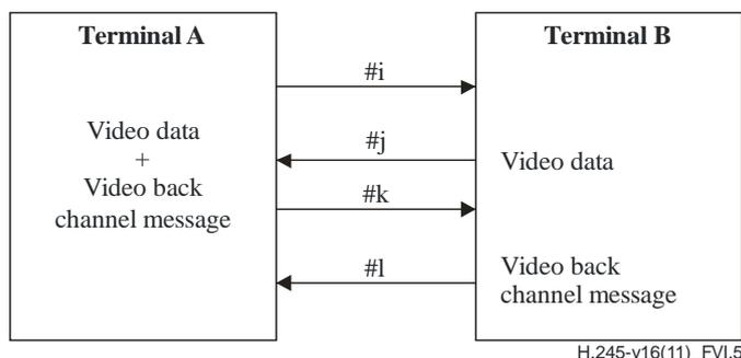
**Figure VI.5 – Coexistence of Separate Logical Channel mode with VideoMux mode**
