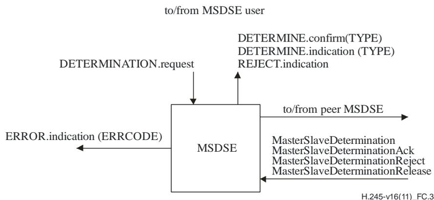
**Figure C.3 – Primitives and messages in the MSDSE**
