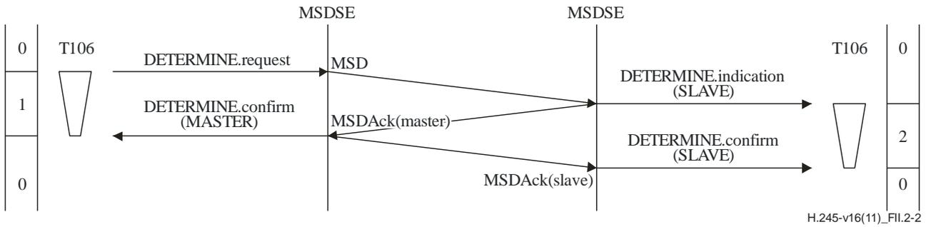
**Figure II.2-2 – Master-slave determination – Slave at remote MSDSE**
