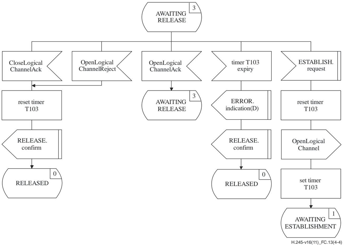
**Figure C.13 – Outgoing LCSE SDL (sheet 4 of 4)**
