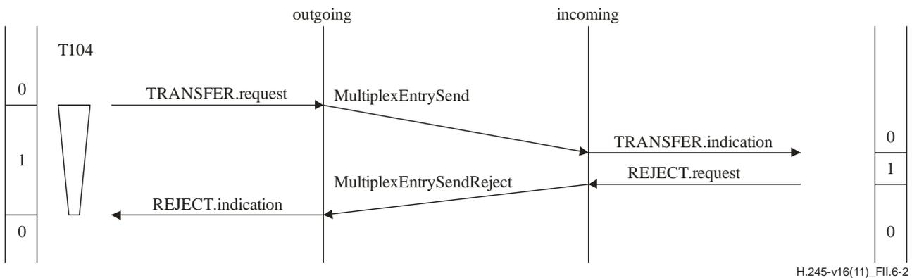
**Figure II.6-2 – Multiplex table send request with rejection from the peer MTSE user**
