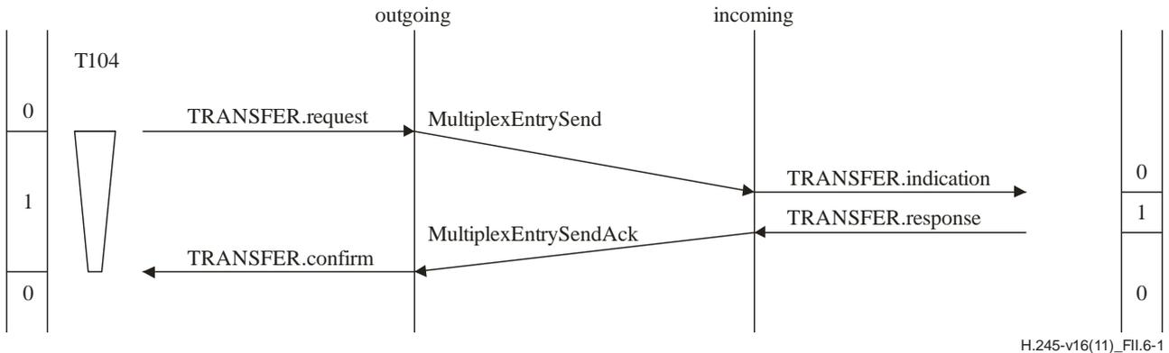
**Figure II.6-1 – Successful multiplex table send request**
