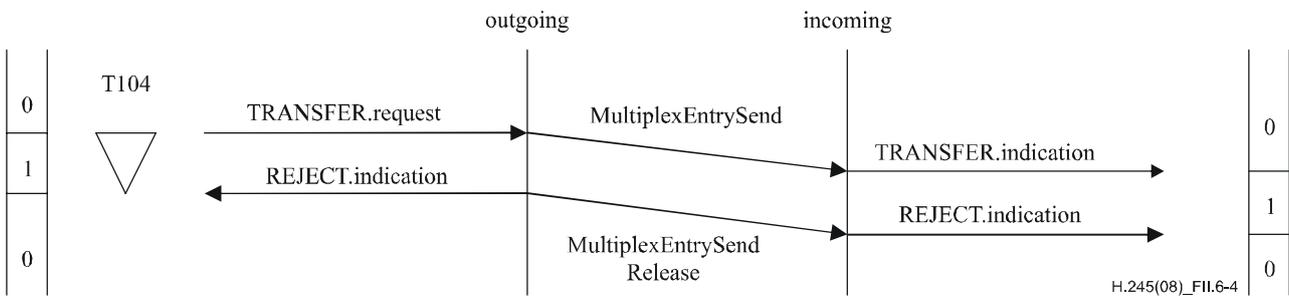
**Figure II.6-4 – Multiplex table send request with timer T104 expiry**
