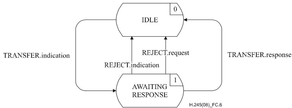
**Figure C.6 – State transition diagram for sequence of primitives at incoming CESE**
