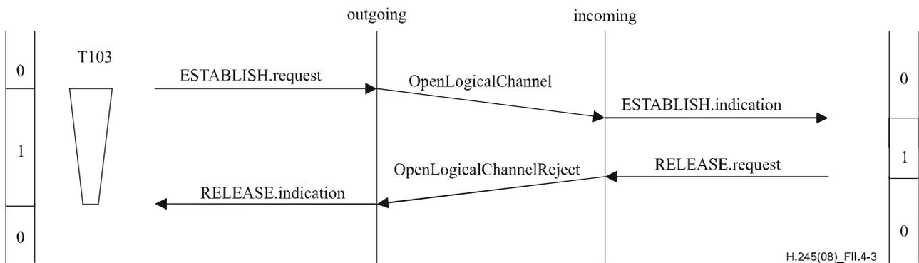
**Figure II.4-3 – Logical channel establishment rejection by peer LCSE user**
