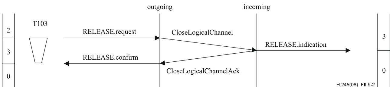
**Figure II.9-2 – Bidirectional logical channel release**
