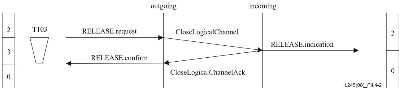
**Figure II.4-2 – Logical channel release**
