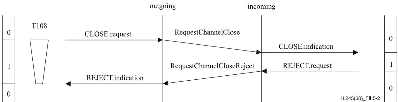
**Figure II.5-2 – Close logical channel request with rejection from peer incoming CLCSE user**
