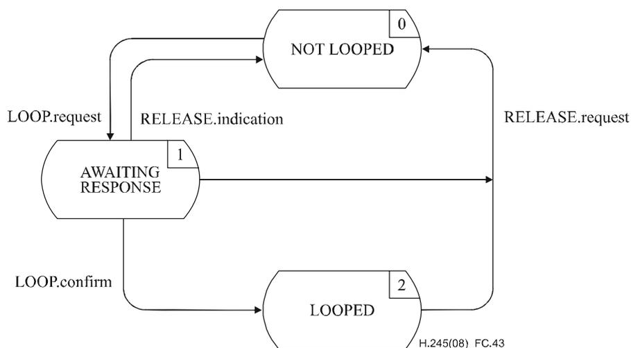
Figure C.43 – State transition diagram for sequence of primitives at outgoing MLSE
