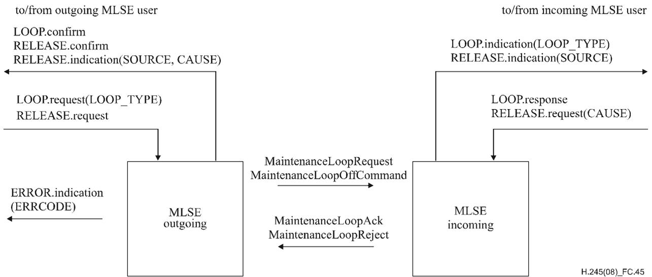
**Figure C.45 – Primitives and messages in the Maintenance Loop Signalling Entity**
