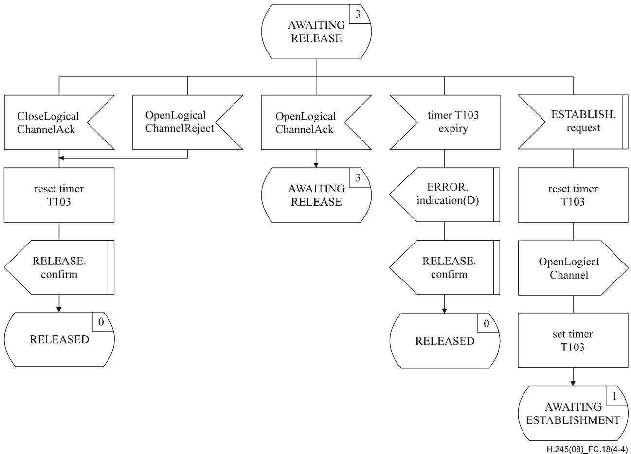
**Figure C.18 – Outgoing B-LCSE SDL (sheet 4 of 4)**
