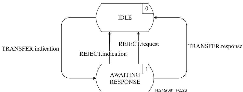
**Figure C.26 – State transition diagram for sequence of primitives at incoming MTSE**
