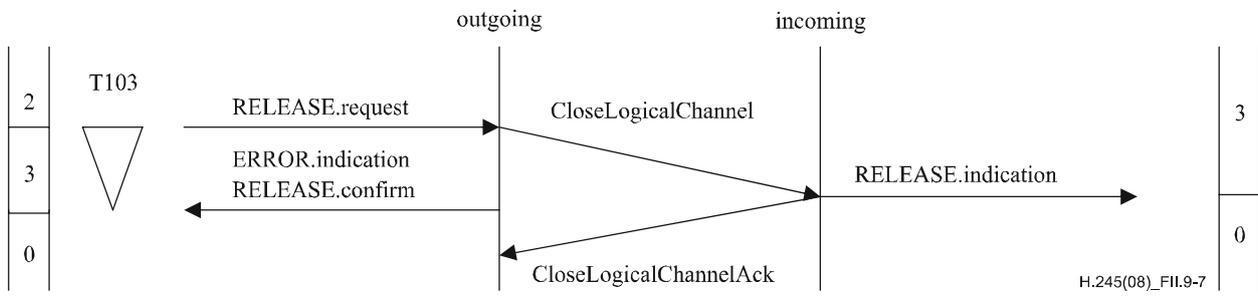
**Figure II.9-7 – Bidirectional logical channel release request with expiry of timer T103 at the outgoing side**
