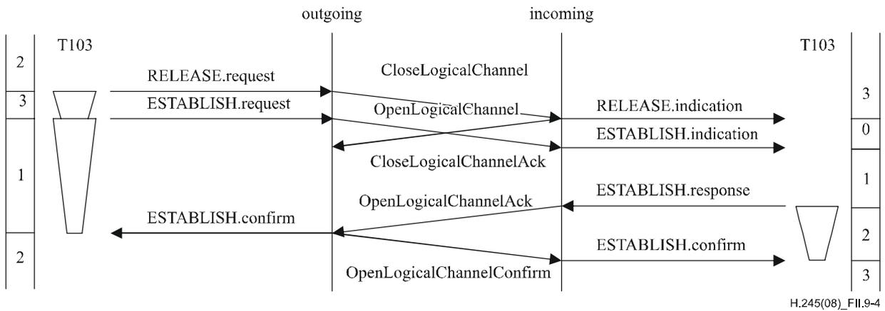
**Figure II.9-4 – Bidirectional logical channel release followed by immediate re-establishment**
