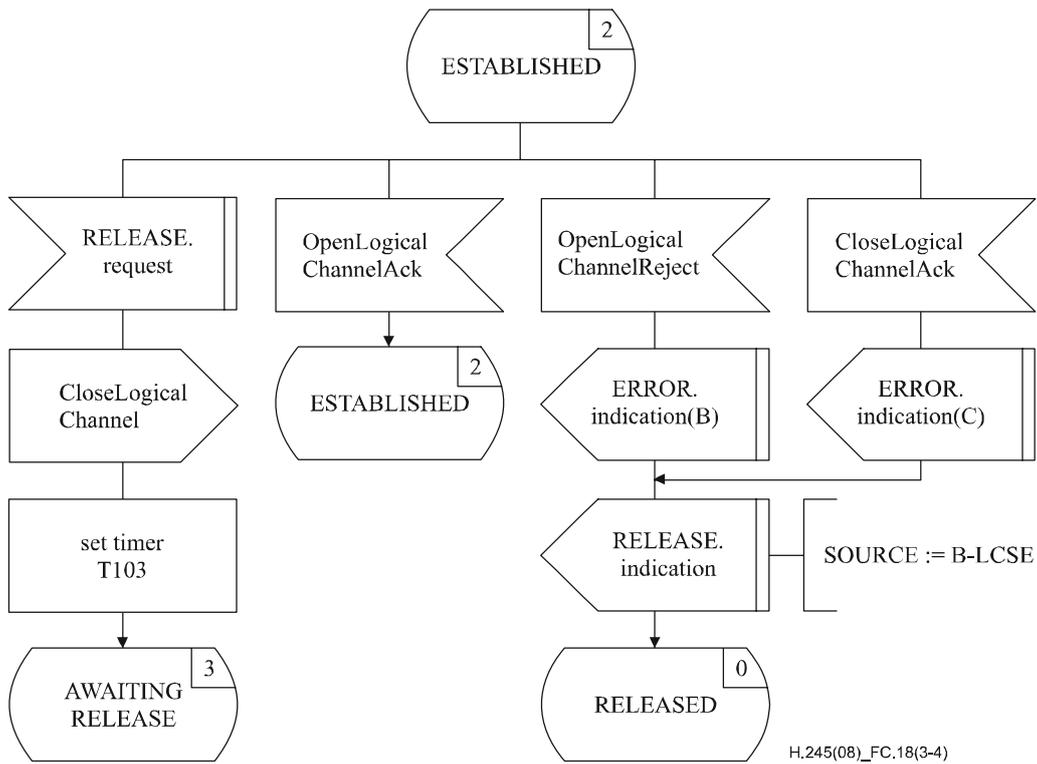
**Figure C.18 – Outgoing B-LCSE SDL (sheet 3 of 4)**
