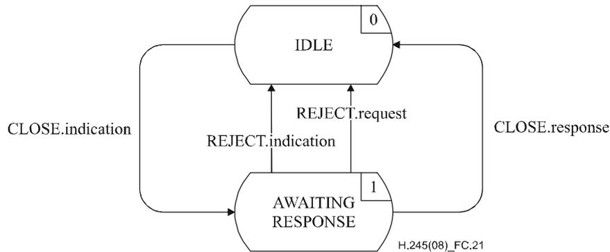
**Figure C.21 – State transition diagram for sequence of primitives at incoming CLCSE**
