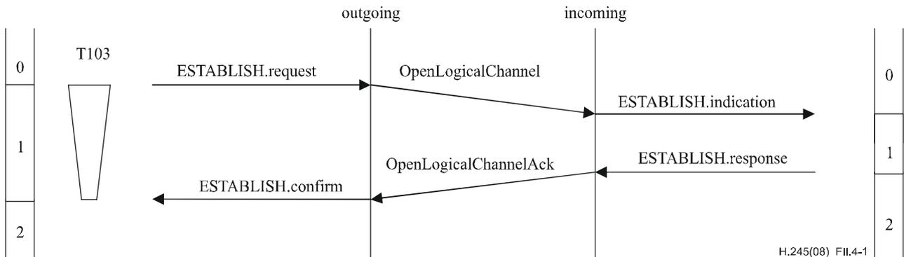
**Figure II.4-1 – Logical channel establishment**
