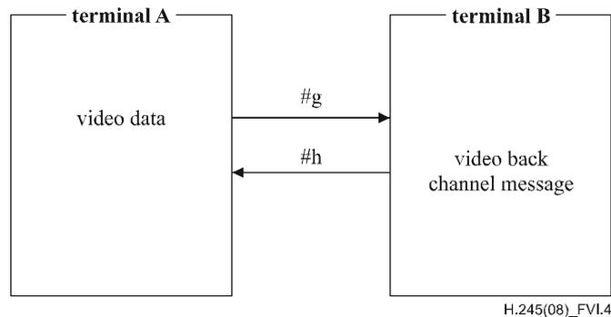
**Figure VI.4 – Separate Logical Channel mode in unidirectional video communication**
