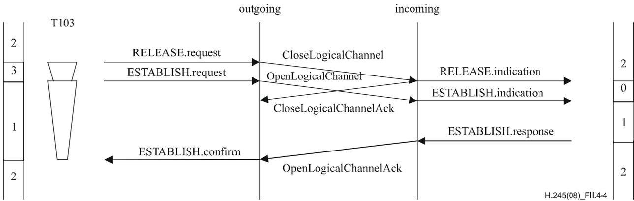
**Figure II.4-4 – Logical channel release followed by immediate re-establishment**
