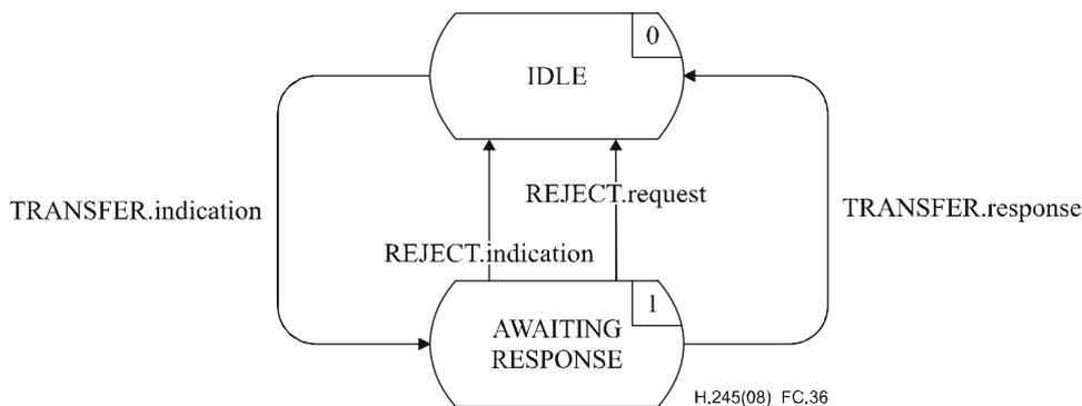
Figure C.36 – State transition diagram for sequence of primitives at incoming MRSE
