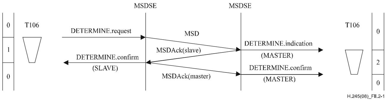
**Figure II.2-1 – Master-slave determination – Master at remote MSDSE**
