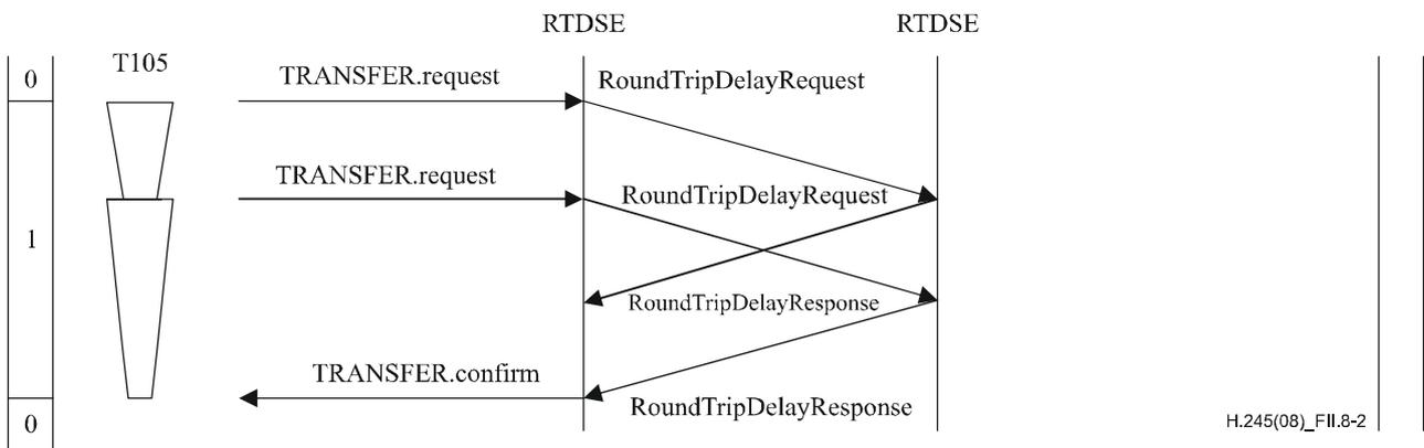
**Figure II.8-2 – Round-trip delay determination procedure with an earlier unacknowledged round-trip delay procedure outstanding**
