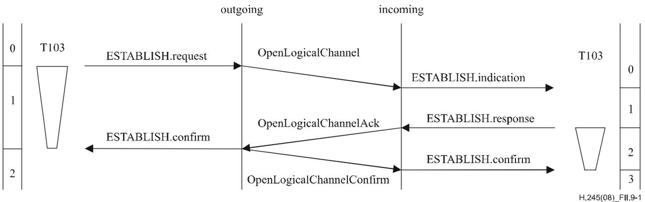
**Figure II.9-1 – Bidirectional logical channel establishment**
