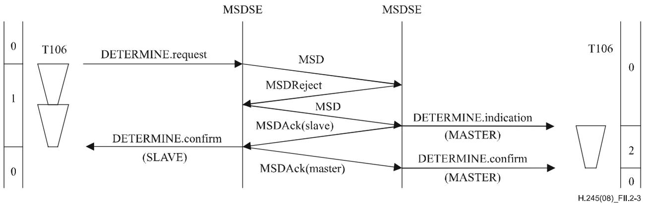
**Figure II.2-3 – Master-slave determination – First attempt produced an indeterminate result. The second attempt was successful**
