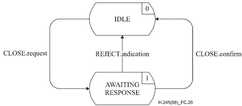
**Figure C.20 – State transition diagram for sequence of primitives at outgoing CLCSE**
