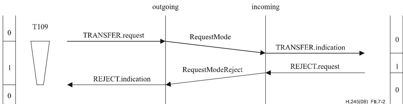
**Figure II.7-2 – Mode request with rejection from the peer MRSE user**
