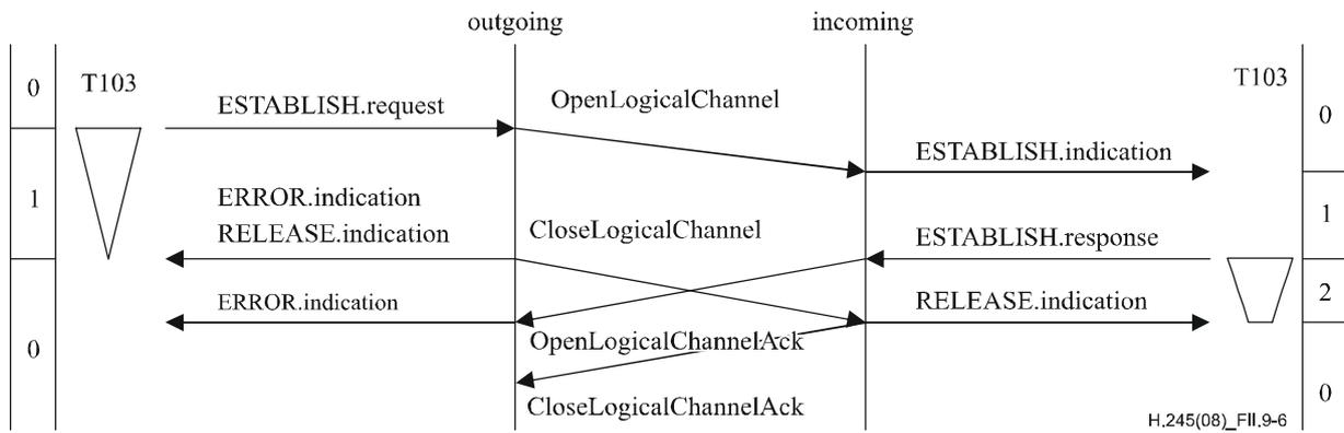
NOTE – Timer T103 at the outgoing side has expired after transmission of the OpenLogicalChannelAck message at the incoming B-LCSE, but before reception of the OpenLogicalChannelAck message at the outgoing B-LCSE.
