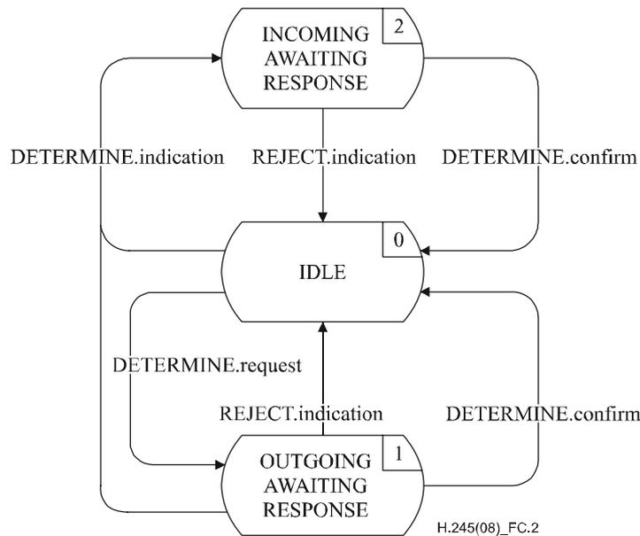
**Figure C.2 – State transition diagram for sequence of primitives at MSDSE**
