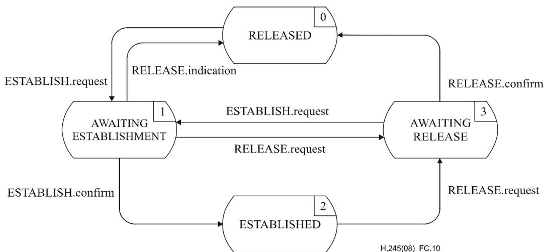
**Figure C.10 – State transition diagram for sequence of primitives at outgoing LCSE**
