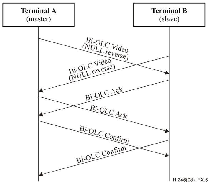
Figure X.5 – Both terminals propose bidirectional OLC with nullData
