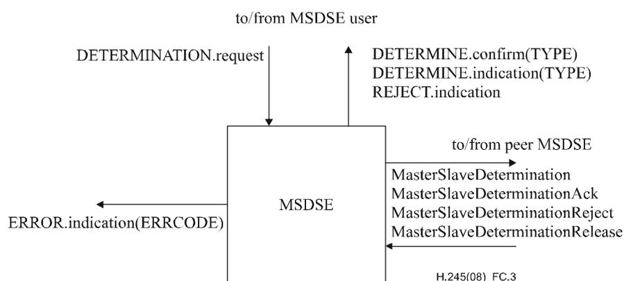
**Figure C.3 – Primitives and messages in the MSDSE**
