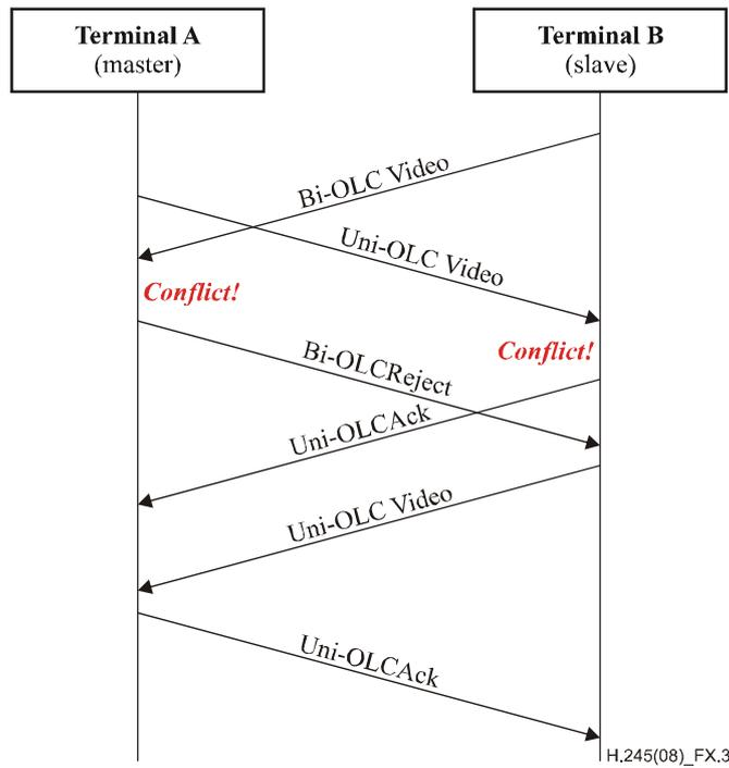
**Figure X.3 – Master proposes unidirectional OLC and slave proposes bidirectional OLC**
