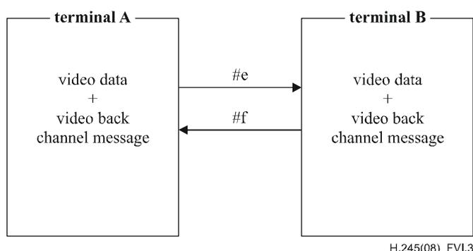
**Figure VI.3 – Logical Channels for VideoMux Mode**
