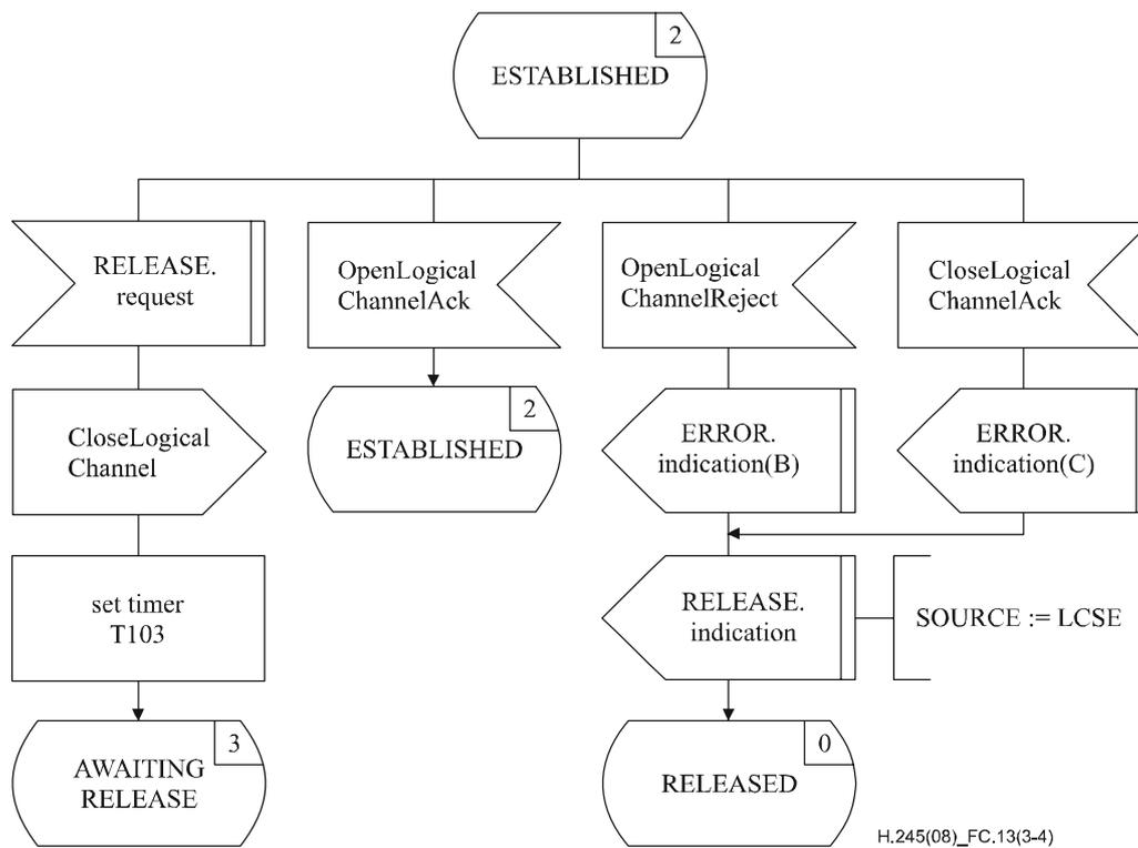
**Figure C.13 – Outgoing LCSE SDL (sheet 3 of 4)**
