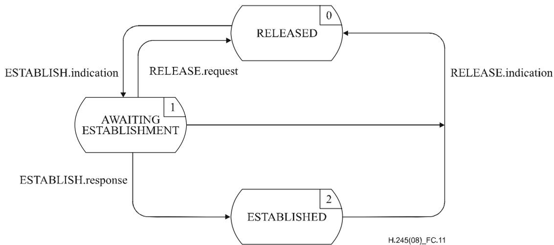
**Figure C.11 – State transition diagram for sequence of primitives at incoming LCSE**
