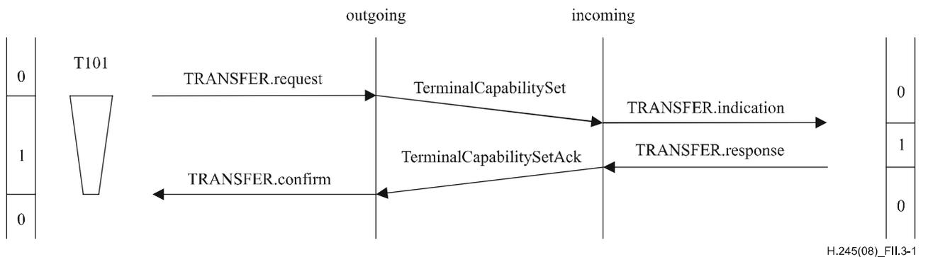
**Figure II.3-1 – Capability exchange with acceptance from the peer incoming CESE user**
