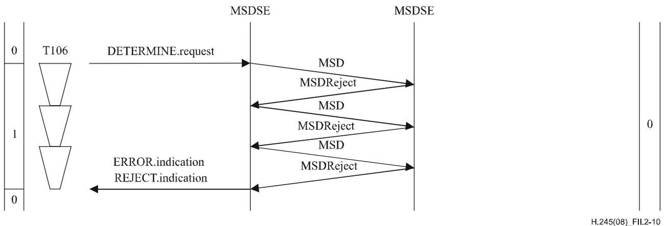
**Figure II.2-10 – Master-slave determination – Indeterminate result with N100 = 3**
