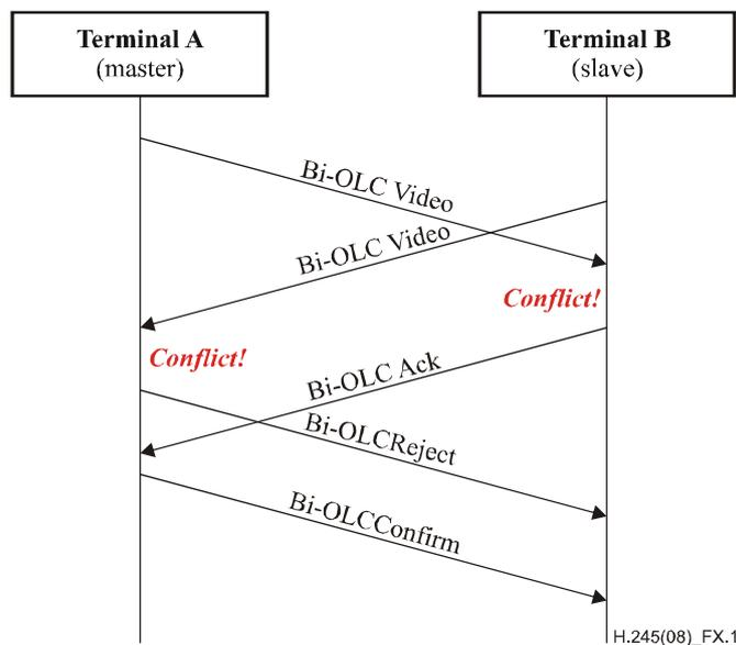
Figure X.1 – Both terminals use bidirectional OLC
