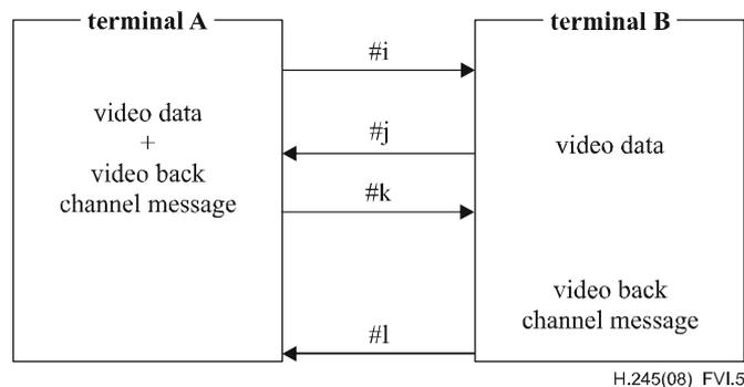
**Figure VI.5 – Coexistence of Separate Logical Channel mode with VideoMux mode**
