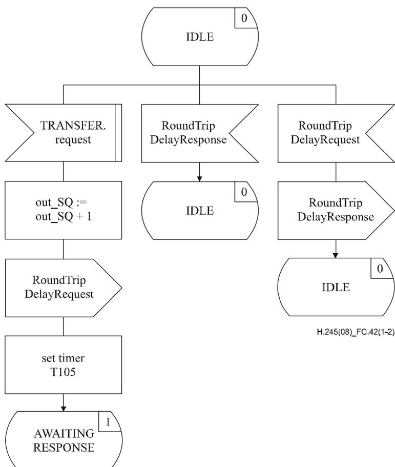
**Figure C.42 – RTDSE SDL (sheet 1 of 2)**
