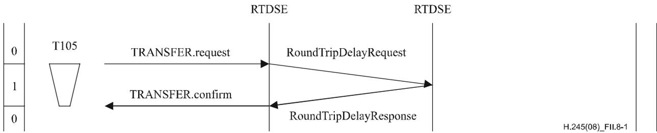
**Figure II.8-1 – Round-trip delay determination procedure**
