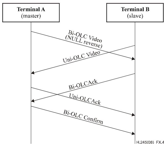
**Figure X.4 – Master proposes bidirectional OLC with nullData and slave proposes unidirectional OLC**
