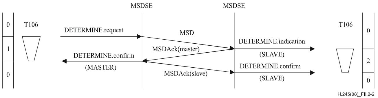
**Figure II.2-2 – Master-slave determination – Slave at remote MSDSE**
