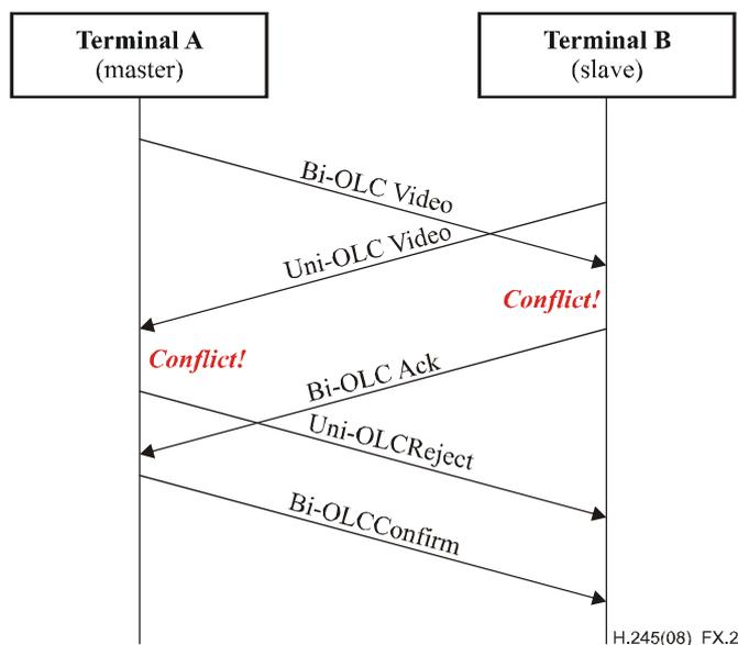
**Figure X.2 – Master proposes bidirectional OLC and slave proposes unidirectional OLC**
