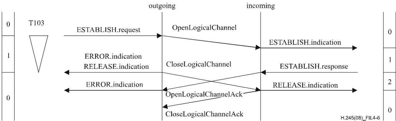
NOTE – Timer T103 has expired after transmission of the OpenLogicalChannelAck message at the incoming LCSE, but before reception of the OpenLogicalChannelAck message at the outgoing LCSE.
