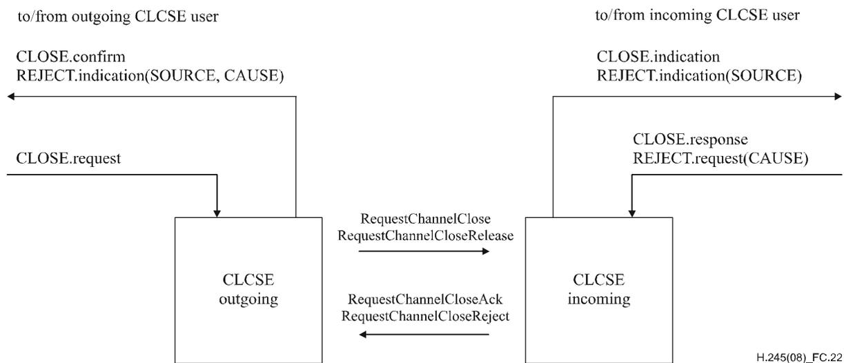
**Figure C.22 – Primitives and messages in the Close Logical Channel Signalling Entity**
