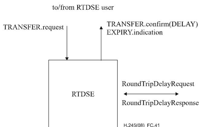
**Figure C.41 – Primitives and messages in the RTDSE**
