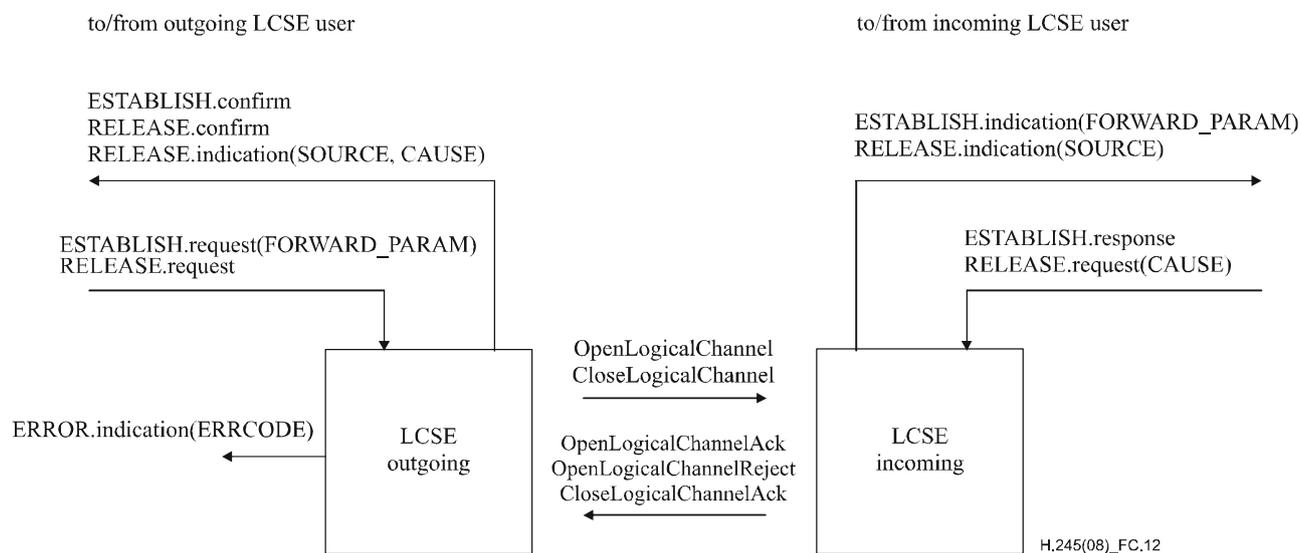
**Figure C.12 – Primitives and messages in the Logical Channel Signalling Entity**
