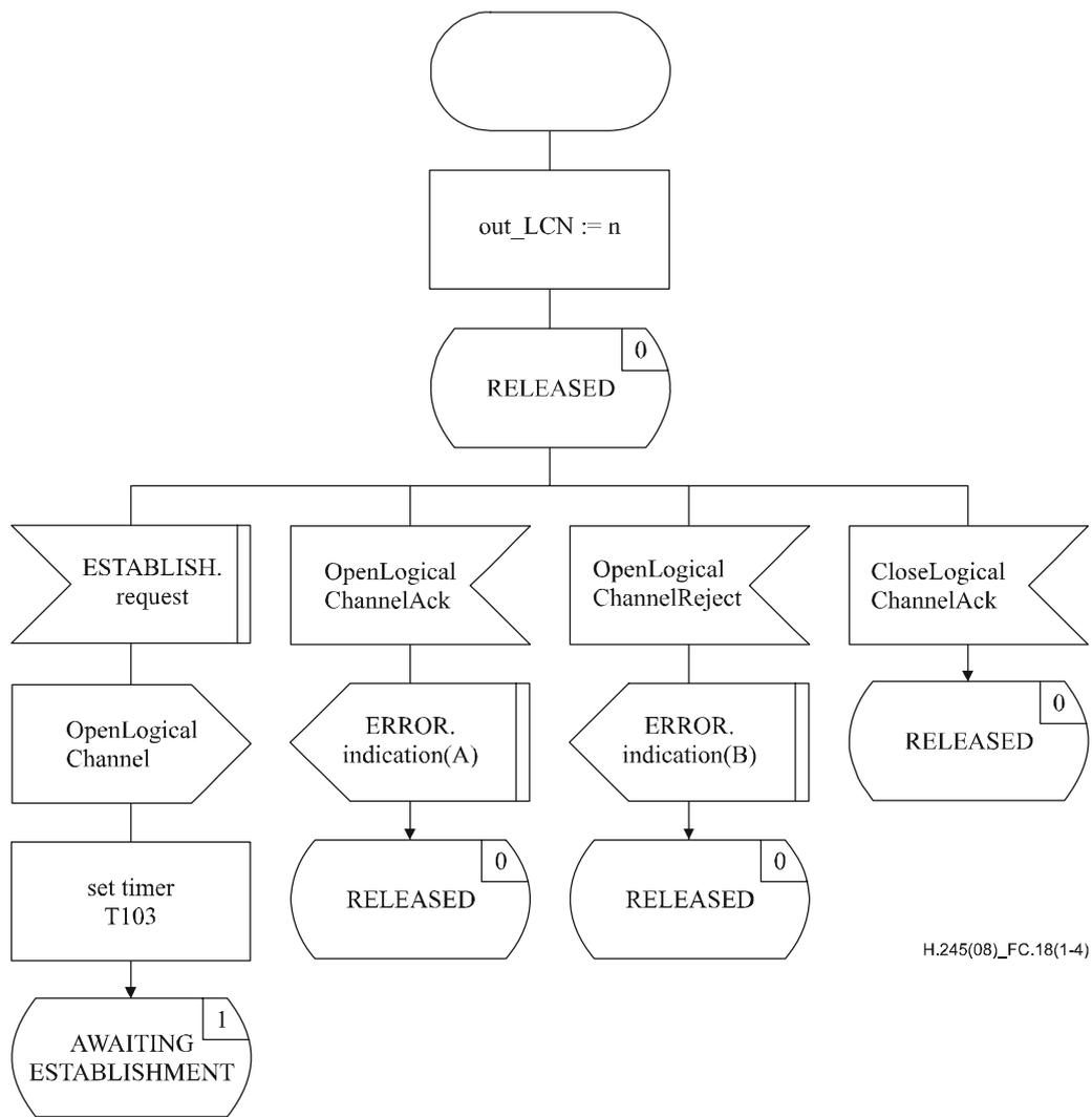
**Figure C.18 – Outgoing B-LCSE SDL (sheet 1 of 4)**
