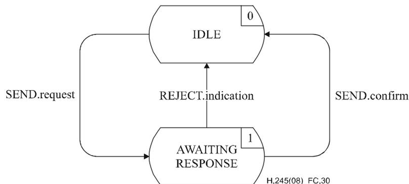
Figure C.30 – State transition diagram for sequence of primitives at outgoing RMESE
