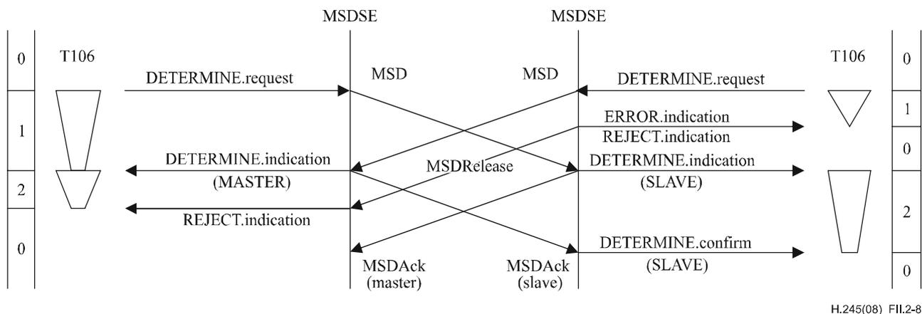
**Figure II.2-8 – Master-slave determination – Simultaneous determination procedures with timer T106 expiry at slave**
