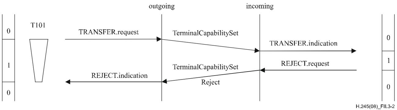
**Figure II.3-2 – Capability exchange with rejection from peer incoming CESE user**
