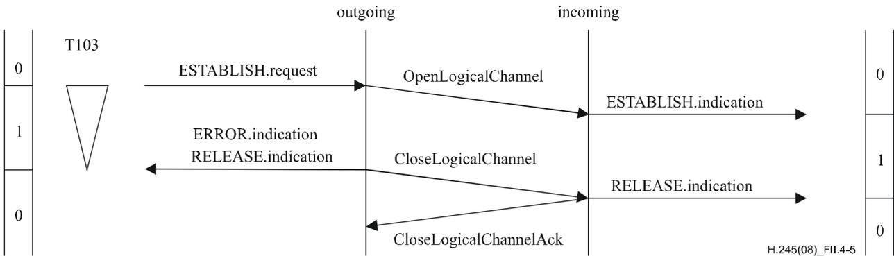
**Figure II.4-5 – Logical channel establishment request with expiry of timer T103 due to slow response from peer incoming LCSE user**
