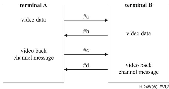
**Figure VI.2 – Logical Channels for Separate Logical Channel Mode**
