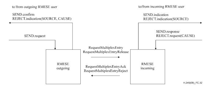
Figure C.32 – Primitives and messages in the Request Multiplex Entry Signalling Entity
