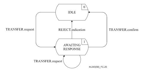
Figure C.25 – State transition diagram for sequence of primitives at outgoing MTSE
