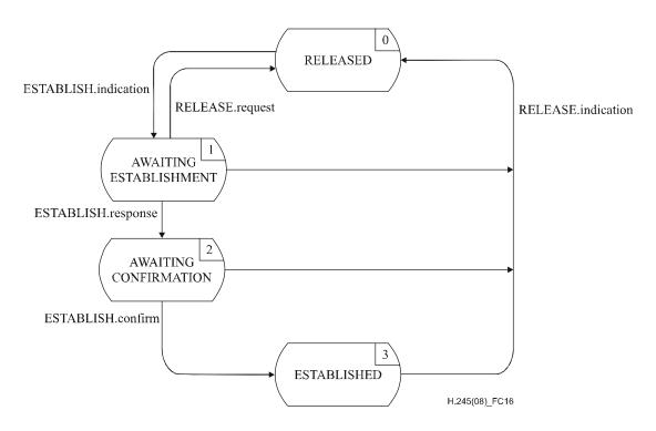
Figure C.16 – State transition diagram for sequence of primitives at incoming B-LCSE
