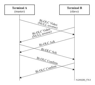
Figure X.5 – Both terminals propose bidirectional OLC with nullData
