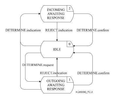
Figure C.2 – State transition diagram for sequence of primitives at MSDSE
