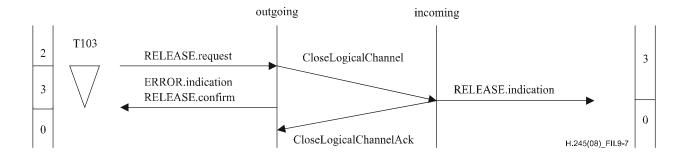
Figure II.9-7 – Bidirectional logical channel release request with expiry of timer T103 at the outgoing side
