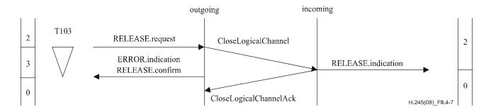
Figure II.4-7 – Logical channel release request with expiry of timer T103
