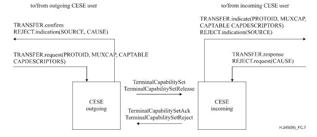
Figure C.7 – Primitives and messages in the Capability Exchange Signalling Entity
