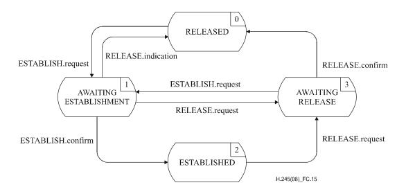
Figure C.15 – State transition diagram for sequence of primitives at outgoing B-LCSE
