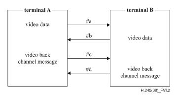
Figure VI.2 – Logical Channels for Separate Logical Channel Mode
