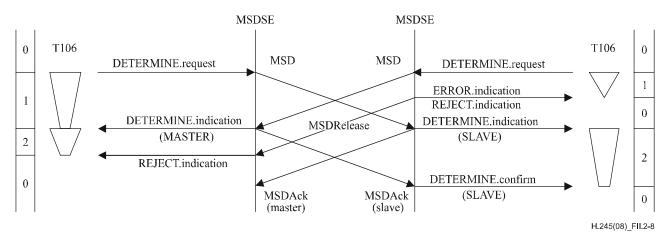
Figure II.2-8 – Master-slave determination – Simultaneous determination procedures with timer T106 expiry at slave
