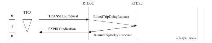
Figure II.8-3 – Round-trip delay determination procedure with timer T105 expiry
