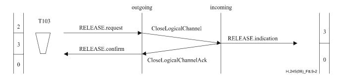
Figure II.9-2 – Bidirectional logical channel release
