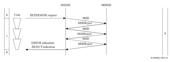
Figure II.2-10 – Master-slave determination – Indeterminate result with N100 = 3
