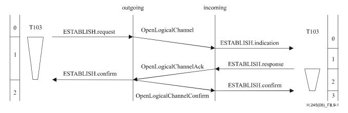
Figure II.9-1 – Bidirectional logical channel establishment
