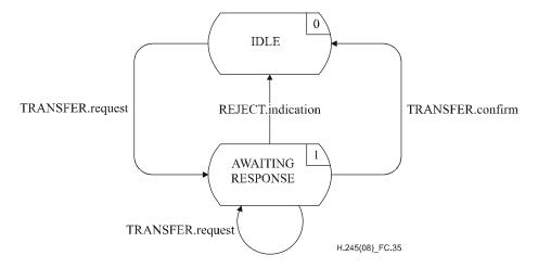
Figure C.35 – State transition diagram for sequence of primitives at outgoing MRSE
