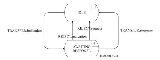
Figure C.36 – State transition diagram for sequence of primitives at incoming MRSE
