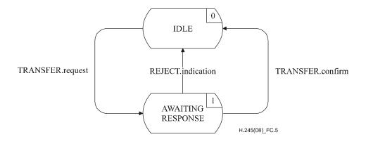
Figure C.5 – State transition diagram for sequence of primitives at outgoing CESE
