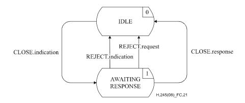
Figure C.21 – State transition diagram for sequence of primitives at incoming CLCSE
