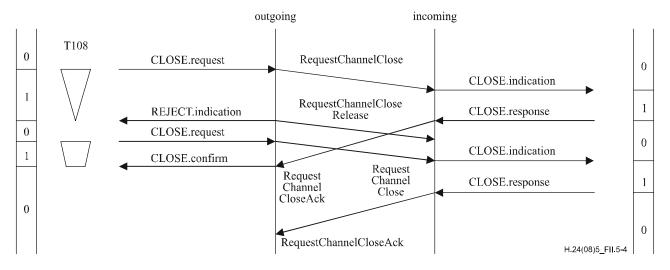
NOTE - The close channel request is confirmed on reception of the first RequestChannelClose message.
