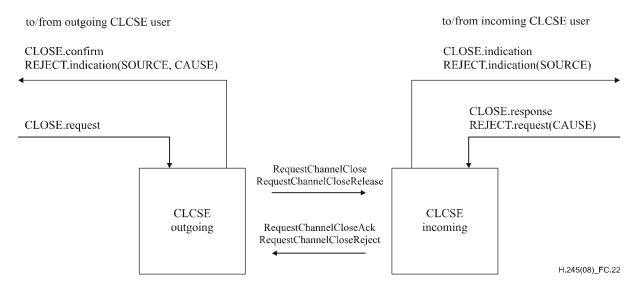
Figure C.22 – Primitives and messages in the Close Logical Channel Signalling Entity
