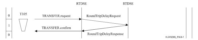
Figure II.8-1 – Round-trip delay determination procedure
