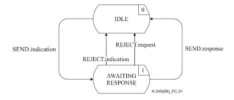
Figure C.31 – State transition diagram for sequence of primitives at incoming RMESE
