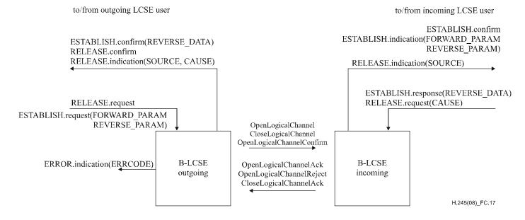
Figure C.17 – Primitives and messages in the bidirectional Logical Channel Signalling Entity
