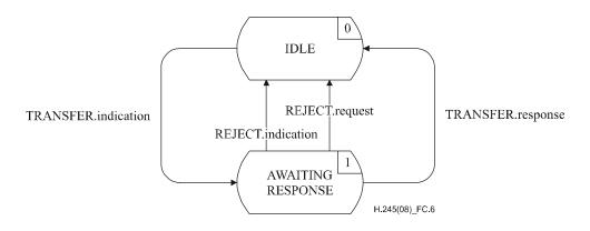
Figure C.6 – State transition diagram for sequence of primitives at incoming CESE
