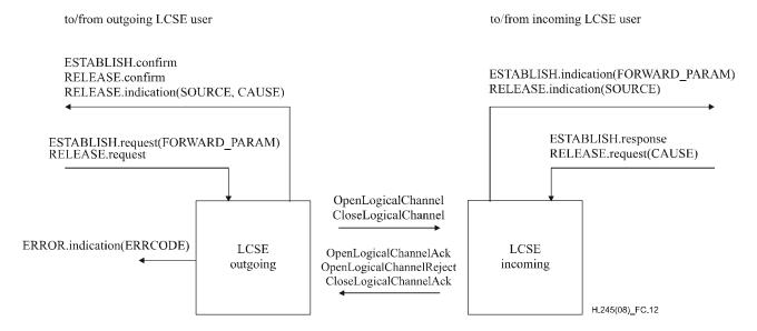
Figure C.12 – Primitives and messages in the Logical Channel Signalling Entity
