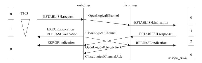
NOTE – Timer T103 has expired after transmission of the OpenLogicalChannelAck message at the incoming LCSE, but before reception of the OpenLogicalChannelAck message at the outgoing LCSE.
