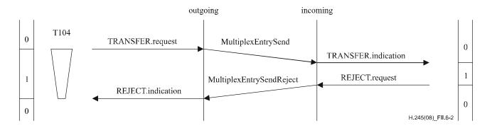
Figure II.6-2 – Multiplex table send request with rejection from the peer MTSE user
