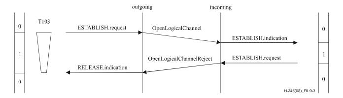
Figure II.9-3 – Bidirectional logical channelestablishment rejection by peer B-LCSE user
