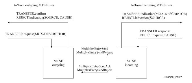
Figure C.27 – Primitives and messages in the Multiplex Table Signalling Entity
