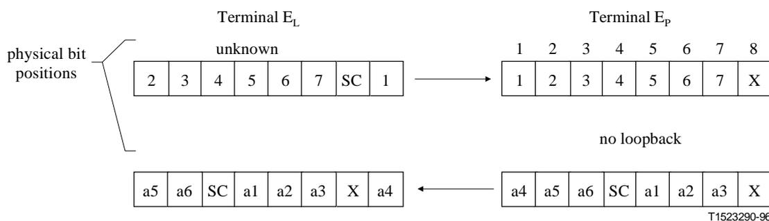
In this case, the first step change must be to move the SC itself and stuff the outgoing bit which will be lost. Then the same loopback procedure is used to identify which of the incoming bits is to be discarded.
