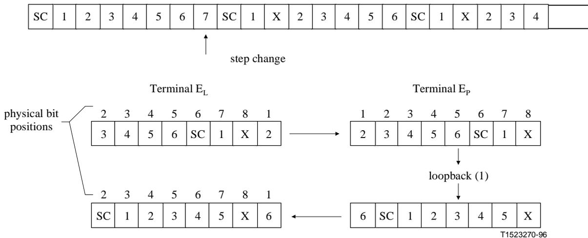
It is now the Bit 8 which is lost.  $E_L$  now sends Loop-off, audio on, and repetitive capability sets, entering mode initialization procedure of 9.1. On the receive side, the signal from  $E_P$  probably has the SC in a different position, since its framer does not see the network timing, but physical Bit 8 continues to be stuffed, and so  $E_L$  discards this; a1-a6 denote PCM audio bits.
