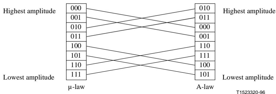
**Figure X.1/H.242 – Order of segments according to amplitude,  $\mu$ -law and A-law PCM**
