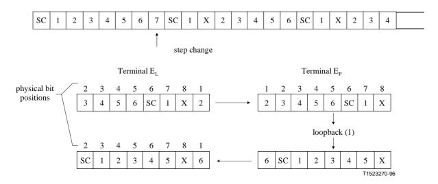
It is now the Bit 8 which is lost.  $E_L$  now sends Loop-off, audio on, and repetitive capability sets, entering mode initialization procedure of 9.1. On the receive side, the signal from  $E_P$  probably has the SC in a different position, since its framer does not see the network timing, but physical Bit 8 continues to be stuffed, and so  $E_L$  discards this; a1-a6 denote PCM audio bits.
