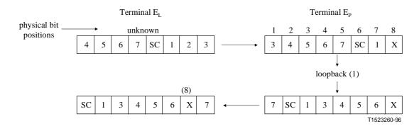
The digital loopback (1) returns the same bits as received at  $E_P$ , with no particular relationship to the network timing, but of course the stuffing bit is correctly positioned.
