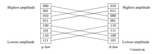
Figure X.1/H.242 – Order of segments according to amplitude, μ-law and A-law PCM
