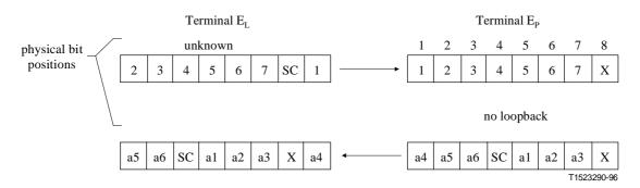
In this case, the first step change must be to move the SC itself and stuff the outgoing bit which will be lost. Then the same loopback procedure is used to identify which of the incoming bits is to be discarded.
