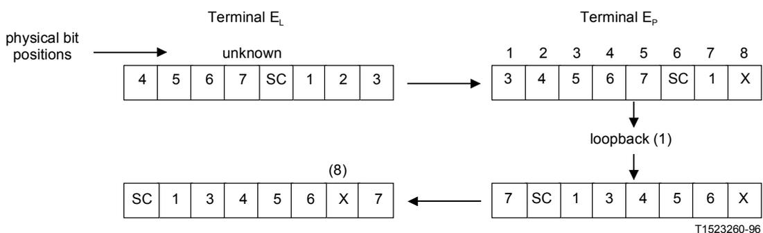
The digital loopback (1) returns the same Bits as received at E<sub>P</sub>, with no particular relationship to the network timing, but of course the stuffing bit is correctly positioned.
