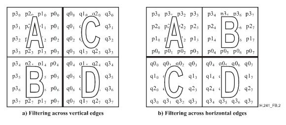
Figure B.2 – Arrangement of 8 × 8 blocks when filtering across vertical or horizontal edges
