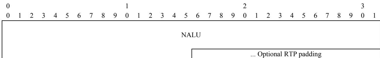
**Figure A.2/H.241 – RTP payload format for simple packet**
