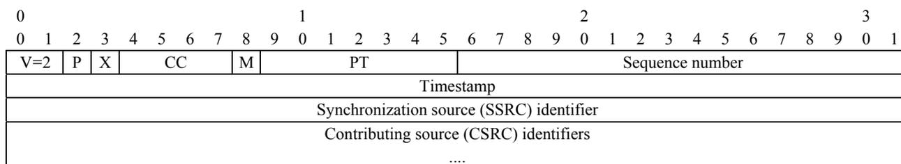
**Figure A.1/H.241 – RTP header according to RFC 3550**
