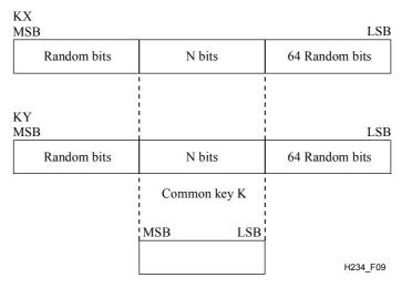
NOTE - N-bit blocks from KX and KY are modulo 2 added to form common key K
