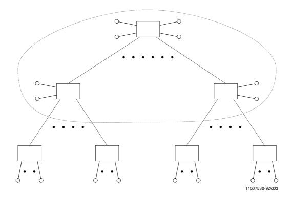
FIGURE 3/H.231 MCU hierarchical configuration
