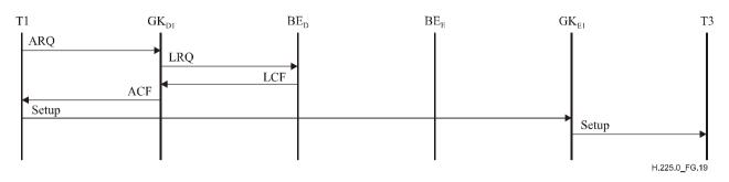
Figure G.19 – Example of GK routed call using cached descriptor
