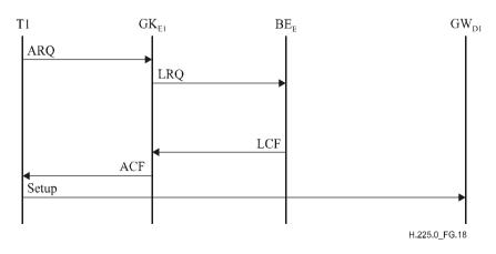
Figure G.18 – Example of call using cached descriptor in local BE
