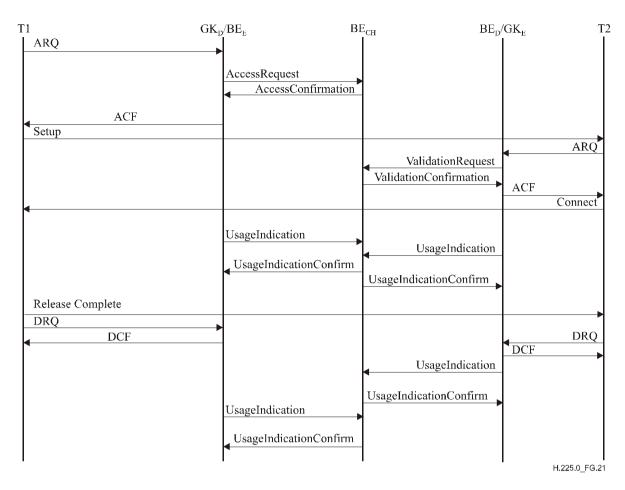
Figure G.21 – Call validation and usage reporting example with clearing house
