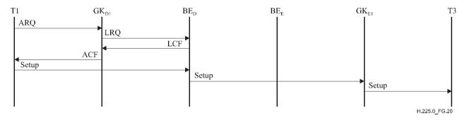
Figure G.20 – Example of call with combined BE/routing GK
