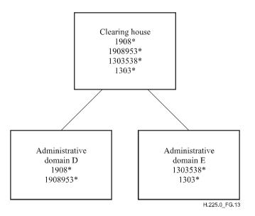
Figure G.13 – Sample clearing house configuration
