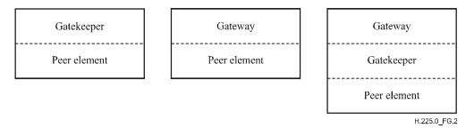
Figure G.2 – Peer element placement examples
