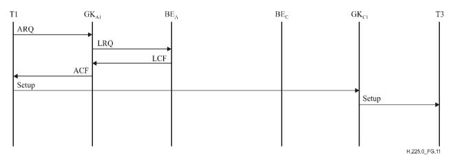
Figure G.11 – Example of remote gatekeeper routed call
