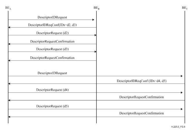
Figure G.8 – Example of descriptor exchange
