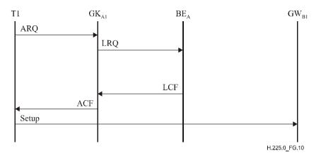
**Figure G.10 – Example of a call with cached address**
