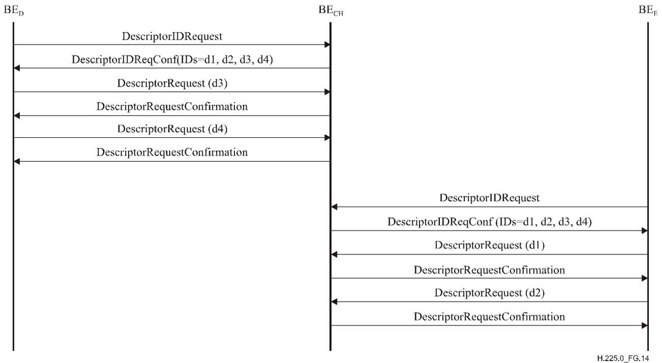
**Figure G.14 – Example descriptor exchange with clearing house**
