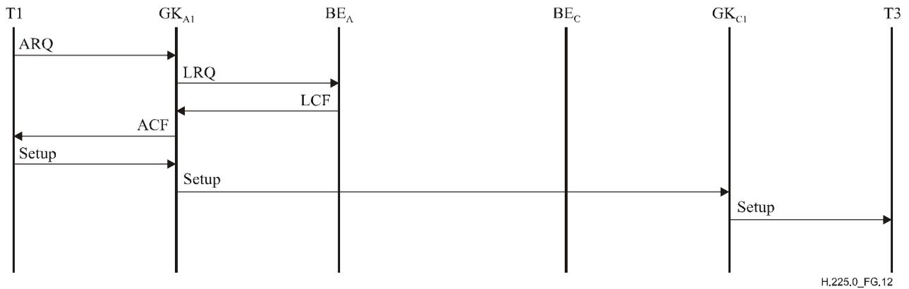
**Figure G.12 – Example of local gatekeeper routed call**
