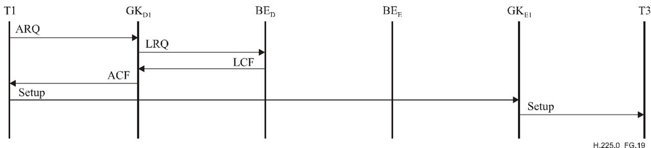
**Figure G.19 – Example of GK routed call using cached descriptor**
