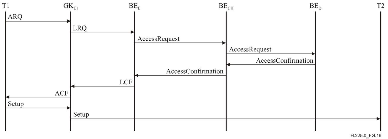
**Figure G.16 – Example of local gatekeeper routed call with clearing house**
