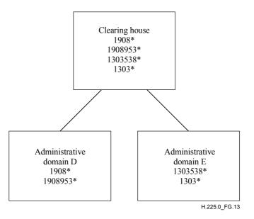
Figure G.13/H.225.0 – Sample clearing house configuration
