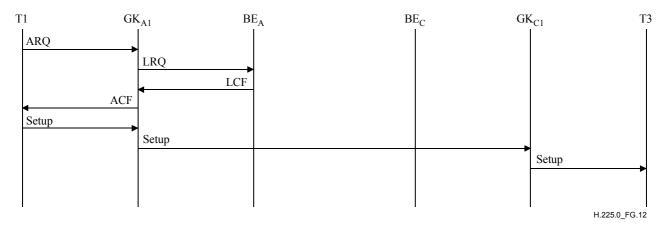
Figure G.12/H.225.0 – Example of local gatekeeper routed call
