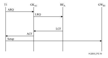
Figure G.10/H.225.0 – Example of a call with cached address
