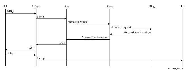
Alternatively, T1's gatekeeper could route the call signalling, as shown in Figure G.16.
