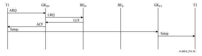
Figure G.19/H.225.0 – Example of GK routed call using cached descriptor
