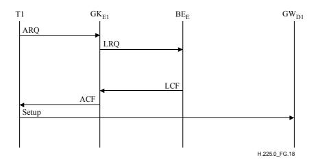
Figure G.18/H.225.0 – Example of call using cached descriptor in local BE
