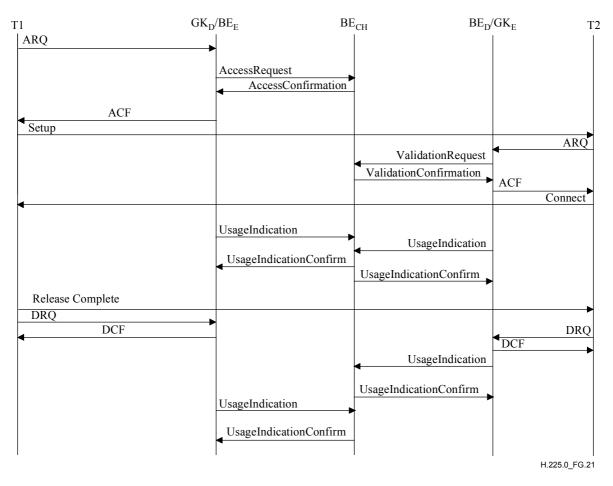
Figure G.21/H.225.0 – Call validation and usage reporting example with clearing house
