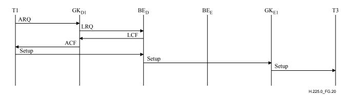
Figure G.20/H.225.0 – Example of call with combined BE/routing GK
