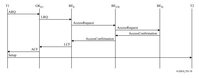
Figure G.15/H.225.0 – Example of call with clearing house
