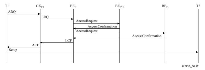
Figure G.17/H.225.0 – Example of clearing house routing using contact info for remote BE
