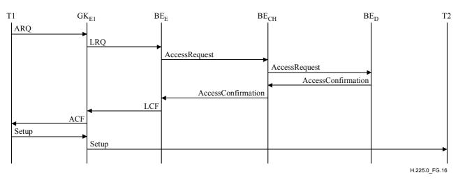
Alternatively, T1's gatekeeper could route the call signalling, as shown in Figure G.16.
