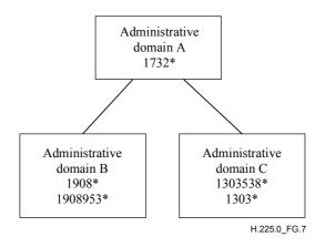
Figure G.7/H.225.0 – Distributed network for signalling examples
