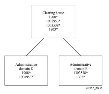
Figure G.13/H.225.0 – Sample clearing house configuration
