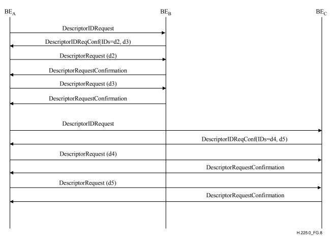
Figure G.8/H.225.0 – Example of descriptor exchange
