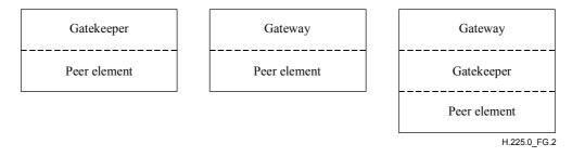
Figure G.2/H.225.0 – Peer element placement examples
