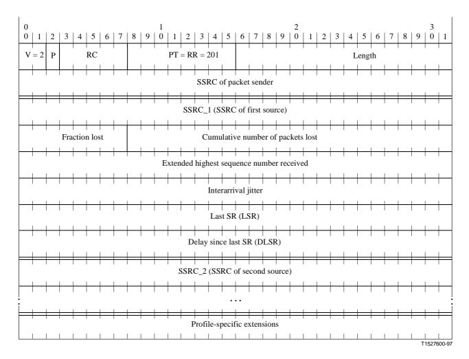
The format of the Receiver Report (RR) packet is the same as that of the SR packet except that the packet type field contains the constant 201 and the five words of sender information are omitted (these are the NTP and RTP timestamps and sender's packet and octet counts). The remaining fields have the same meaning as for the SR packet.
