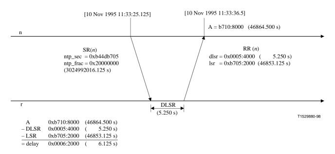
Figure A.2/H.225.0 – Example for round-trip time computation
