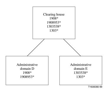
Figure G.13/H.225.0 – Sample Clearing House Configuration
