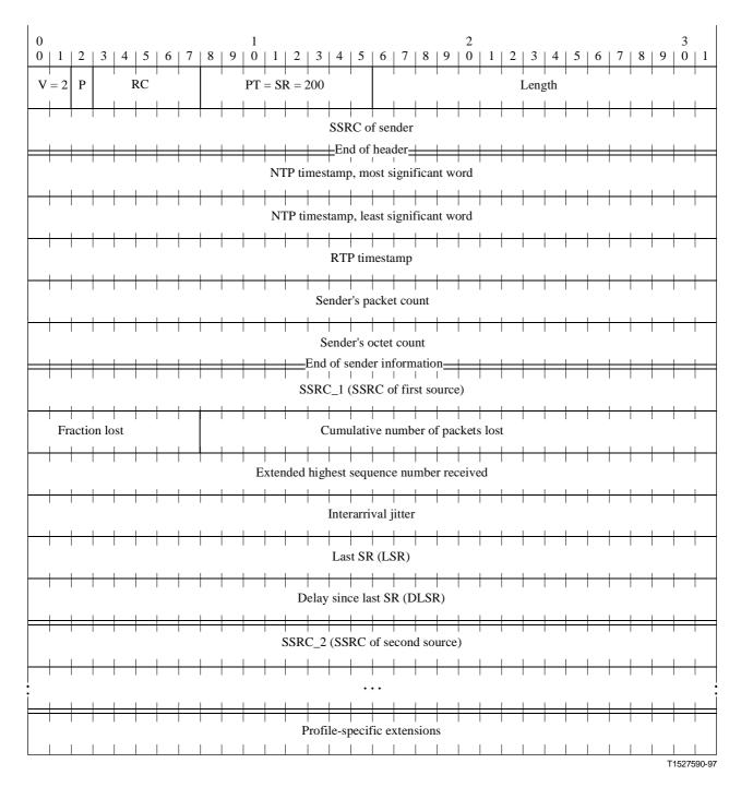
The sender report packet consists of three sections, possibly followed by a fourth profile-specific extension section if defined. The first section, the header, is 8 octets long. The fields have the following meaning:
