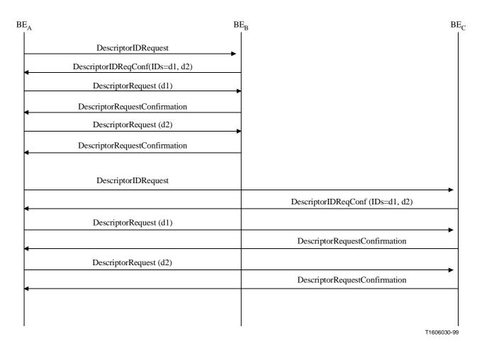
Figure G.8/H.225.0 – Example of Descriptor Exchange
