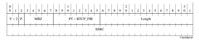
This packet indicates that a receiver requires a full encoded image in order to either start decoding with an entire image or to refresh its image and speed the recovery after a burst of lost packets. The receiver requests the source to force the next image in full "INTRA-frame" coding mode, i.e. without using differential coding. The various fields are defined in the RTP specification (Annex A). SSRC
