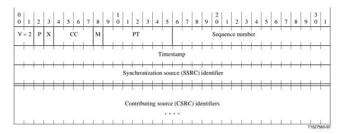
The first twelve octets are present in every RTP packet, while the list of CSRC identifiers is present only when inserted by a mixer. The fields have the following meaning:
