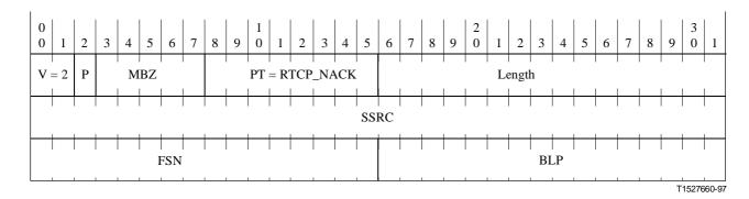
The various fields T, P, PT, length and SSRC are defined in the RTP specification (see Annex A). The value of the Packet Type (PT) identifier is the constant RTCP\_NACK (193). SSRC is the synchronization source identifier for the sender of this packet.
