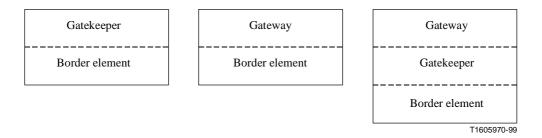
Figure G.2/H.225.0 – Border Element Placement Examples
