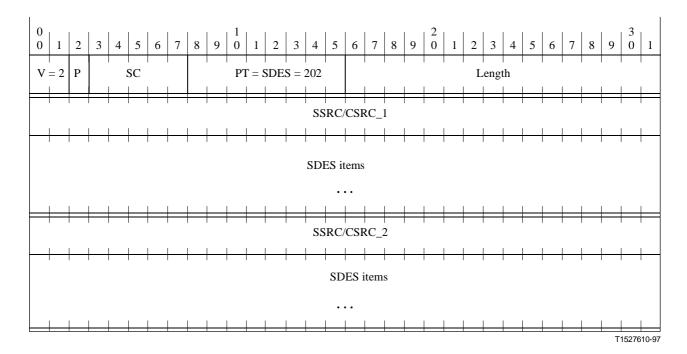
The SDES packet is a three-level structure composed of a header and zero or more chunks, each of which is composed of items describing the source identified in that chunk. The items are described individually in subsequent subclauses.
