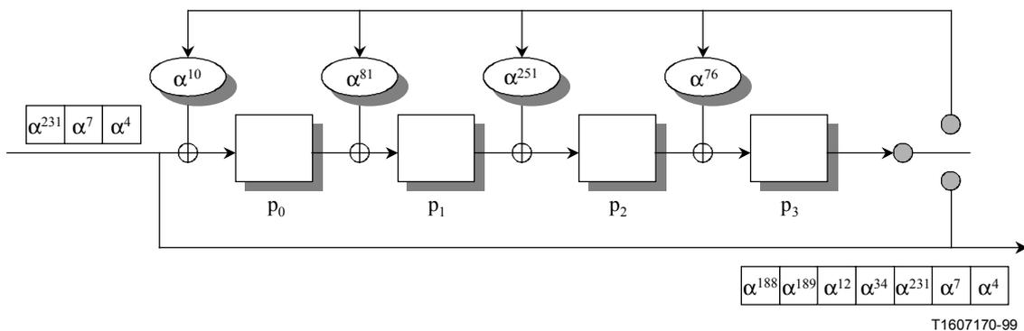
**Figure D.4/H.223 – Example of Reed-Solomon encoder ( $e_{target} = 2$ )**
