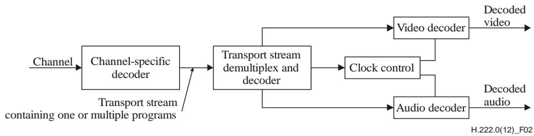
**Figure Intro. 2 – Prototypical transport demultiplexing and decoding example**
