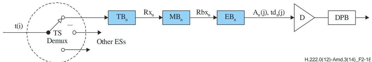
Figure 2-18 – T-STD model extensions for single layer HEVC
