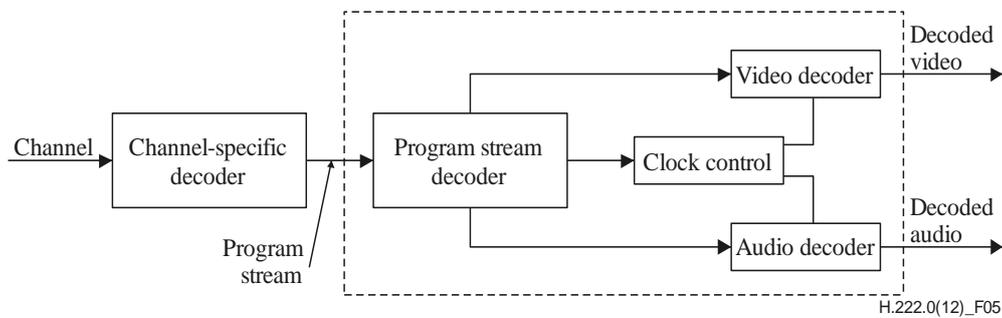
**Figure Intro. 5 – Prototypical decoder for program streams**
