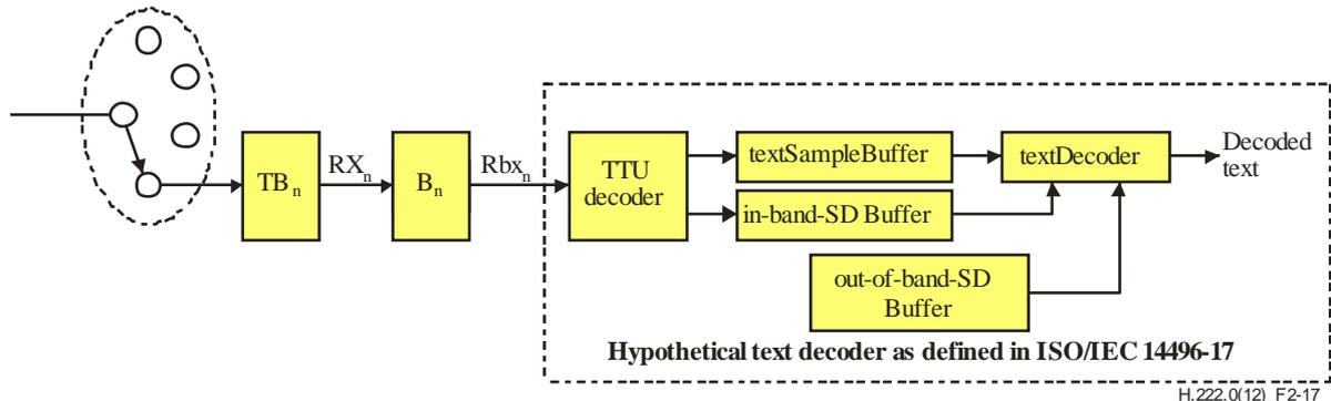
Figure 2-17 – T-STD model extensions for ISO/IEC 14496-17 text streams
