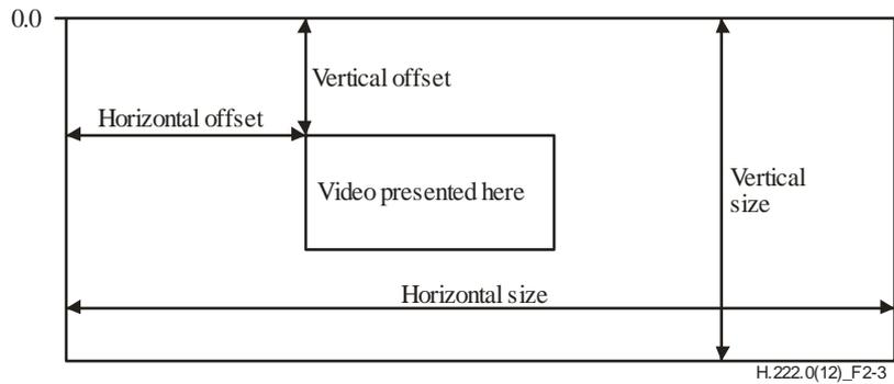
Figure 2-3 – Target background grid descriptor display area
