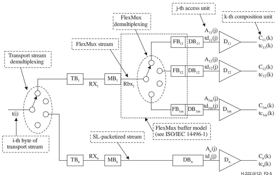
**Figure 2-5 – T-STD model for ISO/IEC 14496 content**
