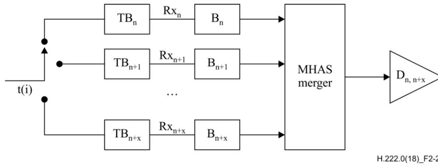
**Figure 2-25 – Transport stream system target decoder for multiple audio elementary streams**
