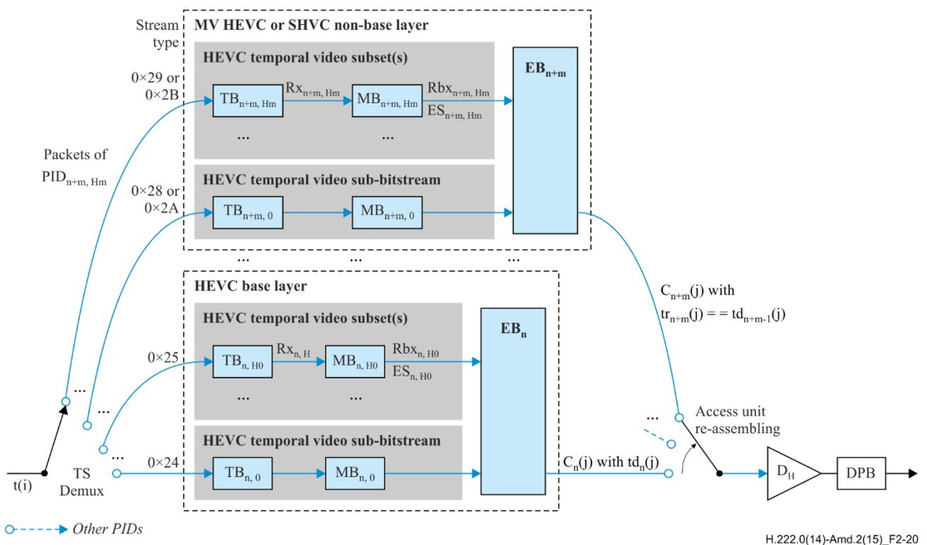
**Figure 2-20 – T-STD model extensions for bitstream-partition-specific CPB operation**
