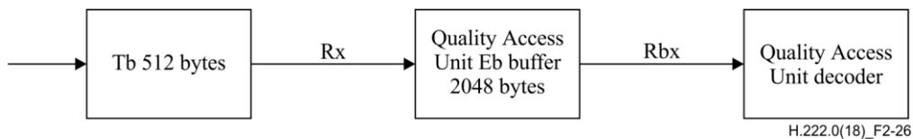
**Figure 2-26 – Quality Access Unit decoder processing model**
