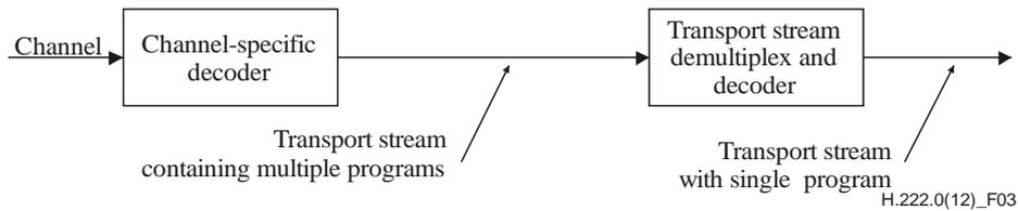
**Figure Intro. 3 – Prototypical transport multiplexing example**
