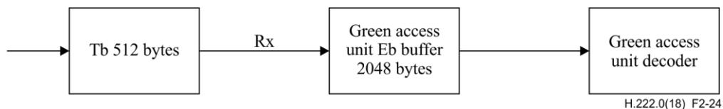
Figure 2-24 – T-STD model extension for green access units
