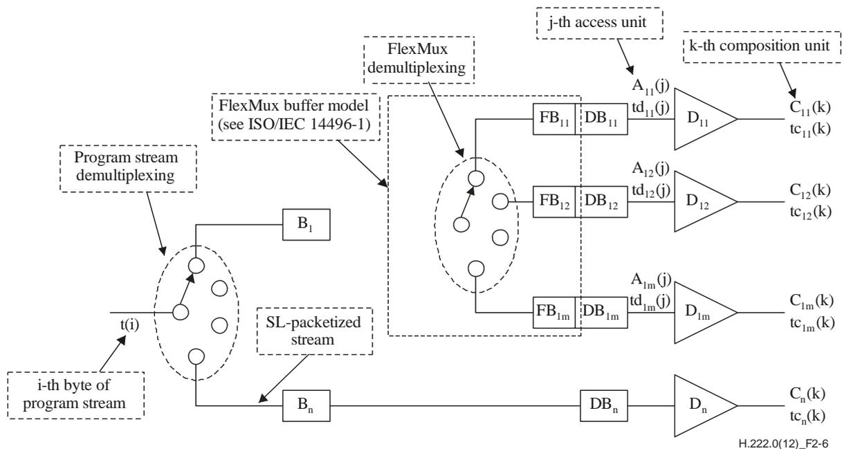
**Figure 2-6 – P-STD model for ISO/IEC 14496 Systems stream**
