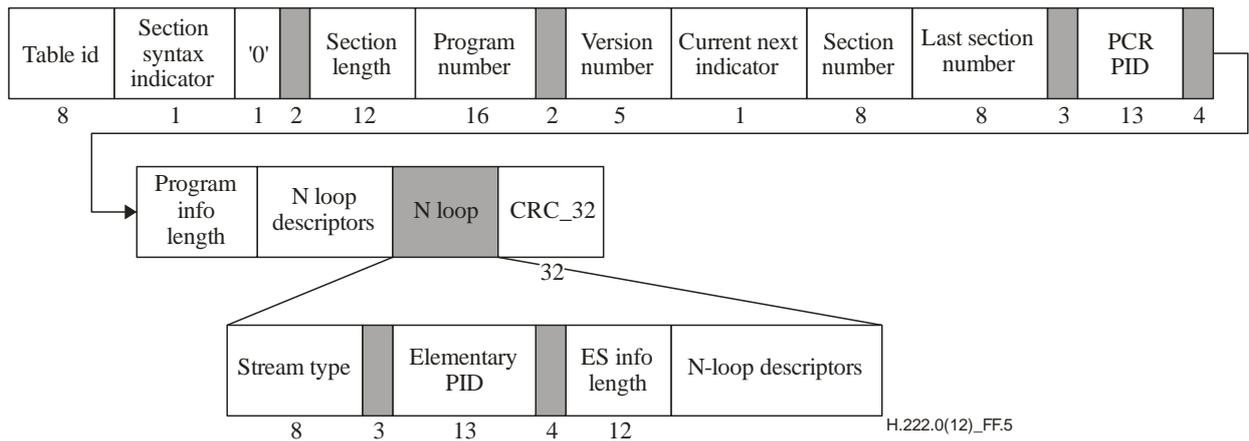
**Figure F.5 – TS program map section diagram**
