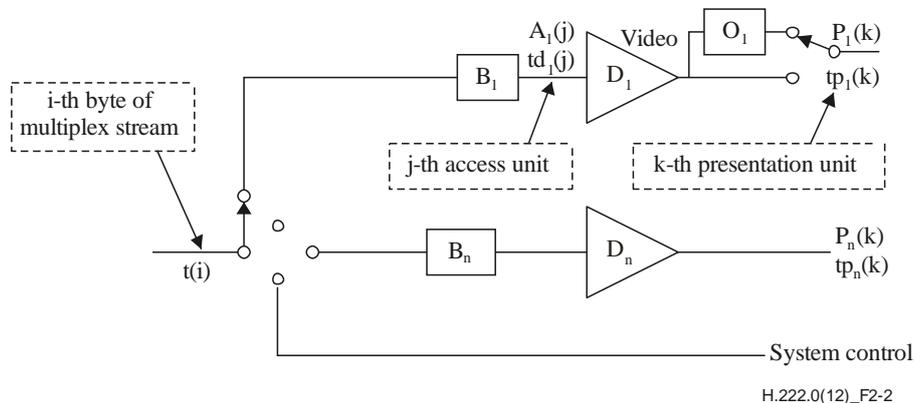
Figure 2-2 – Program stream system target decoder notation
