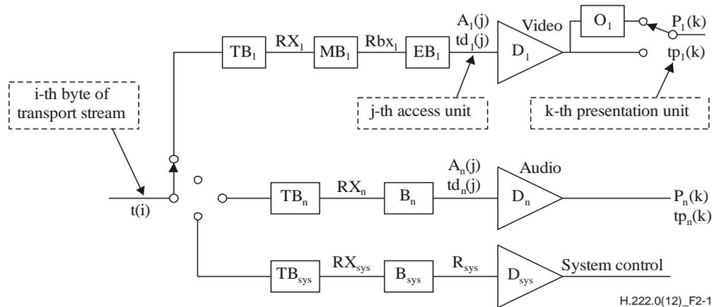
**Figure 2-1 – Transport stream system target decoder notation**
