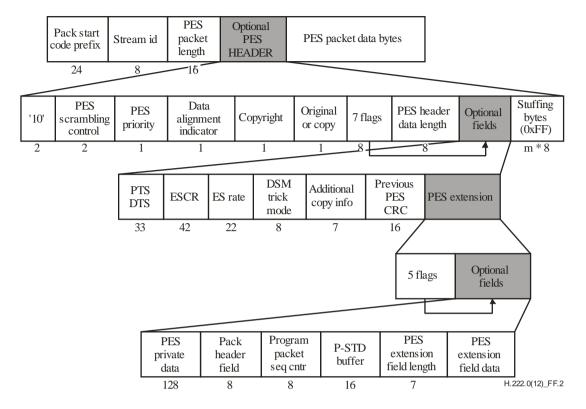
Figure F.2 – PES packet syntax diagram
