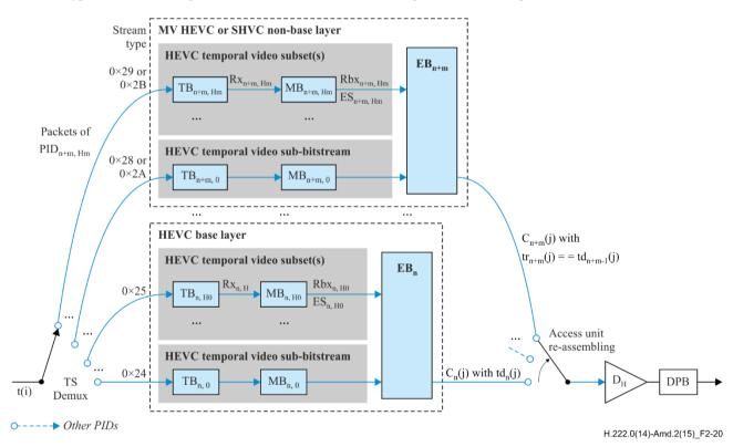
Figure 2-20 – T-STD model extensions for bitstream-partition-specific CPB operation
