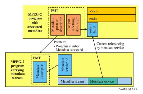
Figure 2-9 – Metadata signalling and referencing
