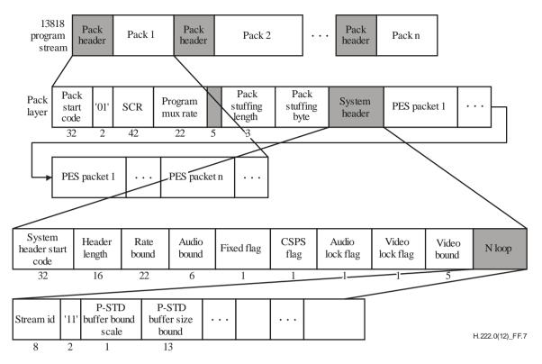
Figure F.7 – Program stream diagram
