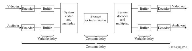
Figure D.1 - Constant delay model
