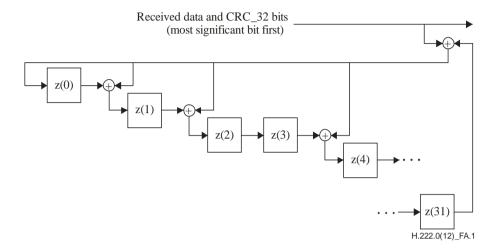
Figure A.1 – 32-bit CRC decoder model
