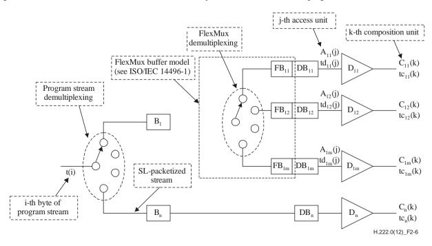
Figure 2-6 – P-STD model for ISO/IEC 14496 Systems stream
