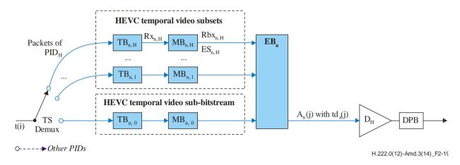
Figure 2-19 - T-STD model extensions for layered transport of HEVC temporal video subsets
