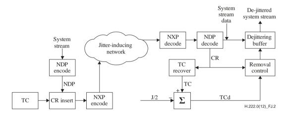
Figure J.2 – Jitter-smoothing using network-layer timestamps
