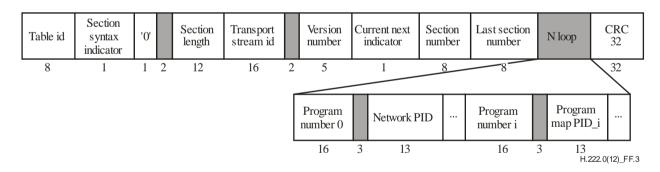
Figure F.3 – Program association section diagram
