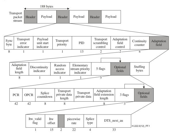
Figure F.1 – Transport stream syntax diagram
