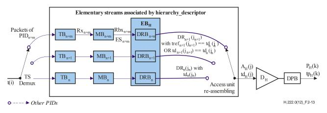
Figure 2-13 – T-STD model extensions for Rec. ITU-T H.264 | ISO/IEC 14496-10 Video with scalable video sub-bitstreams
