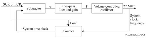
Figure D.2 – STC recovery using PLL
