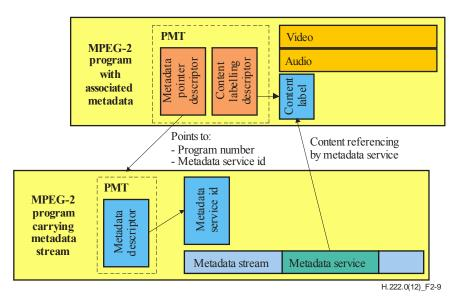
Figure 2-9 – Metadata signalling and referencing
