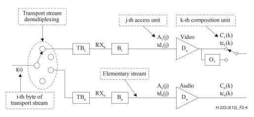
Figure 2-4 – T-STD model extensions for individual ISO/IEC 14496 elementary streams
