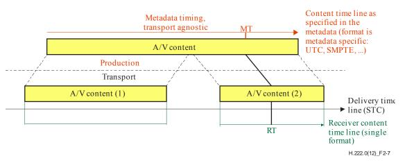
Figure 2-7 – Timing model for delivery of content and metadata
