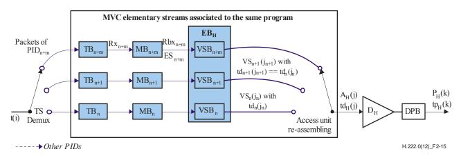
Figure 2-15 – T-STD model extensions for Rec. ITU-T H.264 | ISO/IEC 14496-10 Video with MVC video sub-bitstreams
