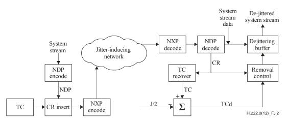
Figure J.2 – Jitter-smoothing using network-layer timestamps
