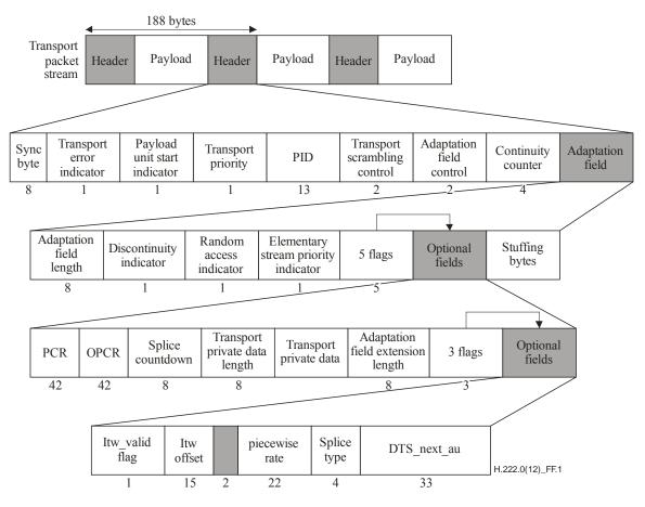
Figure F.1 – Transport stream syntax diagram
