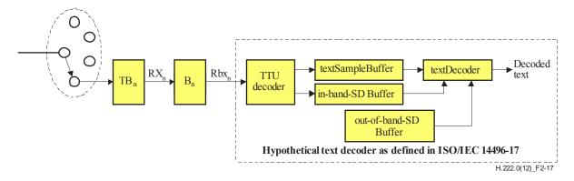
Figure 2-17 – T-STD model extensions for ISO/IEC 14496-17 text streams
