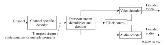
Figure Intro. 2 – Prototypical transport demultiplexing and decoding example
