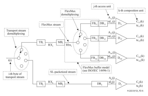
Figure 2-5 – T-STD model for ISO/IEC 14496 content
