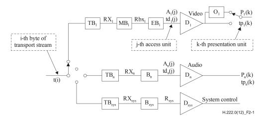
Figure 2-1 – Transport Stream system target decoder notation
