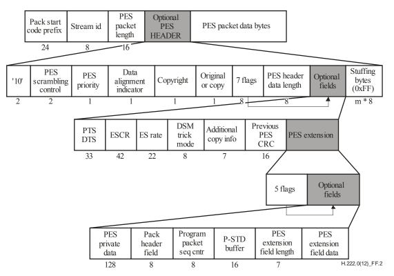
Figure F.2 – PES packet syntax diagram
