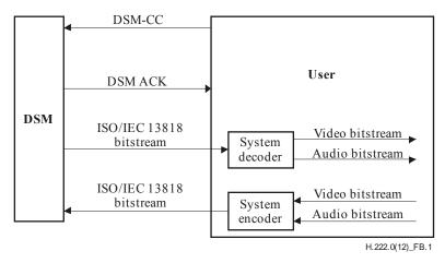
Figure B.1 – Configuration of DSM-CC application
