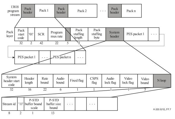
Figure F.7 – Program stream diagram
