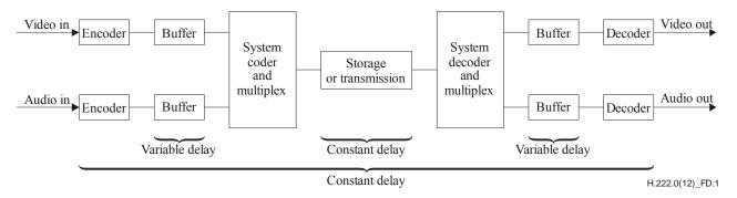
Figure D.1 – Constant delay model
