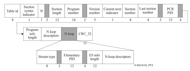
Figure F.5 – TS program map section diagram
