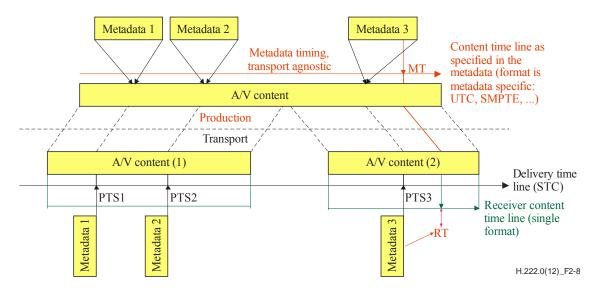
Figure 2-8 – Delivery of metadata in PES packets
