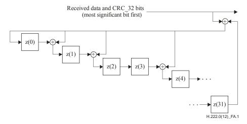
Figure A.1 – 32-bit CRC decoder model
