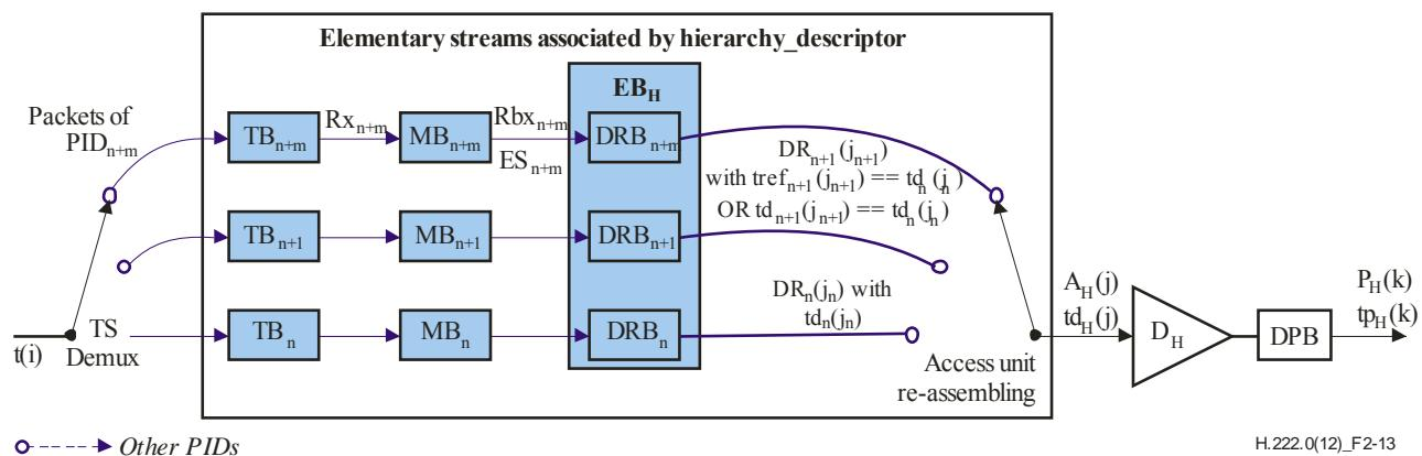
Figure 2-13 – T-STD model extensions for Rec. ITU-T H.264 | ISO/IEC 14496-10
