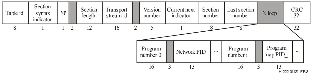
Figure F.3 – Program Association section diagram
