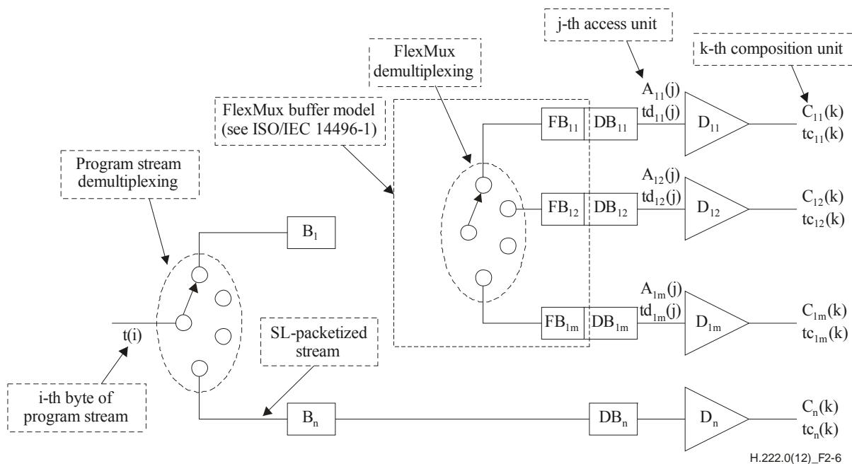
**Figure 2-6 – P-STD model for ISO/IEC 14496 Systems stream**
