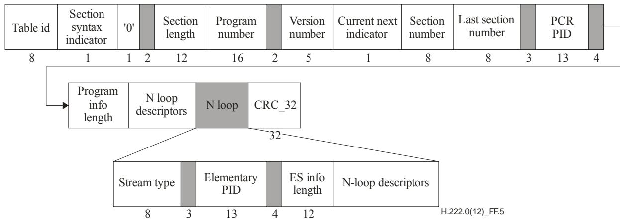
**Figure F.5 – TS program map section diagram****F.1.6 Private section**
