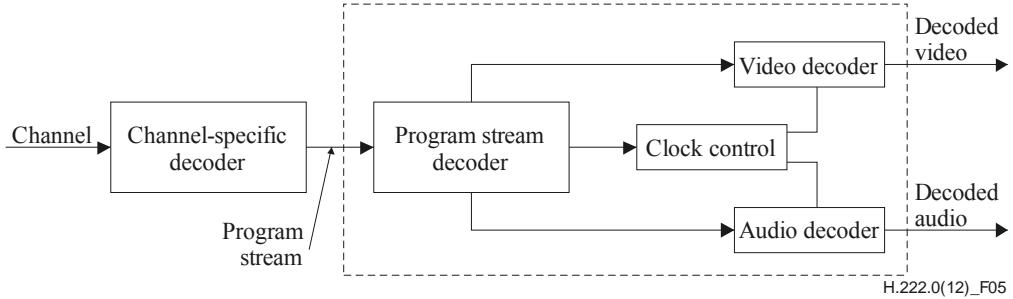
**Figure Intro. 5 – Prototypical decoder for program streams**
