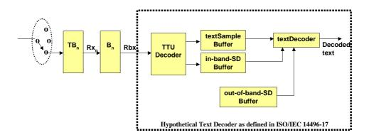
Figure 2-13 – T-STD model extensions for ISO/IEC 14496-17 text streams
