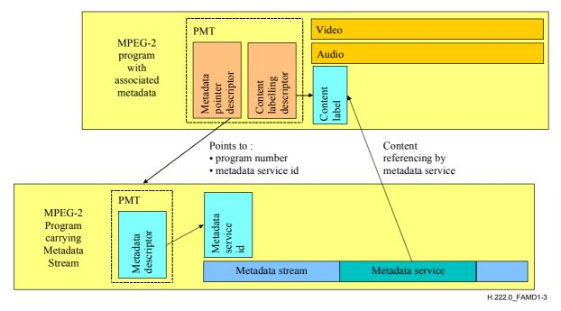
Figure Amd.1-3 – Metadata signalling and referencing
