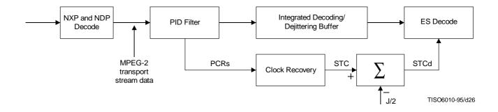
Figure J.3 - Integrated dejittering and MPEG-2 decoding
