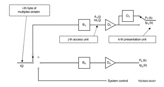
Figure 2-2 - Program Stream system target decoder notation
