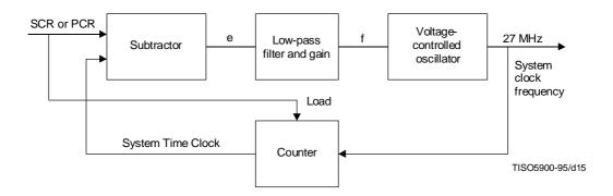
Figure D.2 – STC recovery using PLL
