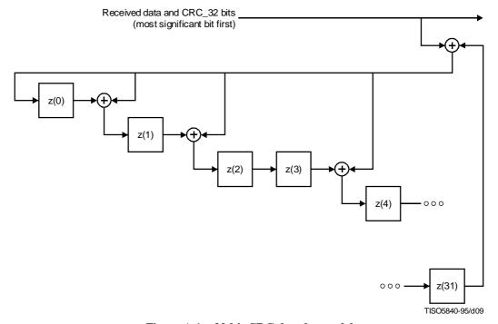
Figure A.1 – 32-bit CRC decoder model
