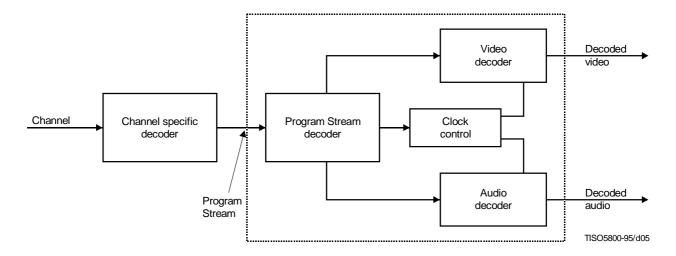
Figure Intro. 5 – Prototypical decoder for Program Streams
