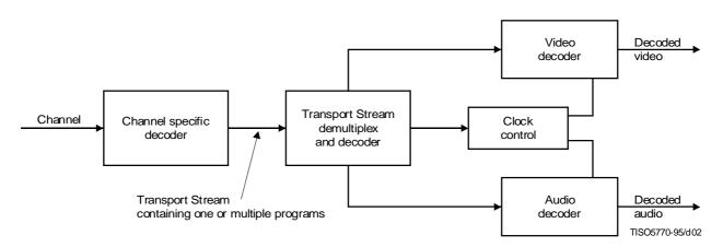
Figure Intro. 2 – Prototypical transport demultiplexing and decoding example
