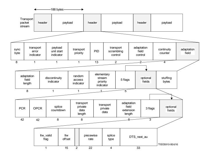
Figure F.1 – Transport Stream syntax diagram
