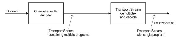
Figure Intro. 3 – Prototypical transport multiplexing example
