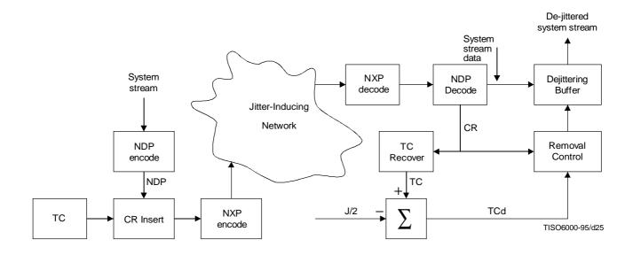
Figure J.2 – Jitter-smoothing using network-layer timestamps
