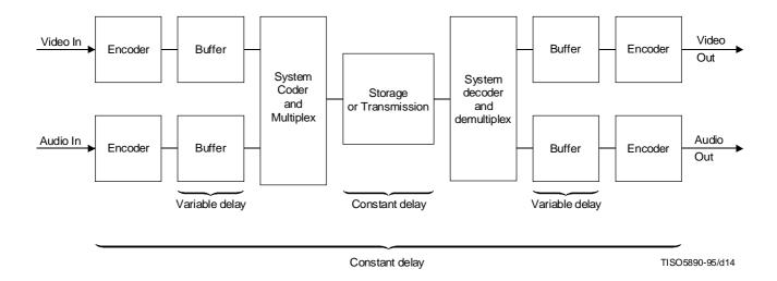
Figure D.1 - Constant delay model
