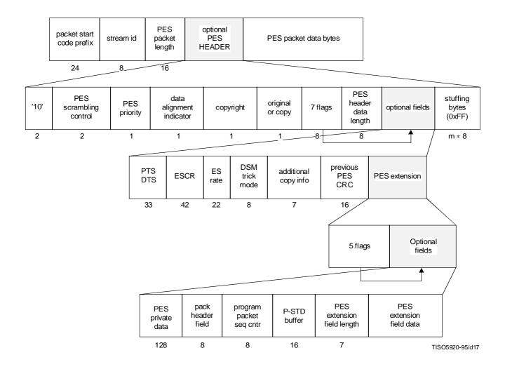
Figure F.2 – PES packet syntax diagram
