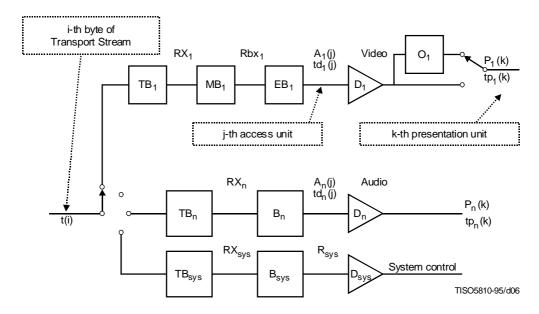
Figure 2-1 - Transport Stream system target decoder notation
