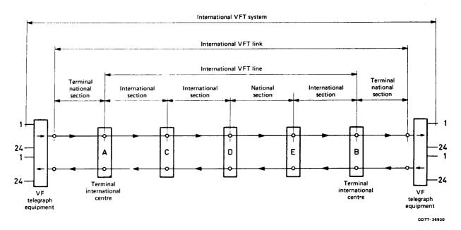
(At the intermediate centres C, D and E and at the terminal international centres A and B, the signals transmitted are at audio frequencies. At these points it is possible to make measurements.)
